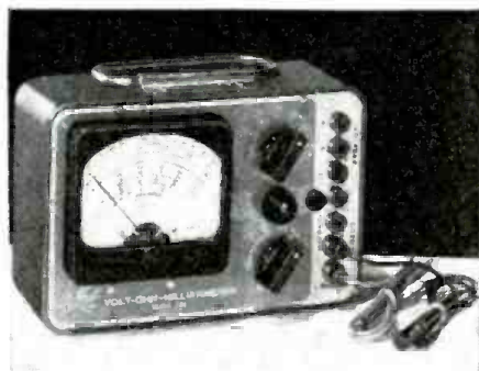
The Hickok Model 435 measures a. c. at 5,000 ohms per volt.
