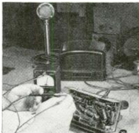
Be sure set is off when measuring resistance.
