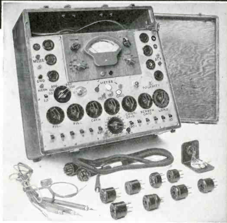
Fig. 1—Front of the complete tester and set analyzer. Standard analyzer adapters are used. A special adapter tests acorn tubes.
