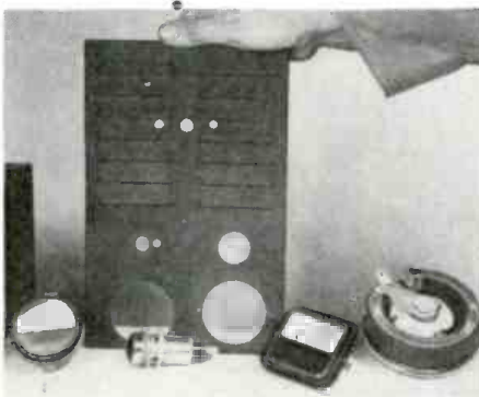
Photo 3—Drill holes in panel for new parts.
