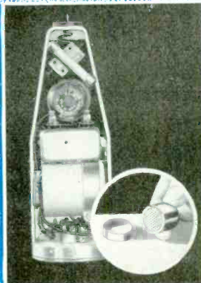
The amplifier is contained within the case of Western Electric's 640AA condenser miko. Mike (inset), screws on end.
