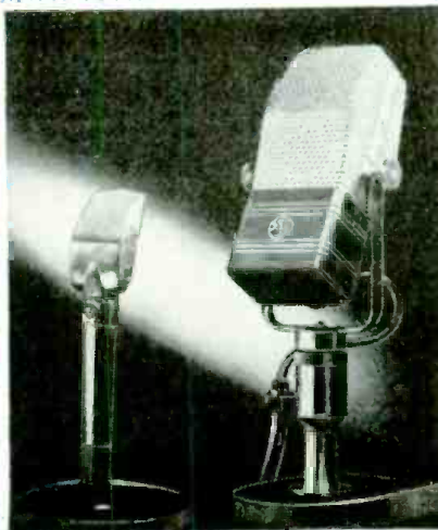
The Stephens C-1 is a new condenser microphone that phase-modulates a crystal oscillator. Response extends from one-half cycle in 24 hours upward to 15 kc.
