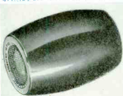
The Stephens C-1 is a new condenser microphone that phase-modulates a crystal oscillator. Response extends from one-half cycle in 24 hours upward to 15 kc.
