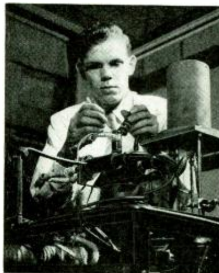
Loading sample chamber of mass spectrometer in preparation for an analysis of metal vapor.
