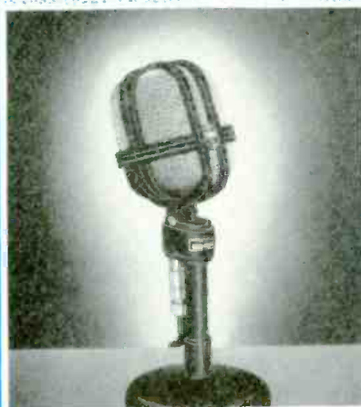
This cardioid, Turner Model 77, has a front-to-rear discrimination of 15 db.
