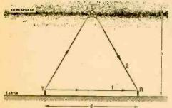
Fig. 7—How height of ionosphere is checked.
