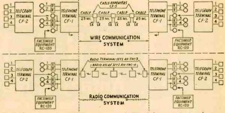
Fig. 2—Comparison, wire and VHF communication facilities, U.S. Army multi-channel systems.
