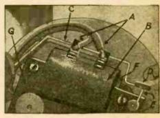
A-A.C. terminals. B-Field coil. C-Alarm striker reed. D-Alarm release. F-Bell.
