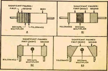
Resistance markings as used by both RMA and AWS codes. Note that body color is not part of the code in A—in the others, body color is one of the significant figures.
