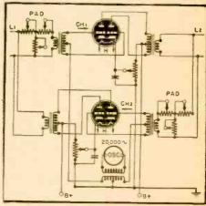
tion because of interaction. H. L. Donaldson of Chicago has a simple solution to this problem. A super-audible oscillation alternately biases each of the two amplifiers shown. In other words, channel 1 operates while Channel 2 is cut off during one alternation of the 20,000 cycle oscillation, and vice versa during the next alternation. Thus no feedback can occur. The high frequency does not interfere with the audio frequencies
