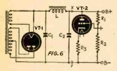
grid is made more negative with respect to the cathode. Accordingly, a certain amount of degenerative action and stabilization may be expected. In effect we have a shunt resistance across the output of the B supply, between the B plus and B minus terminals, consisting of the tube's platecathode resistance in series with R3. Somewhat better regulation may be obtained by substituting a special bias battery for R<sub>2</sub>, thus maintaining constant voltage between
