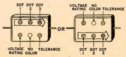
Basic 3-dot color code provides working voltage and tolerance indications. See Table 1.
