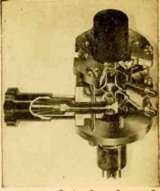
Courtesy Sperry Gyroscope Co. Cut-away shows Klystron's internal construction, co-ax leads and vernier tuning screw.
