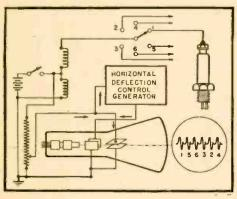
A voltage divider across the primary picks off a suitable voltage. This is applied to both sets of deflecting plates of the oscilloscope. In addition, the horizontal plates are influenced by a deflection control generator connected in series. The frequency of the latter is adjusted to the *nth* sub-multiple of the breaker point frequency, where n is the number of cylinders in the particular engine.
