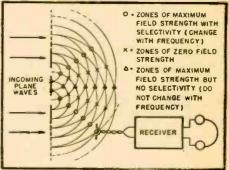
Incoming waves strike a metal baffle containing slits. Their width may be equal to the wave length of the signals and their spacing several times greater. As a result of spreading, cylindrical waves are formed beyond the baffle, resulting in weakening and strengthening of energy at different points, as shown. Positions of maximum and minimum strength will vary with the fre-
