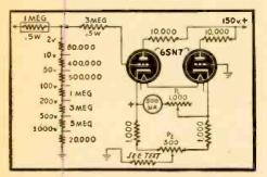
The balanced electronic voltmeter circuit.
