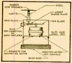
Fig. 3-Plan of the electrostatic modulator.
