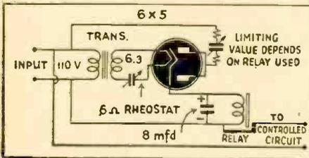
The rheostat should be one that will carry the filament current without heating up. The limiting resistor shown in the plate circuit of the rectifier tube depends on the relay used, and should be so chosen that the relay is not overloaded.
