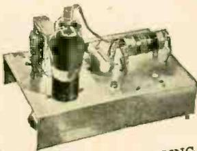
You build this **MEASURING INSTRUMENT** early in Course. Useful for work on Radios to make spare time money. It is a vacuum tube multimeter, measures A.C., D.C., R.F. volts, D.C. currents, resistance, receiver output.
