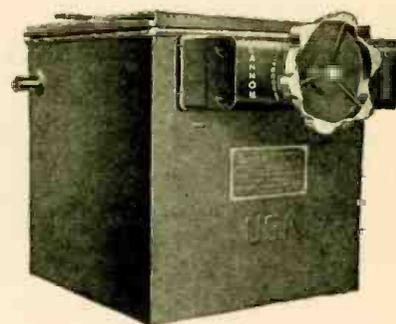
Receptacle No. 11749 also called the "Battery Kit" because it is affixed to the case, is made of aluminum alloy, finished with black acid-proof lacquer. The two pin contacts are leaded copper for 12-24 volt rating, 600 amperes continuous duty.
