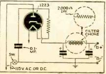
Fig. 4. The rectifier and filter circuit.
