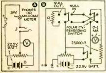
Fig. 6. Measures A.V.C. circuits accurately
