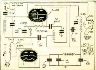
Fig. I. A simple but effective converter circuit is used.
