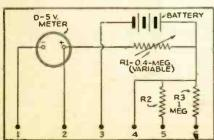
Fig. 5. Versatile home-made test meter.
