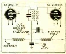
Fig. 2. Airline 62-106; replace shorted 0.1-mf. condenser with one rated at 600 W.Y.
