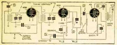
Fig. 1. Typical circuit of a midget A.C.-D.C. receiver.
