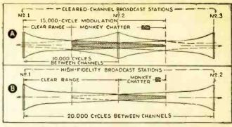
Fig. 2. Crosstalk ("monkey chatter") may be heard between stations 10 kc. apart if the modulation exceeds 5,000 cycles-per-sideband, as shown at A; (note that cleared-channel stations in practice are spaced 50 kc. apart and hence are unlikely to interfere). At 8, this proximity has been redded to nil by carrier allocations that are not less than 20 kc. apart.
