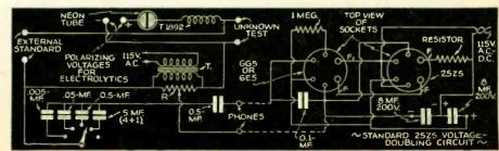
Fig. 2. Affords visual indication of bridge-circuit balance in a condenser
