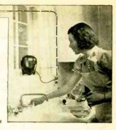
ERE, illustrated above, is a variation of the wired-radio type of inter-communicator, in which only 1-way operation is possible, which Radio-Craft has termed the "Wired-Radio Nursemaid."
