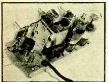
Figure B. This is the compact chassis of the 5-meter converter. It supplies its own operating power.
