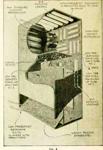
Phantom view of Bi-Fonic Reproducer; sound is reflected, not absorbed.
