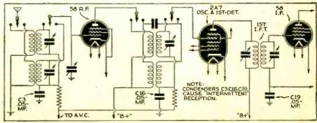
Fig. 1. RCA-Victor Models 121, 122; intermittent reception traced to open 0.05-mf. bypass condensers in the grid-return circuits of the Antenna, R.F. and 1st 1.F. circuits.
