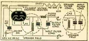
Fig. 2. Typical power-supply circuits of A.C.-D.C. sets.
