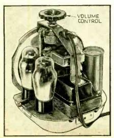
Fig. B. Interior view of the "Radio Nurse" or loudspeaker unit. This is an upside-down position, since the volume control operates from below.
