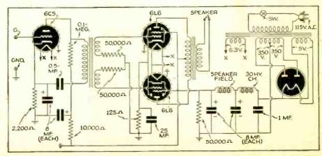
Fig. 3. Circuit of a high-fidelity amplifier which will do justice to the quality of the signal obtainable from the high-fidelity tuner.
