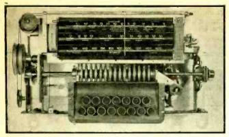
Fig. B. Front view of the Stewart-Warner electro-mechanical pushbutton tuning mechanism . . . a marvel of mechanical ingenuity.
