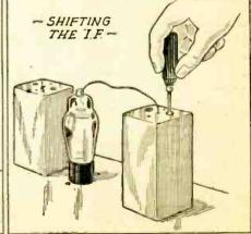
Fig. 1. Service Men are equipped to modify older sets to receive WOXR (New York), KPMC (California), KXBY (Missouri), and WBRY (Connecticut). As shown, the job may entail (A) trimming for higher frequencies, (B) carefully removing turns from coils, or (C) shifting the I.F. to a slightly different frequency.
