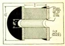
Fig. 2. Winding data for inductance used in the bass-compensated volume-control circuit.
