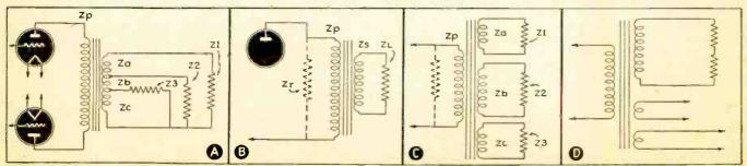
Fig. 1, "Equivalent diagrams" of effective impedances. A—3 magnetic loudspeakers, 2 standard dynamics and 1 large dynamic, connected to single, tapped secondary; B—glaring example of "mismatched" impedances; C—matching assorted speakers to multi-secondary transformer; D—showing importance of reflected impedances. In general, Zs indicates impedance of any one seç. tap; Zo, load imp. on or across it; and Zr, reflected toad imp.
