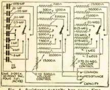
Fig. 4. Resistance-capacity box saves time.
