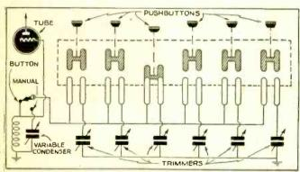
Fig. 15. A typical pushbutton assembly of the circuit-closing type.
