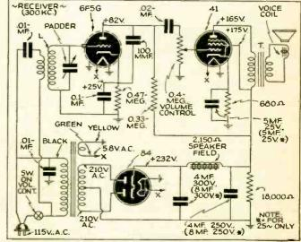
Fig. 2. Diagram of the "Radio Nurse" or reproducing unit shown, in Fig. B, on pg. 53. The volume control knob which extends out of the bottom of the bakelite shell of the Nurse is adjusted until the tick of a watch laid on top of the remote "ear" can be heard loudly. The electric light wiring automatically supplies the required "connection" between the 2 units.
