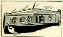
ZIPI, and this new car aerial extends to a height of 4 ins.; zipi, and it recesses to nearly cowleight (arrow, insert). Note control knob below car's Instrument panel (see drawing, above). (1630)
