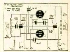
Schematic circuit of the Hammarlund unit-type ama-teur radio transmitter illustrated photographically and described on pg. 33. This factory pre-design of the assembly helps insure best results. (1623)
