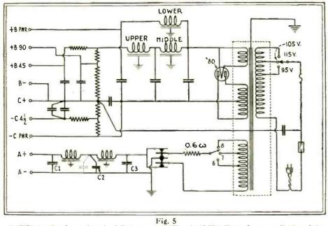
"ABC" six-volt tube-supply unit of Fada types and "82-11"," illustrating an application of the Fada types "86-1" and "82-H 1500-mf, dry ".1" condensers.
