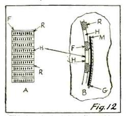
While the mesh-unit principle is illustrated here, the vidges between the "piston-vents" illustrated here are not of the best shape. It is an early model.
