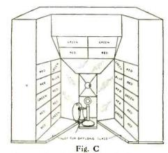
The grouping of the color filters, in front of the color-sensitive photoelectric cells, is shown in this perspective sketch of the television transmitter.
