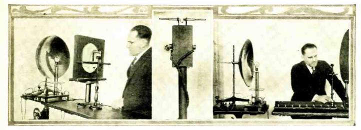
Fig. 1 The tube is emitting ultra-short waves which are reflected, just like light, through the lens in the center, to a glass of water, and thenee to the little receiver. Fig. 5 A close-up of the antenna and detector of the 14-cm. radio receiver.
