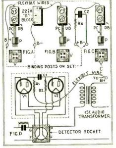
(Q. 37) The layout of ports and the alternative hook-ups of the "Detector Booster" are indicated in the above picture layouts (A, B, C) and schematic diagram (D).
