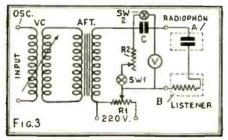
An experimental circuit, with controls designed to test the characteristics of the "Radiophan," To be exact, the listener is one plate of the condenser, as well as a resistar.
