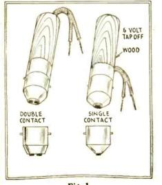
Fig. 1 A simple tap to the automobile storage battery will operate a receiver efficiently.
