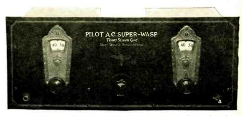
The attractive appearance of the "A.C. Super-Wasp." in its metal-paneled cabinet, is shown above. The jack permits the use of phones, which are desirable for tuning, as well as a lond speaker.
