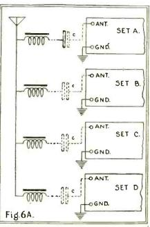
Multiple reception. In this illustration the Multiple reception. In this illustration the center-resonance coils have been placed in non-inductive relation to the grid circuit induc-tances; the coupling which takes place is almost entirely by the coil-to-coil capacity afforded.
