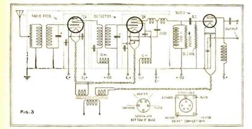
This circuit illustrates two applications of A.C. screen-grid tubes: transformer coupling has replaced the tuned impedance in the R.F. coupler, Note the type '24 detector, (Primary of second R.F.T. has about one-third the number of secondary turns.) For satisfactory operation it is necessary to use extremely high plate-circuit impedance; in the audio input, a 500-henry choke (A.F. transformer secondary) is recommended by the author.
