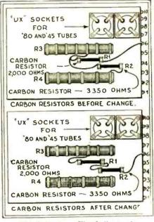
Fig. 2 (top) Fig. 3 (bottom) The original connection of the Radiola "44" power pack above: the later connection is aboven below.
