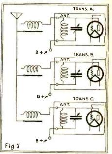
Multiple transmission through a single antenna is obtained by the use of verve-resonance coils for couplers. These pass only the frequencies to which they are tuned.
