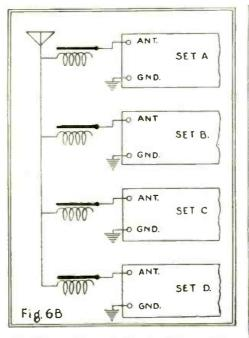
Multiple reception. In this circuit the coupling takes flace in a ratio somewhat different from that which obtains in Fig. 6.4.
