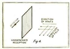
When this frame of parallel wires, at right anales to the front, is perpendicular 20.02.0 allows the waves to pass the electric field, it freely.
