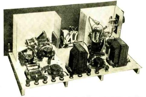
The chassis of the "A.C. Super-Wasp" without power pack. The manner in which the special shields are separated into halves facilitates assembly. The difference in layout from the D.C. model is slight, but incorporates some advantages. Additional by-passing is required by the use of biasing filament-return resistors; and special chokes are used in the plate and screen-grid leads of the '24 tube.
