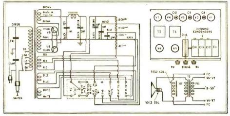
Power-pack parts layout and reproducer connections of the Steinite "50.4" and "102.4."
