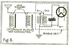
A wave-trap effect, obtained by use of the waveresonance coil. This arrangement is quite un-like any other "wave-traps," in both theory and performance.
