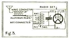
This is a recommended method of connecting a wave-resonance coil
