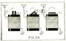
When the rotable (tickler) coil in the detector's in new the volume (tester) continue detectors splate eivenit is at C1, reception is normal; at C2, it gives regeneration and sensitivity in-creases up to a "spill over." elt C3 it makes the circuit oscillate and radiate a disturbing signal S2
