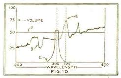
Selectivity may be advanced to the point of distortion: static is, however, thus excluded except on the narrow vereband the circuit passes. (A, static; B, surge; C, program; D, good volume.)
