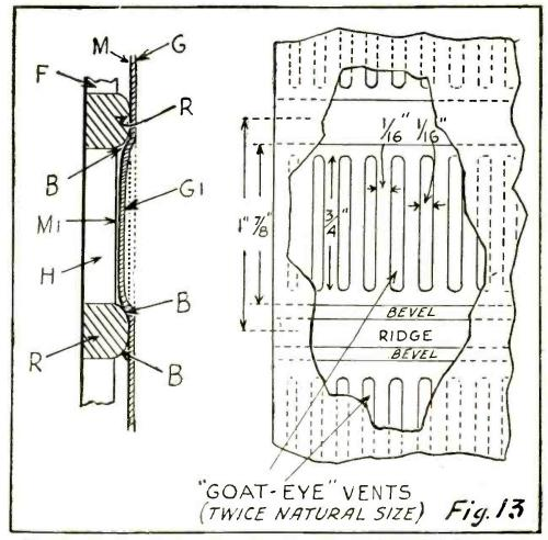
The construction of a mesh-unit reproducer shown above, with a flat fixed electrode F, is very easy; but the result will be imperfect and buzzing reproduction. The reason is that the plate voltage pulls the diaphragm into a convex shape, instead of permitting it to remain flat. The principal attraction is toward the shoulders B-B.
