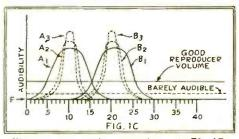
With the same station separation as in Fig. 1B, the greater selectivity obtained from additional tuned R.F. circuits B2 and B3 permits londer reproduction with less interference.
