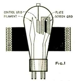
As screen-grid tubes acquire a silver-like interior surface during evacuation, it is difficult to visualize the interior construction. The relation of the four "elements" is shown in this figure.
