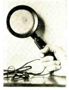
Fig. A One model of the "Radiophon," showing the reproducing surface above the handle.
