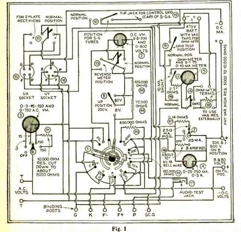
Schematic circuit and connections of the Portable Radio Testing Laboratory.
