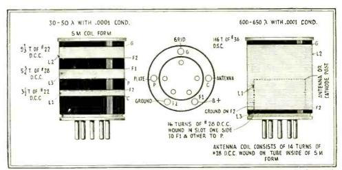
Those of our readers who have inquired the coil specifications of the long- and short-wave receiver used by KIK, as described by Mr. Brauner in our November issue, will find them here. The larger coil adapts a short-wave set to ship's calling wave. The coil form is 2% inches in diameter.
