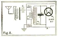
Capacitative coupling of the wave-resonance tuner, in place of the usual antenno lead, to the first radio-frequency stage.
