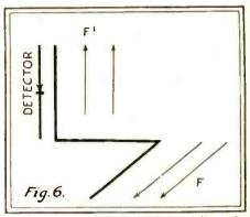
The heavy line indicates the short coupling rod, which would pick up a signal in one of its sec-tions; and, by the flow of current, transfer the signal to the detector.
