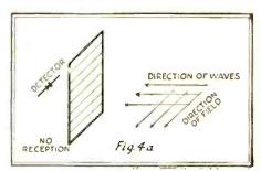
If, on the other hand, the wires of the Hertz "polarization grid" are turned until they parallel the electric field, they shield against it.
