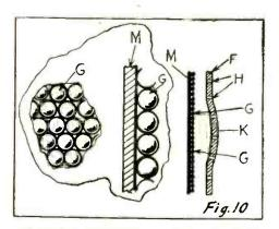
The Reisz elastic-diaphragm speaker, in which one plate is formed by conductive granules imbedded in an insulator, yet free to more otherwise.
