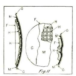
In the Reisz unilaterally-driven reproducer, above, the "fistan-vents" are circular holes punched through a convex, saucer-like dise of metal, vehose thickness is exaggerated here.
