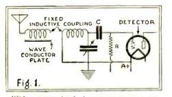
With a strong signal, the wave-resonance tuner, indicated by the special symbol at the left, may be coupled inductively to the grid circuit of a detector effectively. This circuit is selective.
