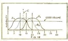
With one tuned circuit, two stations fully ten kilocycles apart interfere; a lessened separation, as at B2, causes high continuous whistles.
