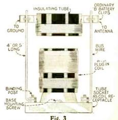
Fig. 3 A tube-base plug-in coil is easily equipped with an adjustable winding in this way.
