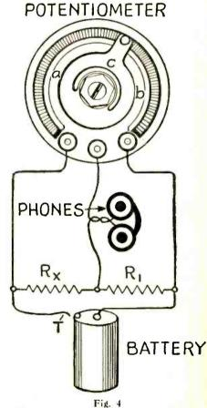
This simple kink provides a bridge circuit whereby a resistor's approximate value may be determined, with a potentiometer whose resistance strip is evenly wound.
