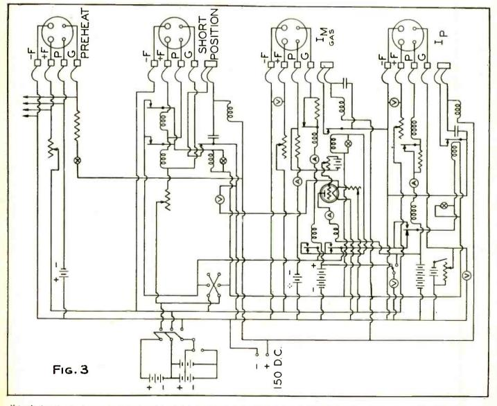
Not only does the circuit above look complicated, but it is! It is that of a large testing machine which tube makers use to sort out defective tubes on com-pletion of the processes of manufacture. A great many mechanical features are incorporated in the design, but cannot be shown here; the relays (here shown as meters) close other circuits which work the ejectors that throw out all tubes whose test readings depart from the standard too much, either above or below the limits of tolerance.
