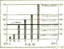
Taking the "signal level" as 30, and "static level" as lettered, interference has the effect shoron; a powerful local signal also may paralyze the first R.F. tube.
