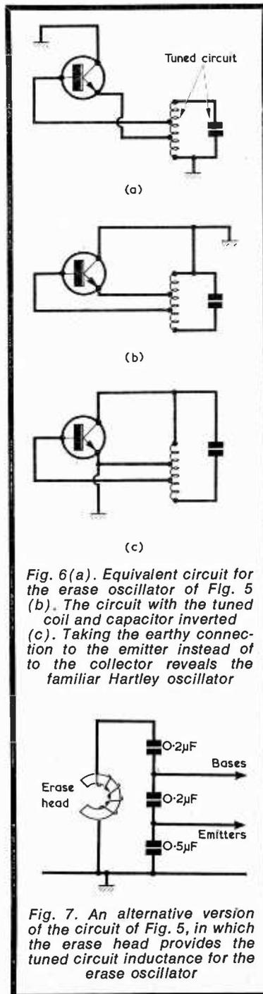
Fig. 6(a). Equivalent circuit for the erase oscillator of Fig. 5 (b). The circuit with the tuned coil and capacitor inverted (c). Taking the earthy connection to the emitter instead of to the collector reveals the familiar Hartley oscillator
