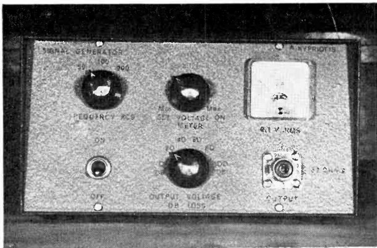
Front view of the prototype unit. S1 is at the top left, R25 is at top centre and S2 is at bottom centre
