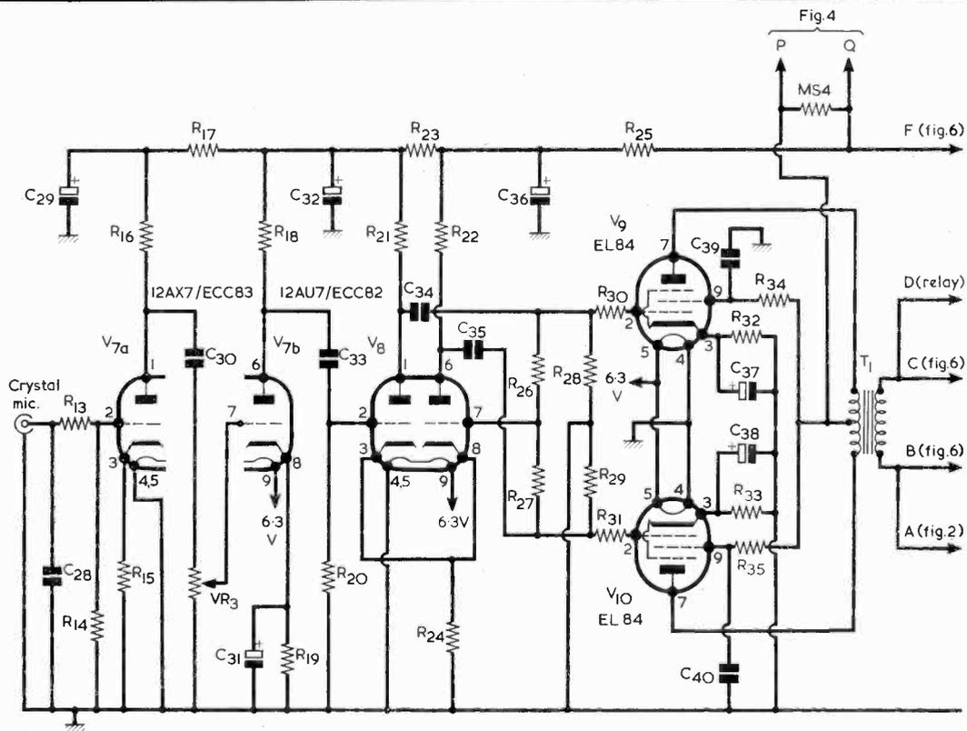
Fig. 3. The modulator amplifier
