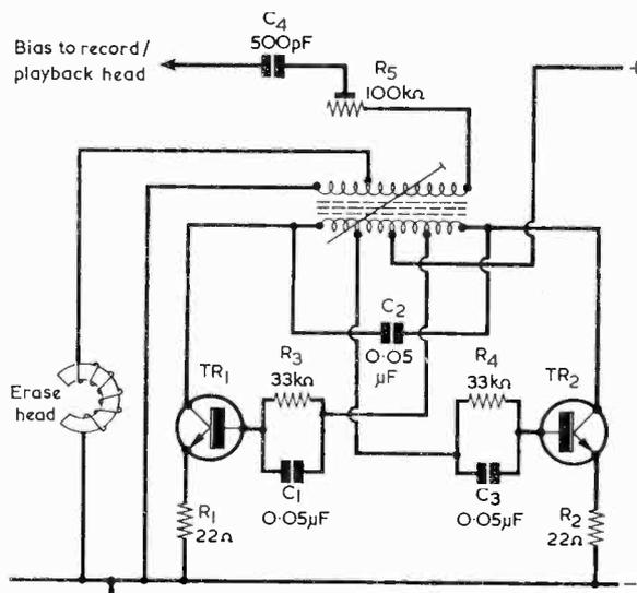
Fig. 4. A push-pull erase oscillator circuit
