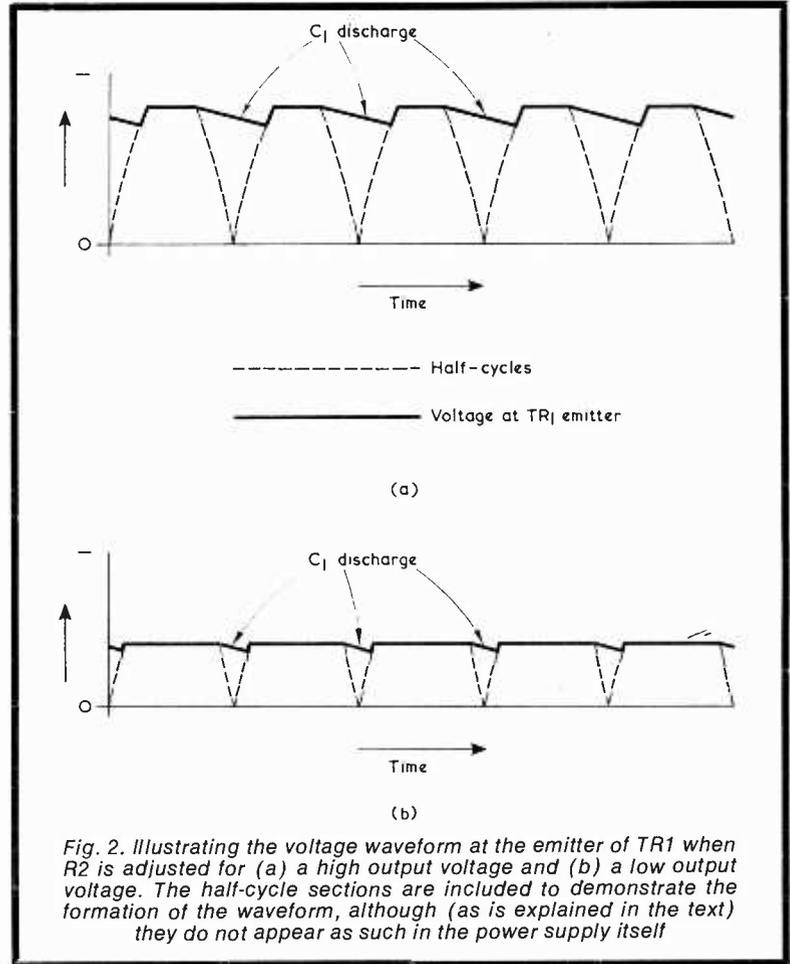
Fig. 2. Illustrating the voltage waveform at the emitter of TR1 when R2 is adjusted for (a) a high output voltage and (b) a low output voltage. The half-cycle sections are included to demonstrate the formation of the waveform, although (as is explained in the text) they do not appear as such in the power supply itself
