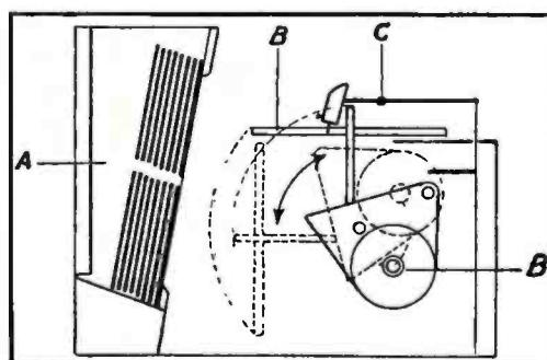
**Fig. 3—Step two: turntable rotated 90 degrees and record ejected from magazine.**
