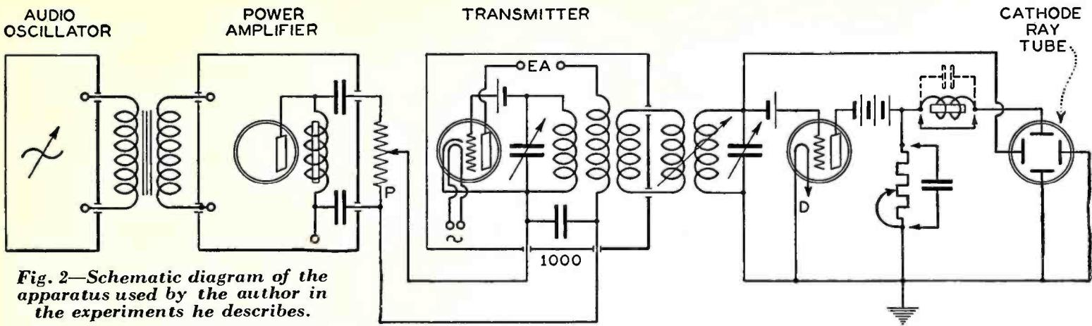
**Fig. 2—Schematic diagram of the apparatus used by the author in the experiments he describes.**
