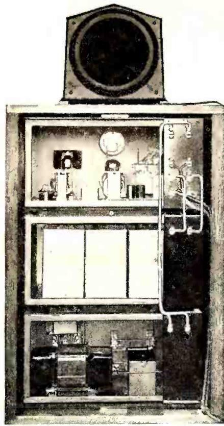
Rear view of audio-frequency voltmeter.
