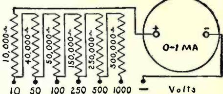
The Super Akra-Ohm wire-wound Resistor is especially adapted for use as a Voltage Multiplier as shown in the above diagram. It is carefully designed to insure an accuracy of 1 per cent and a constant permanency of calibration. Its use is also highly recommended for Laboratory Standards, High Voltage Regulators, Telephone Equipment, and Television Amplifiers, Grid and Plate Resistors, etc.
