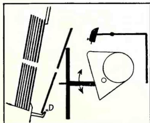
**Fig. 5—Step four: turntable rising to play record.**
