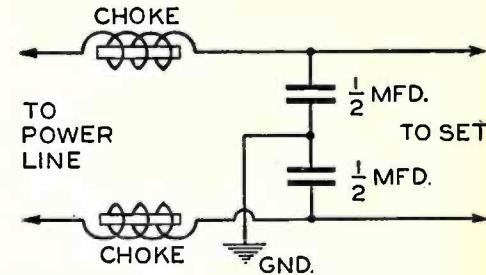
Fig. 2—Using r.f. chokes for additional filter action.
