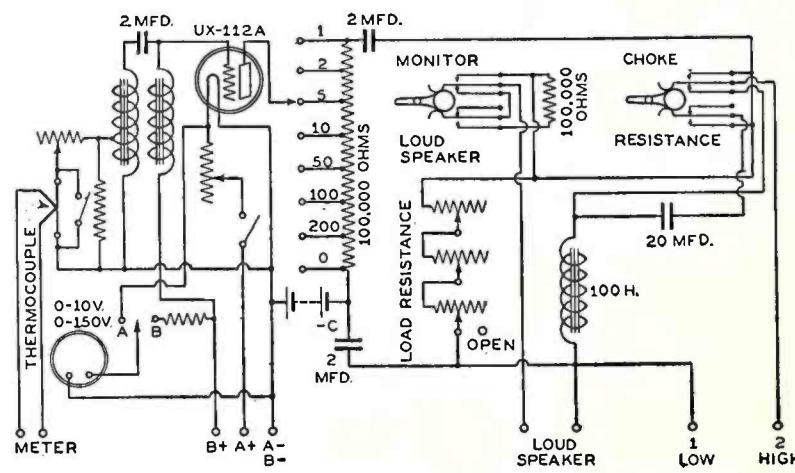
Fig. 1—Circuit of A.F. voltmeter and loading device.
