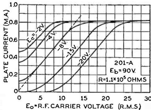
The curves on this sheet are for a 201-A-type tube operated with a resistance load in the plate circuit from a battery potential of 90 volts. Five curves are shown for grid biases from -2 to -20 volts. These curves were made by measuring the plate current as the r.f. input voltage was gradually increased from 0 up to 30 volts. The plate currents obtained with the various input voltages were then plotted and the series of curves shown on this sheet was obtained.
