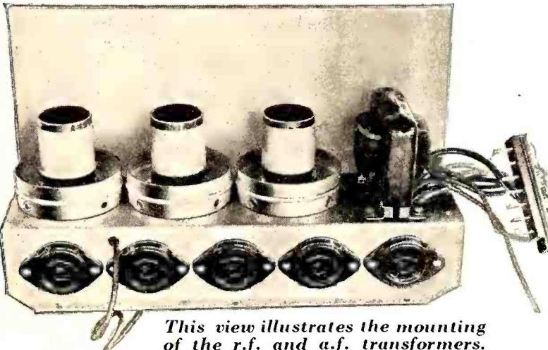
gasket to make it weatherproof. The cable to the set is again an armored one. The total filament current taken from the car's battery is 3.75 amperes.
