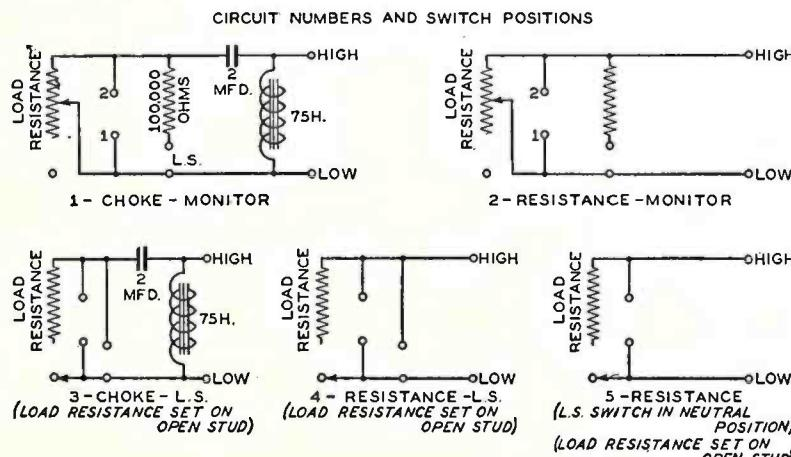
Fig. 2—Circuits obtainable with loading device.
