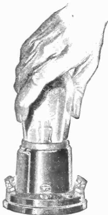
Socket instantly cleaned by twisting tube
