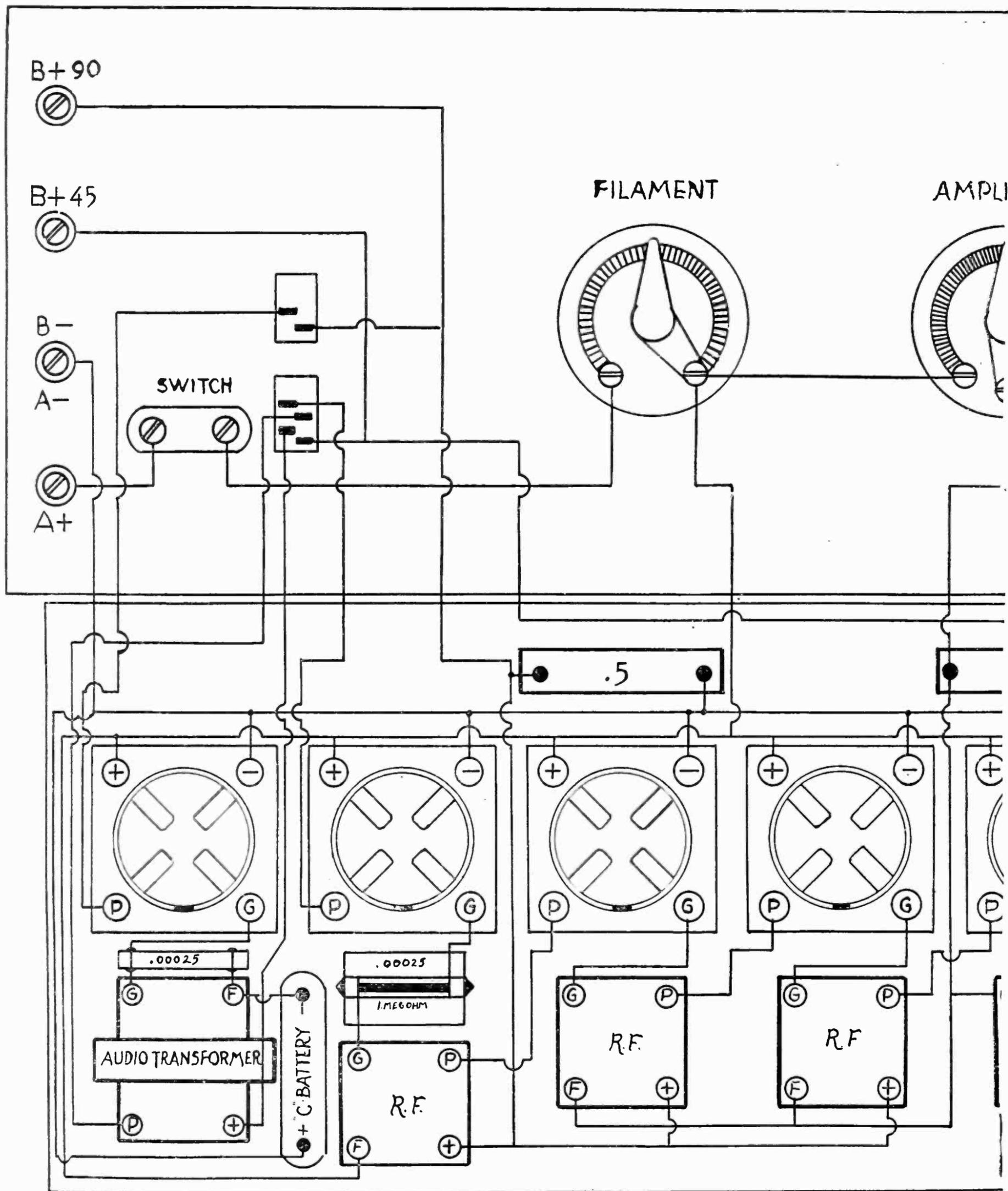
be much the sharper of the two in adjustment, although with a good loop its tuning condenser should tune fairly sharply. These two condensers must be varied more or less in unison, the general tuning practice being slowly to increase the oscillator control, or left-hand condenser, while the other condenser, which tunes the loop, is increased with it, or con-
