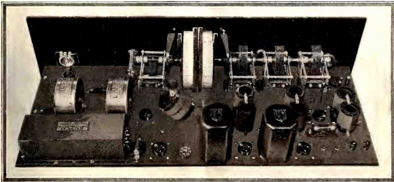
Showing complete built-up Camfield "10" Receiver
