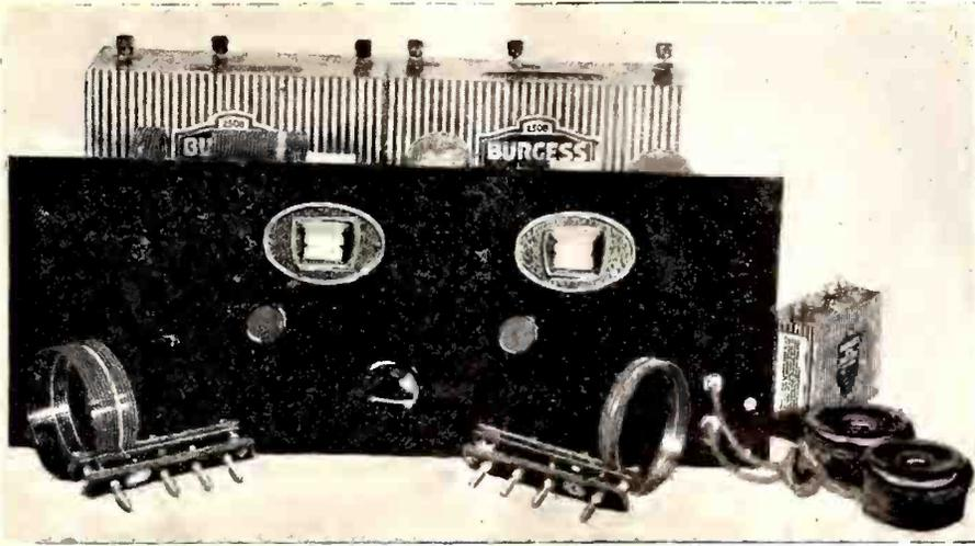
Front panel and some of the parts and accessories used in the Radio Age Short Wave Receiver
