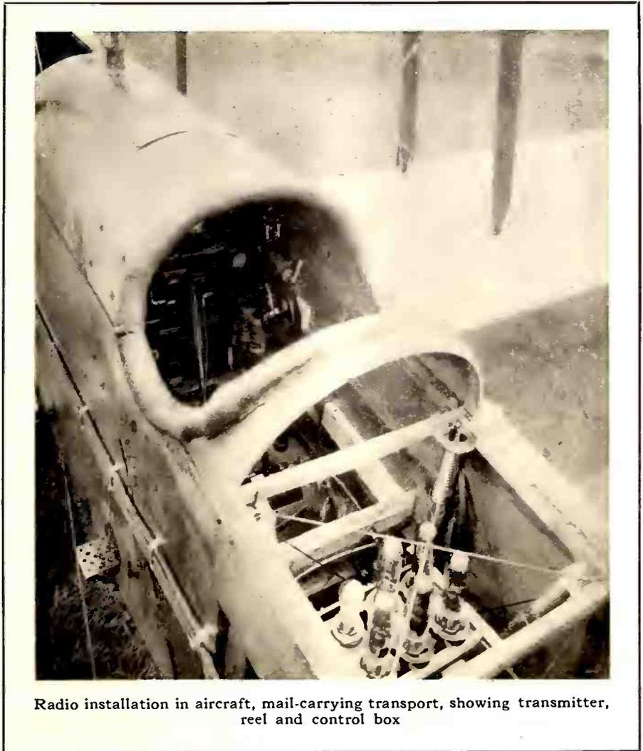
Radio installation in aircraft, mail-carrying transport, showing transmitter, reel and control box
