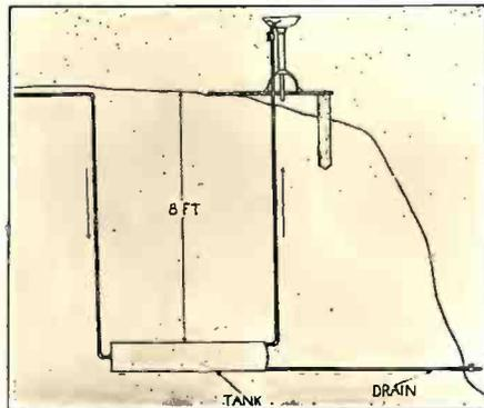
Several coolers of this type have been installed at the Fairlawn golf course near Akron, Ohio. Water from the surface sprinkling system often reaches a temperature near the boiling point, but after being passed through the tank it emerges from the fountain at about fifty degrees Fahrenheit.
