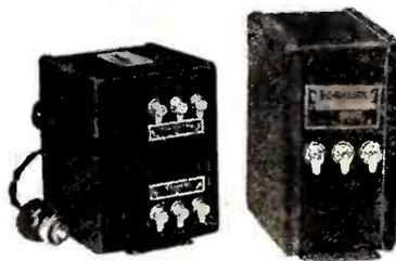
Here is a power unit that will satisfy the ever increasing demand for improved quality of reception. A split secondary 550 volts either side of center, makes possible full wave rectification, using two 216-B or two 281 tubes. Current capacity, 130 milli-amperes. The low voltage secondary, 7½ volts, will supply two UX-210 power tubes, enabling the use of push-pull amplification in the last audio stage.
