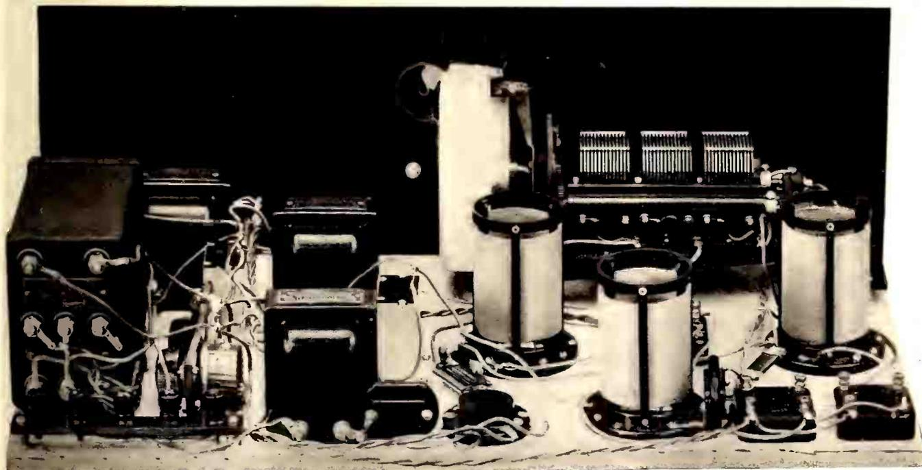
Rear View of A. C. Operated Receiver Showing Placement of Parts and Associated Wiring. The Set is Wired with Flexible Rubber Covered Wire, Simplifying Wiring and Construction. The 171 Bias Resistor and By-pass Condenser are Hidden from View Behind the Out-put Transformer.
