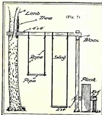
plank to the wheel. As a rule the plank should be at least three feet from the ground. The pipe lends stiffness which is desirable.
