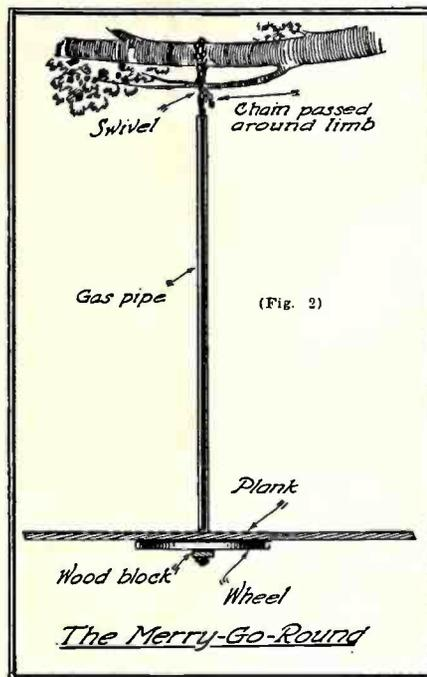
merry-go-round that is really different. Fasten a short piece of chain to a limb and attach a swivel to it, preferably with a ring. Attach a longer chain to this and run it through a gas pipe. Fit a large iron wheel with a plank on top onto the lower end of the pipe, setting it fast with a set screw. The lower end of the chain is kept from slipping up the pipe by tying or otherwise securing it to a block of wood or piece of iron.
