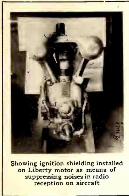
Showing ignition shielding installed on Liberty motor as means of suppressing noises in radio reception on aircraft
