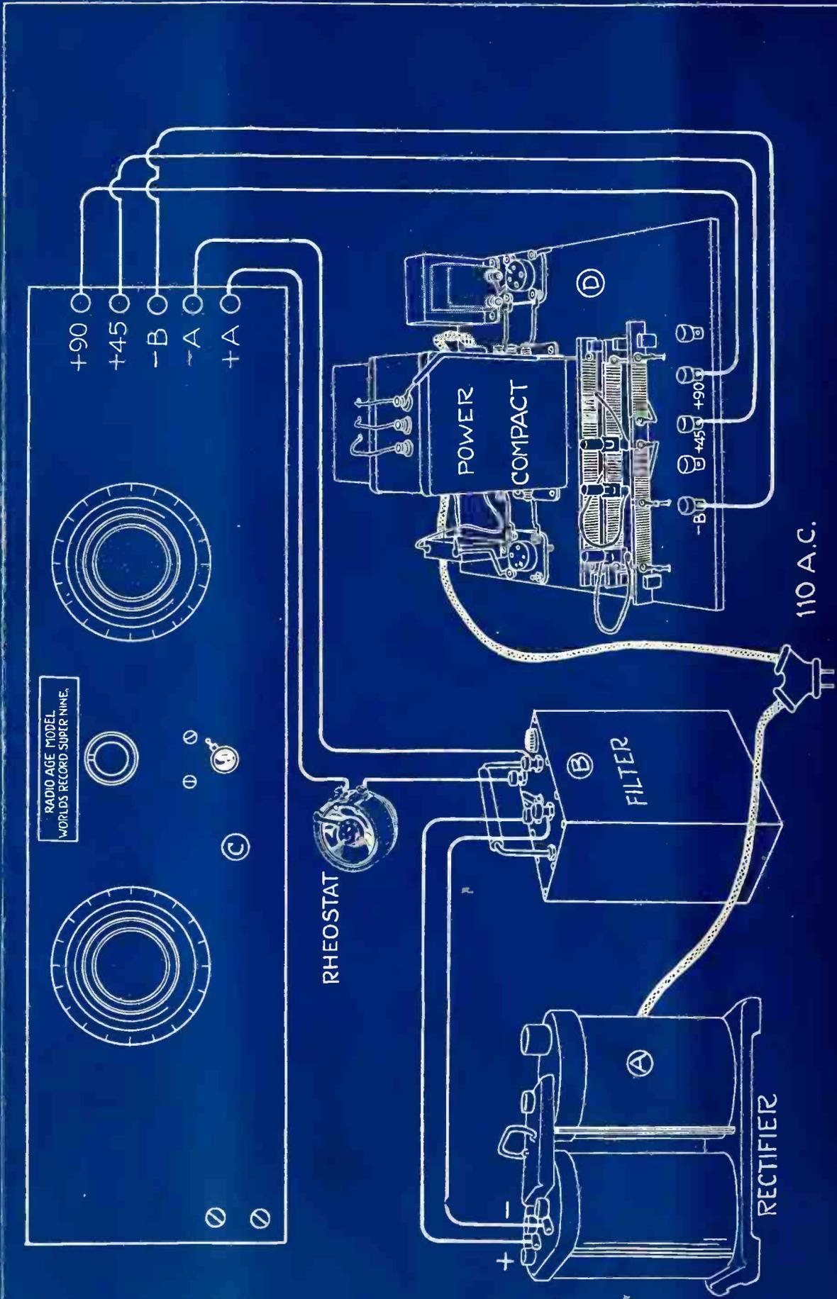
FIG. 3 PICTORIAL REPRESENTATION OF COMPLETE A, B, AND C, ELIMINATION SYSTEM USED WITH WORLDS RECORD SUPER 9
