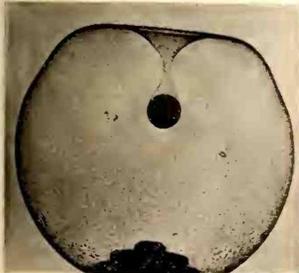
**STEEL BALL DROPPED IN A SOAP BUBBLE.** This photograph, made about a hundredth of a second after the ball first touched the bubble, shows that it has not yet begun to break, but extends down around the ball like an elastic membrane
