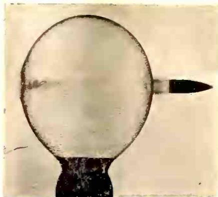
**THE BULLET AND THE BUBBLE** photogr aph made in the sound laboratory of the U. S. Bureau of Standards by means of an electric spark, by Philip P. Quayle, showing a soap bubble through which has been fired a rifle bullet. The bullet has passed out of the bubble, but it still stands, with a hole in each side. The lines extending from the front of the bullet are sound waves
