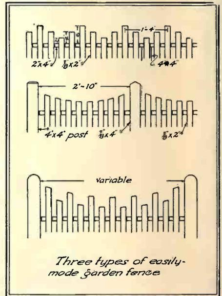
Although clear pine is the favorite garden fence material, pecky cypress is superior because it does, without the help of paint if necessary, withstand the inroads of rot. A home done in a gray stucco, or painted a neutral gray, will match ideally a pecky cypress fence because in a short time the wood, unadorned with paint, will assume a weathered gray effect, too. Of course the application of paint will give you any color you want.
