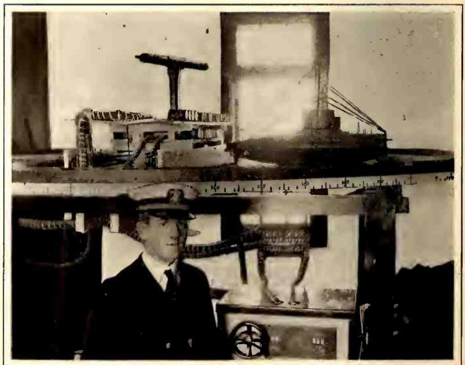
Naval radio direction finder with model submarine on test run
