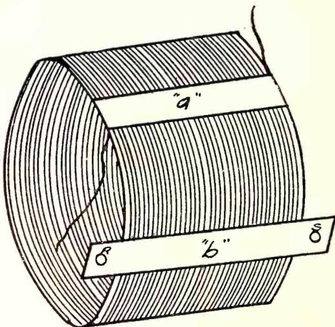
Fig. 2. "R" and "S" of section "b" are holes in mounting strip to take machine screws for fastening coils to mounting brackets
