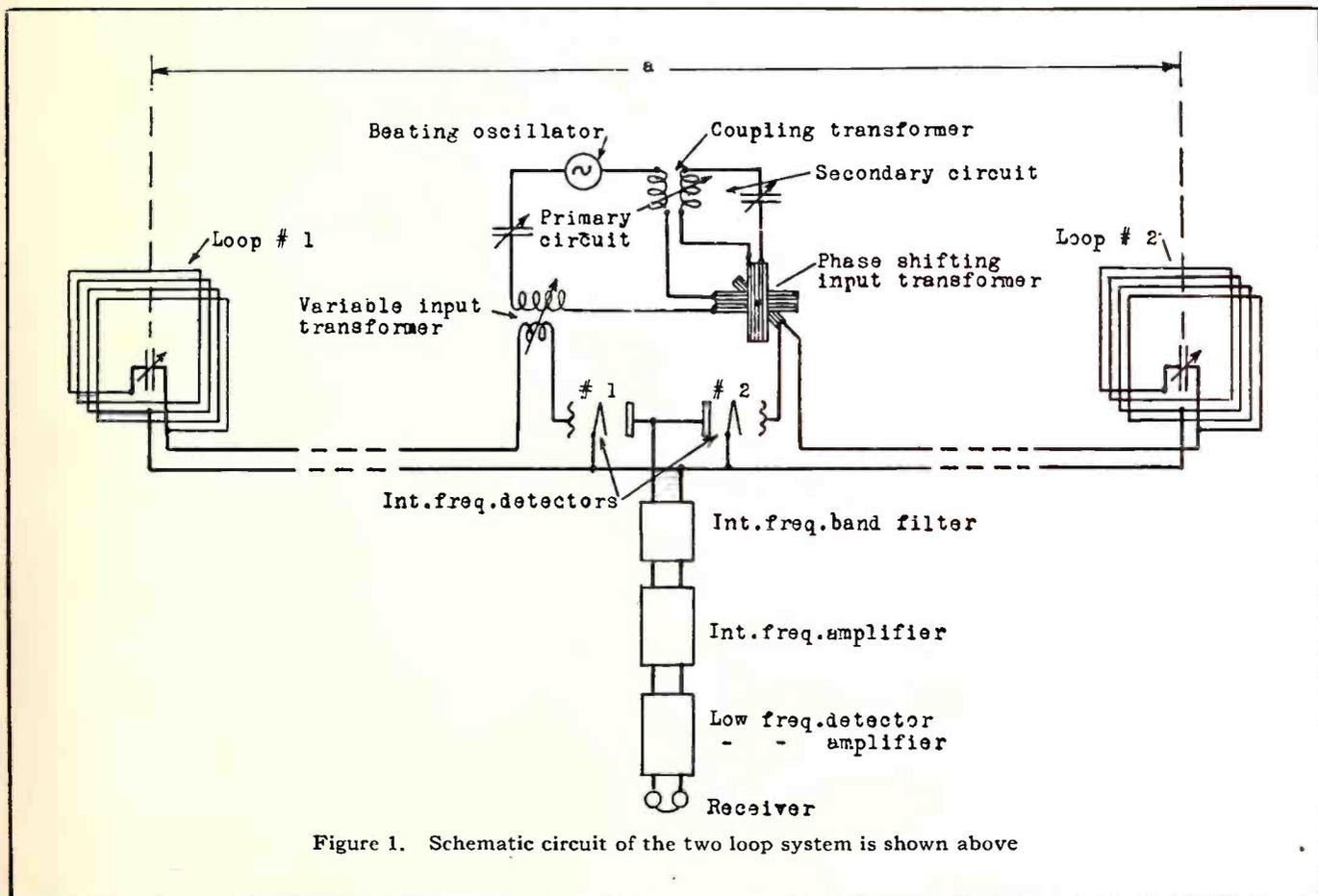
Figure 1. Schematic circuit of the two loop system is shown above
