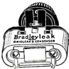
The accompanying cuts illustrate its appearance, which is very much like the familiar Bradleyleak filament control. The leak is variable continuously from about one-quarter to ten megohms of resistance, and can be used with any type of tube now on the market with perfect satisfaction.
