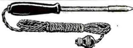
Test No. 3. Security electrical soldering iron No. 25. Made especially for radio work. Designed to reach heretofore inaccessible points of complex sets. A  $\frac{3}{8}$ " rod 5" long and with  $\frac{1}{2}$ " removable copper tie 2" long. Heating element of nichrome wire at tip where heat is needed. Flows solder freely. Guaranteed for one year and passed by Radio Age Institute Tests. Made by Security Electric Mfg. Co., Chicago, Ill.
