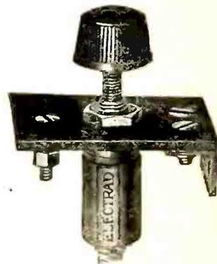
Test No. 6. Electrad Variable Grid Leak and condenser combined. A novel instrument that is attracting wide attention of fans who want compact parts. A perfect variable pressure Grid Leak,  $\frac{1}{4}$  to 30 megohms, together with special .00025 mfd. condenser. Practically no hysteresis losses noticed in special Radio Age Institute tests. Metal parts gold plated. Mounted on a bakelite panel. Made by Electrad, Inc., 428 Broadway, New York.
