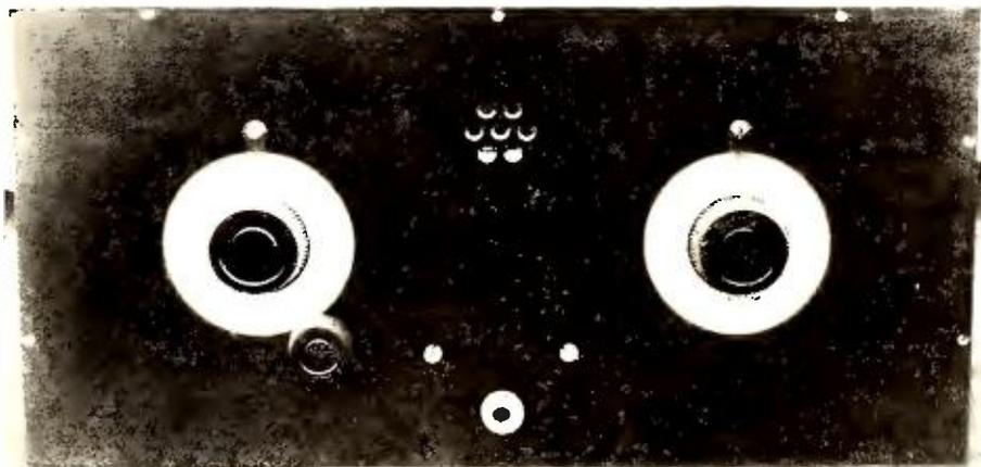
*Doesn't it look simple? The rheostat's inside and is always set at the right value. The tube lights when the phone plug is pushed in. The left hand condenser has a vernier control and accomplishes the tuning.*
