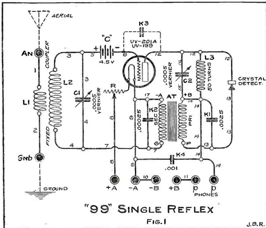
not permit of oscillating current flow in the opposite direction.
