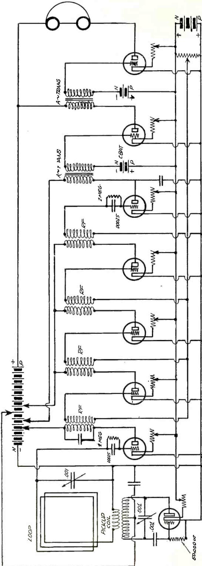
Figure 1. An eight tube Super-Heterodyne, the action of which is described by Mr. Peirce in the accompanying article. The action and rules governing the operation and design of super-heterodyne receivers are taken one by one and discussed frankly and clearly by our technical editor.
