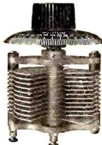
G. M. Proudfoot, engineer for the Cruger Manufacturing Company, has designed a new condenser for the purpose of reducing losses and inefficient capacities.
