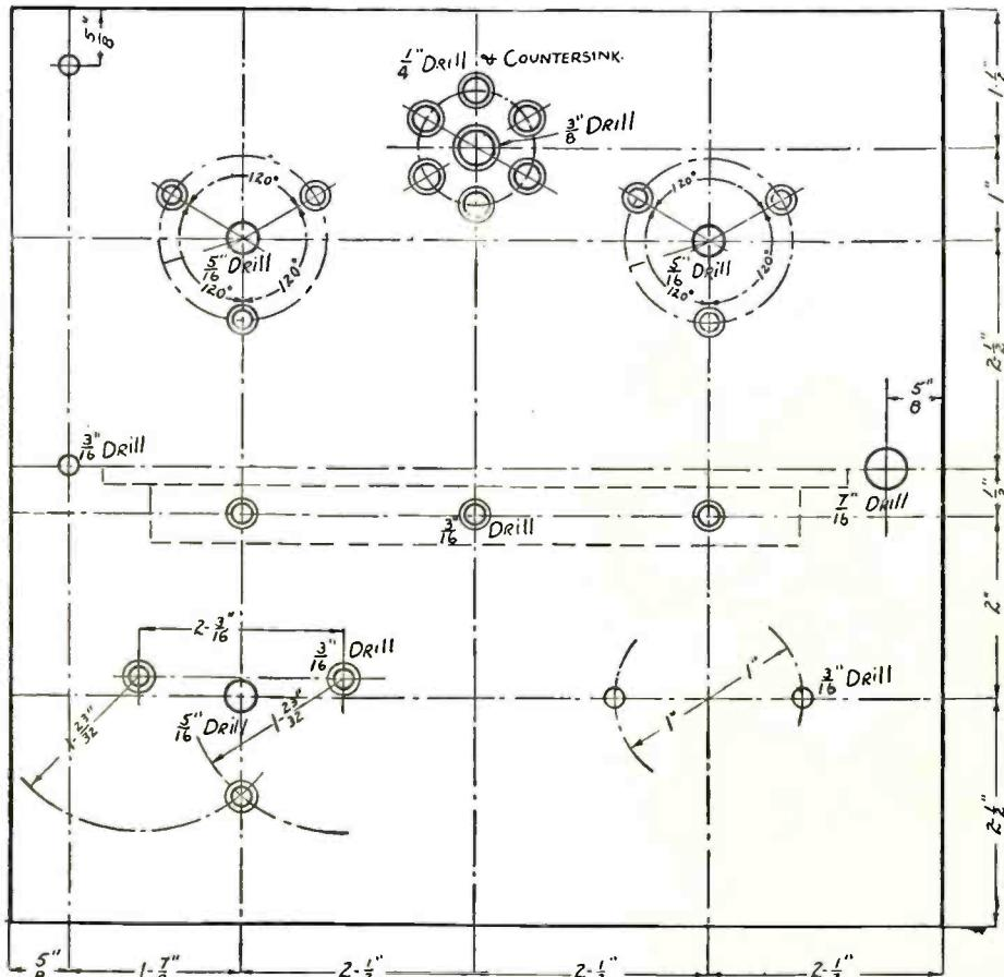
Figure 3. Template, drilling and layout instructions for the simple reflex described in the accompanying article.
