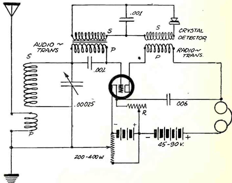
Figure 7. The wiring diagram of the Sure Fire Reflex Receiver.
