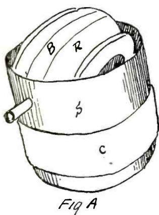
Figure 1c. Arrangement of the coupler and plate coils.
