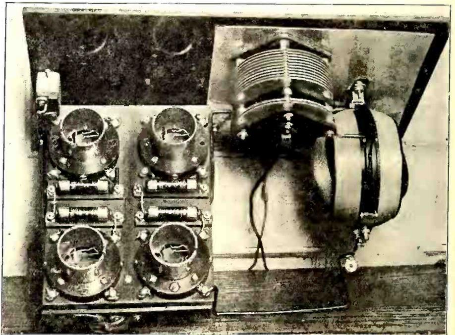
The above photographs picture a method used by a radio fan to eliminate controls for the filaments of the tubes. The cartridge types of resistance are of the proper value to be used instead of rheostats, thereby making the use of four extra controls unnecessary. The circuit is the conventional single circuit using a variocoupler as tuner. The panel view shows how simple the control of this set is. (Kadel & Herbert Photo.)
