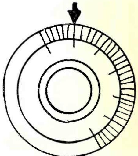
Figure 2. On homemade sets, the builder usually scratches an indicating mark on the panel. Here's another method of solving this really necessary operation.
