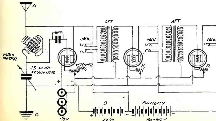
Figure 1. Using WD 11 tubes for amplifiers on the single variometer circuit. Note the connections on the dry cells which give the necessary extra amperage when more than
