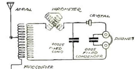
Figure 2. The Long Distance Crystal Hookup, which is giving very good results over extremely long distances. Tuning is accomplished with the variocoupler and variometer shown in the circuit.
