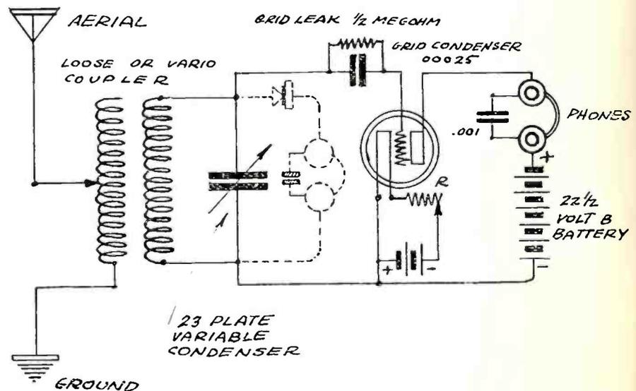
Figure 3. A two circuit crystal hookup can be remodeled into a one tube set with the few simple changes as indicated in the circuit diagram.
