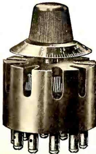
The amplitrol not only adjusts the filament to its maximum efficiency, but it also automatically switches on and off the plate circuit. Unlike automatic filament control, the amplitrol does not put a sudden strain on the filament. It provides a gradual current increase for the filament, prolonging the life of the vacuum tube at least one-third.
