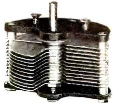
Variable condensers to be efficient must be well made. Loose joints or faulty construction soon allow the plates to get out of alignment and decrease their efficiency.
