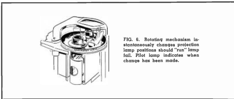
FIG. 6. Rotating mechanism instantaneously changes projection lamp positions should "run" lamp fail. Pilot lamp indicates when change has been made.
