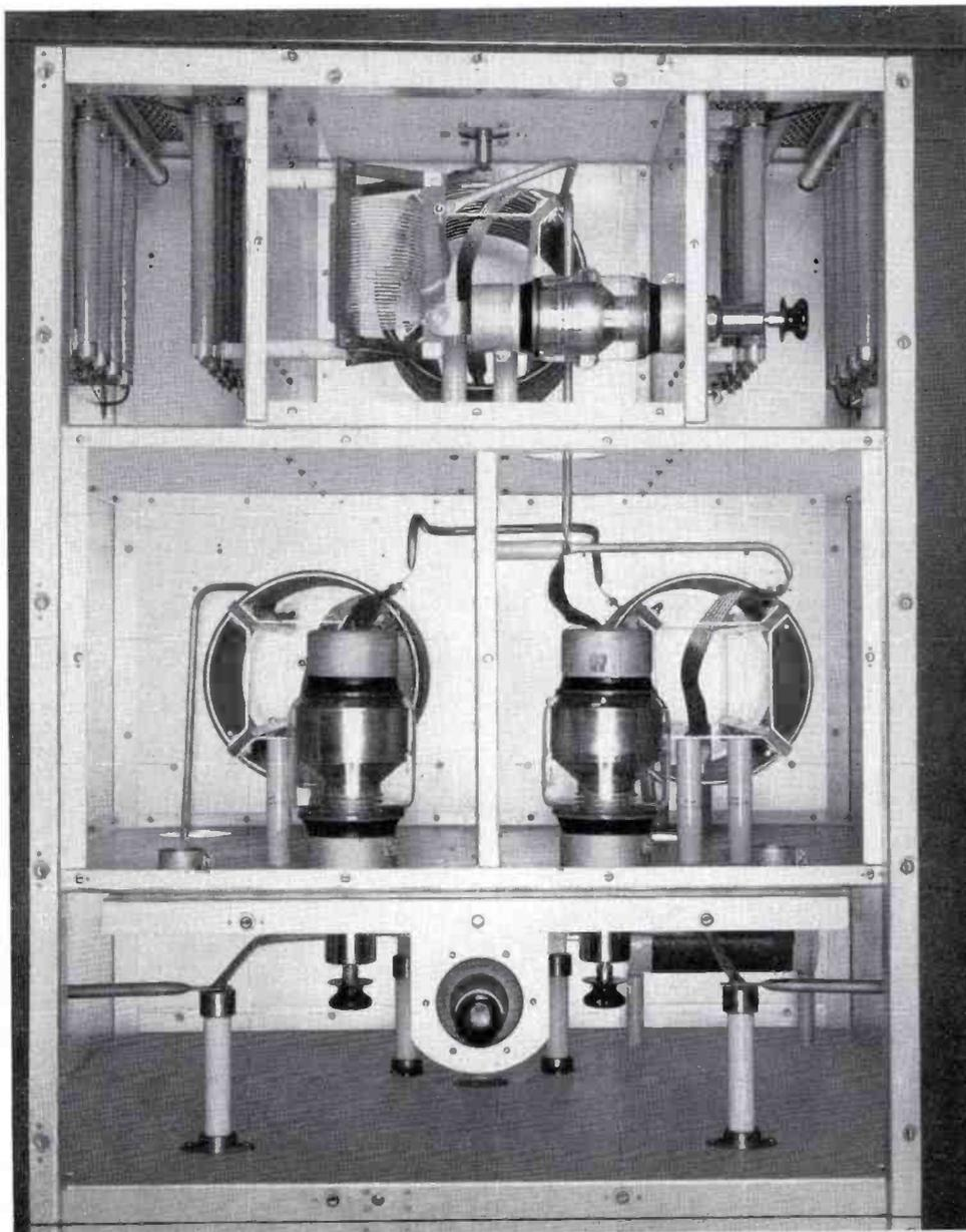
FIG. 11. Rear view of Exciter-Modulator cubicle showing combining network and harmonic filter components.
