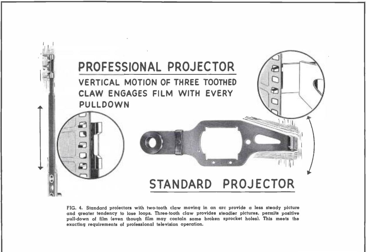
FIG. 4. Standard projectors with two-tooth claw moving in an arc provide a less steady picture and greater tendency to lose loops. Three-tooth claw provides steadier pictures, permits positive pull-down of film (even though film may contain some broken sprocket holes). This meets the exacting requirements of professional television operation.
