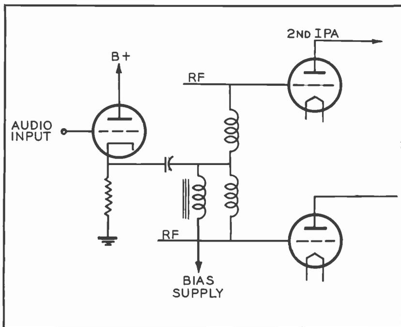
FIG. 12. Simplified circuit of Drive Regulator.
