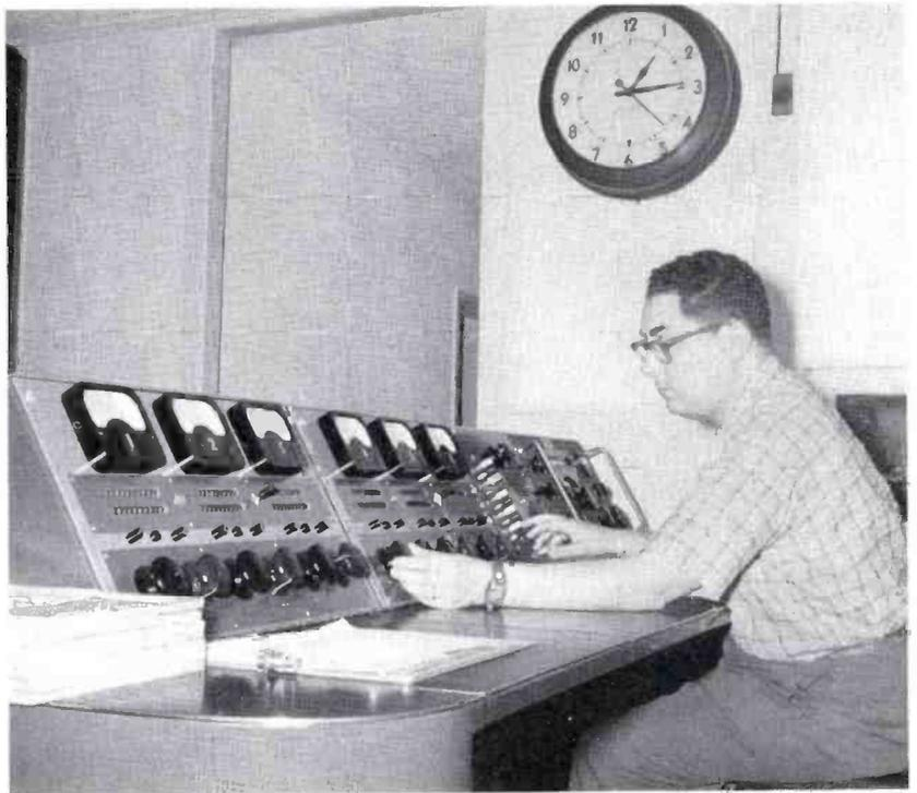
FIG. 32. Audio control at Maxoqueira handles incoming program circuits from Germany.
