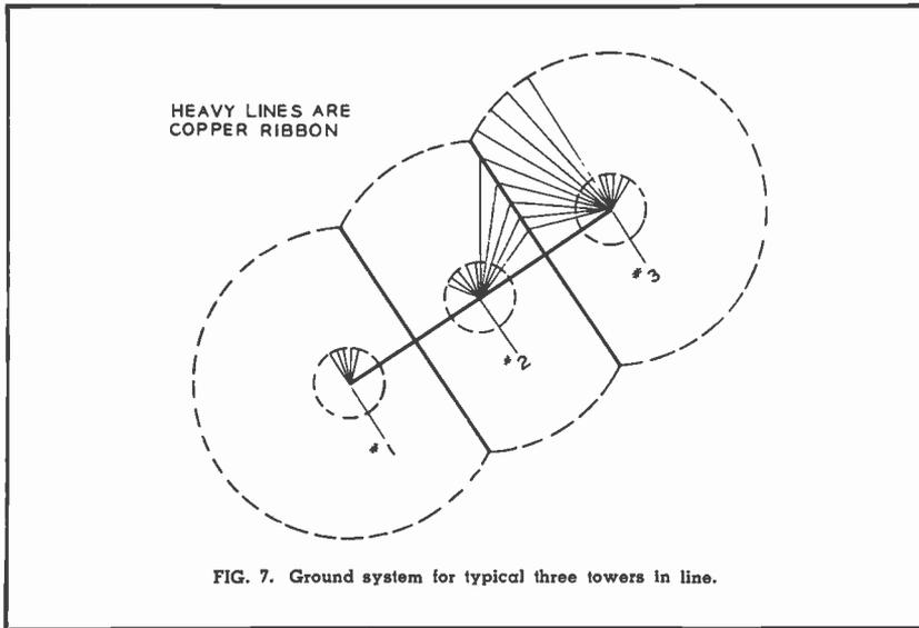
FIG. 7. Ground system for typical three towers in line.
