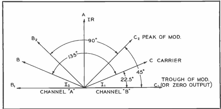
FIG. 6. Ampliphase vector diagram.
