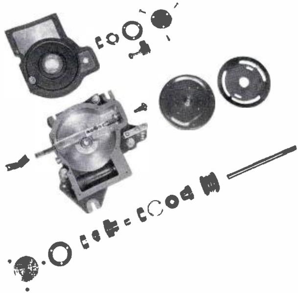
FIG. 3. Exploded view of the intermittent mechanism which permits claw to move straight up and down, engaging the film to its maximum extent.
