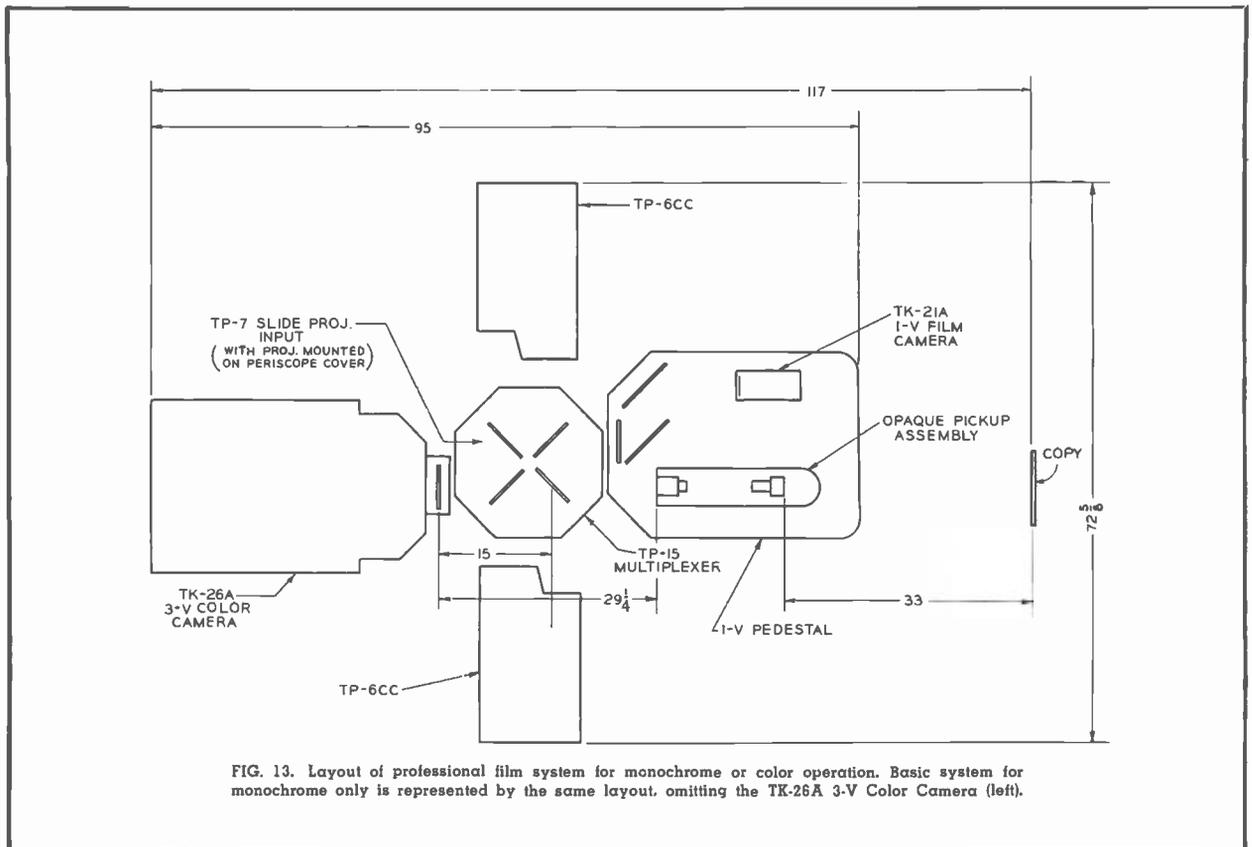
FIG. 13. Layout of professional film system for monochrome or color operation. Basic system for monochrome only is represented by the same layout, omitting the TK-26A 3-V Color Camera (left).
