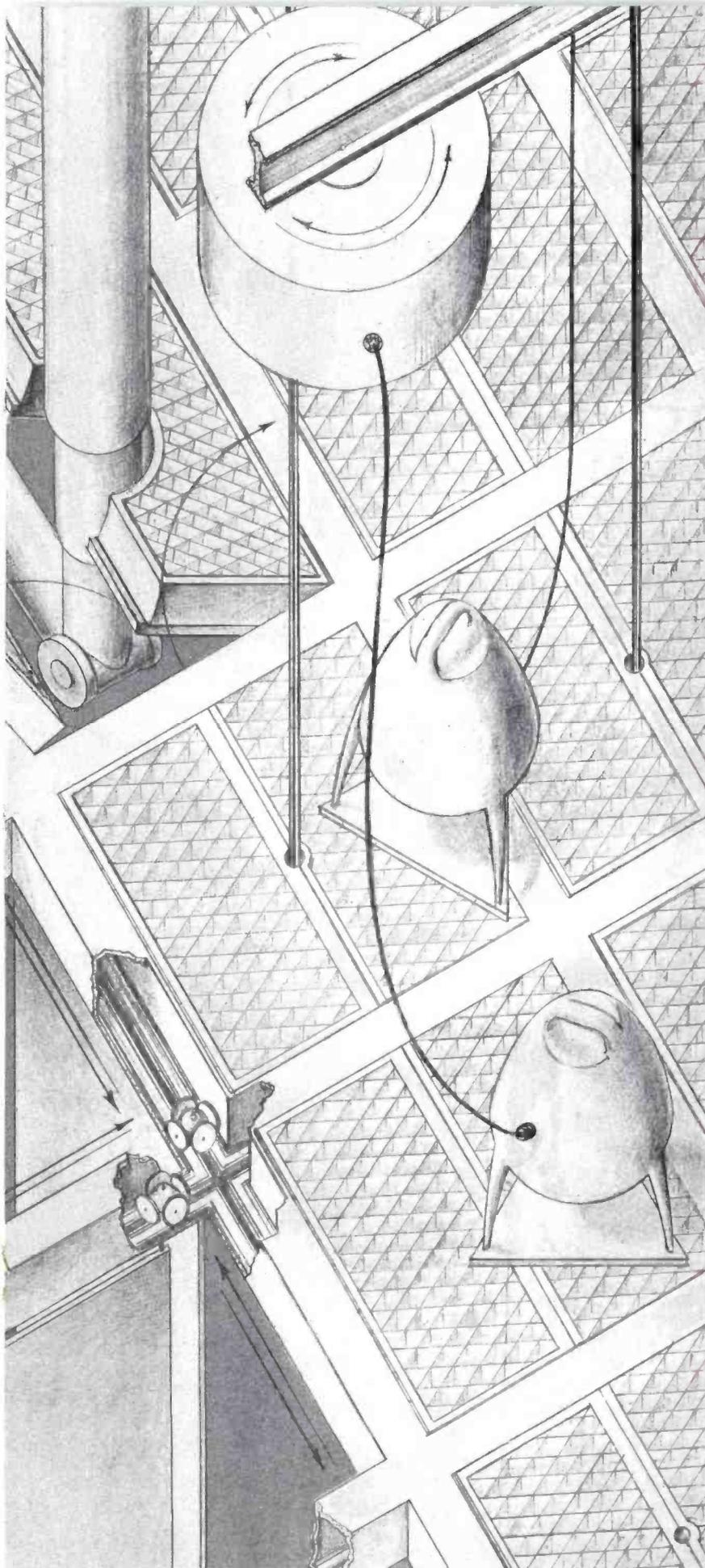
*Lighting, Camera and Microphone* equipments mount on ceilings above the grid and project through it for use in the studio, thereby clearing the studio floor for the performer. The equipments rise into the floors above for maintenance and repair, without immobilizing the studio for these activities.
