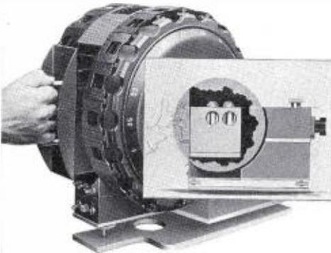
FIG. 11. Quick lamp change feature of the TP-7. Spare lamp can immediately be moved into place by pulling handle as shown.
