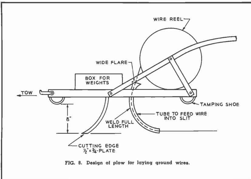
FIG. 8. Design of plow for laying ground wires.
