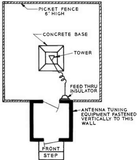
FIG. 2. Plan view of the antenna tuning house.
