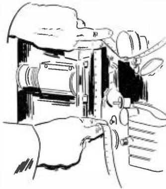
spot. The claw-type intermittent can be serviced in the field, while the sprocket-type must be returned to the factory for servicing.
