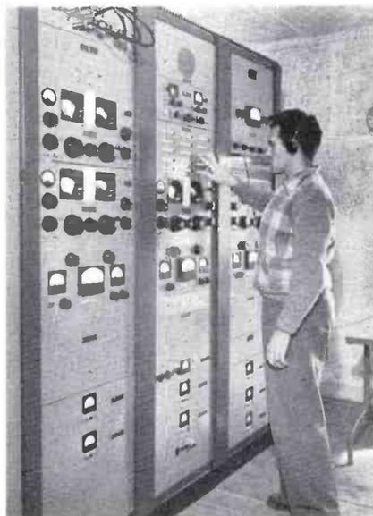
FIG. 33. Typical triple diversity receiving system used at Maxoqueira.
