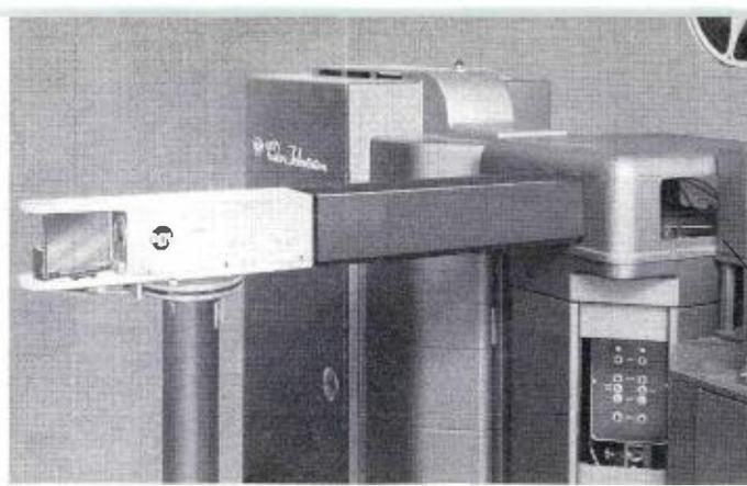
FIG. 12. Opaque pickup assembly for television flip cards, small packages and products may be used for color or monochrome presentations.
