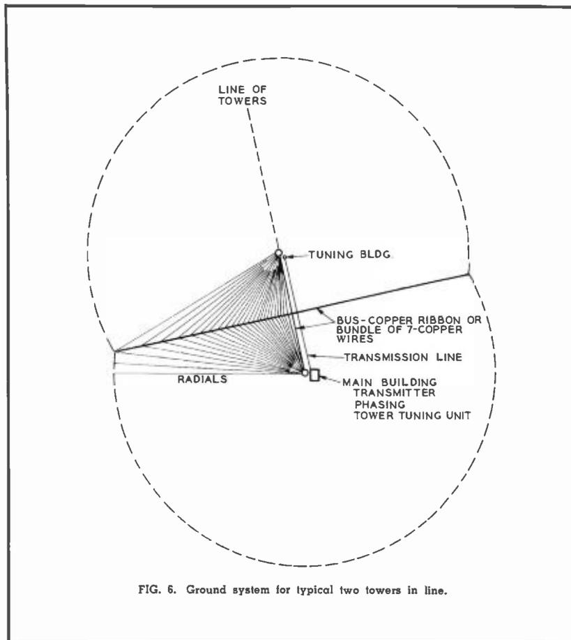
FIG. 6. Ground system for typical two towers in line.
