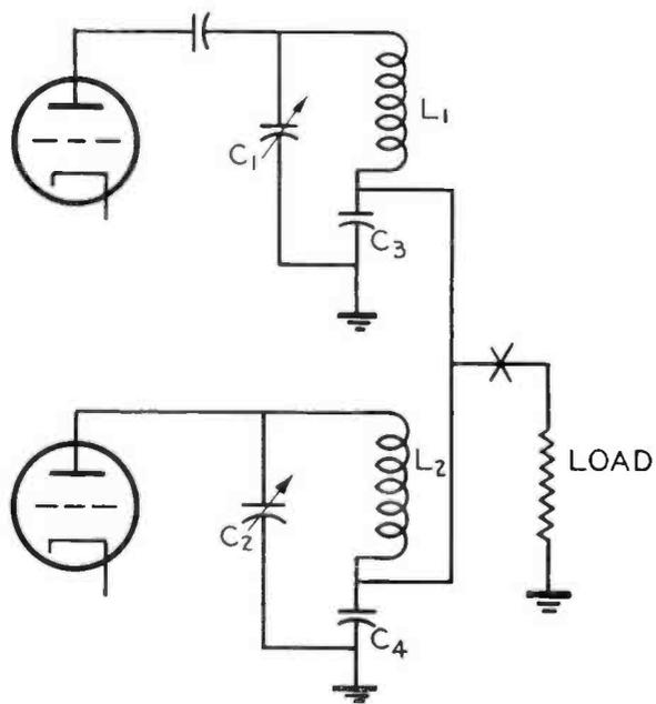
FIG. 10. Simplified circuit of PA output. Note that phase variation of PA input produces change in output load currents.
