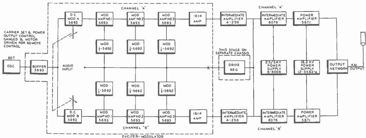
FIG. 2. Basic circuits of RCA Ampliphase Transmitter.
