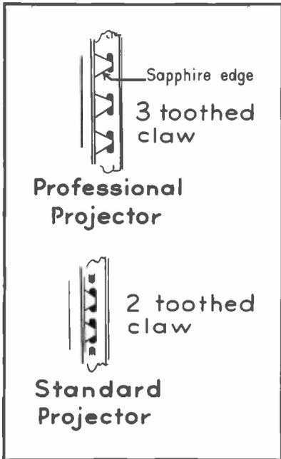
FIG. 2. Comparison of three-tooth vs. two-tooth claw pull-down.
