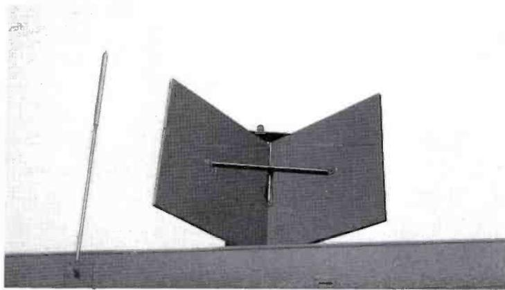
FIG. 4. Close-up of coax and corner reflector antennas atop mobile unit. These are used for 450 mc transmission to WHHM studios.
