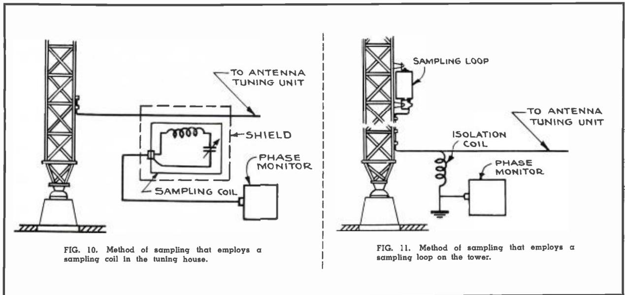
FIG. 10. Method of sampling that employs a sampling coil in the tuning house.
