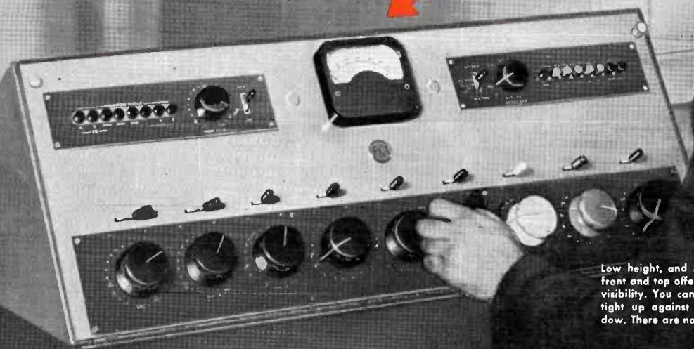
Low height, and 30-degree sloping front and top offer maximum studio visibility. You can install the BC-2B tight up against your studio window. There are no rear connections.
