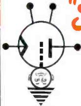
Stands on its head, electrically speaking, because its grid-flange construction permits grounded-grid operation with effective isolation of input and output circuits. Benefits: simplified circuitry, lower lead inductance, and more stable operation.
