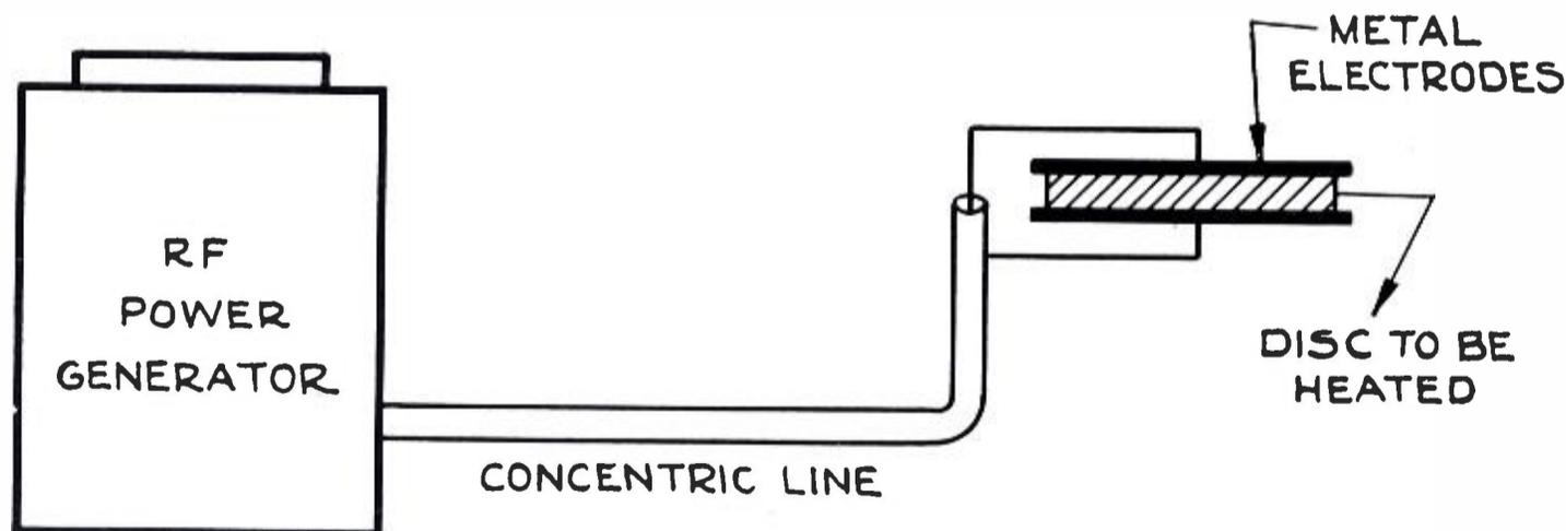
4. RCA engineers have added a final touch to this molding procedure by using radio frequency power as the means of pre-heating the thermoplastic disks. R-F current from an 8 Mc oscillator is caused to flow through the disk to be heated as shown
