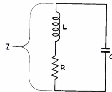
FIG. 6. Basic shunt peaked network.
