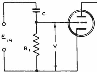
FIG. 3. Grid coupling network.
