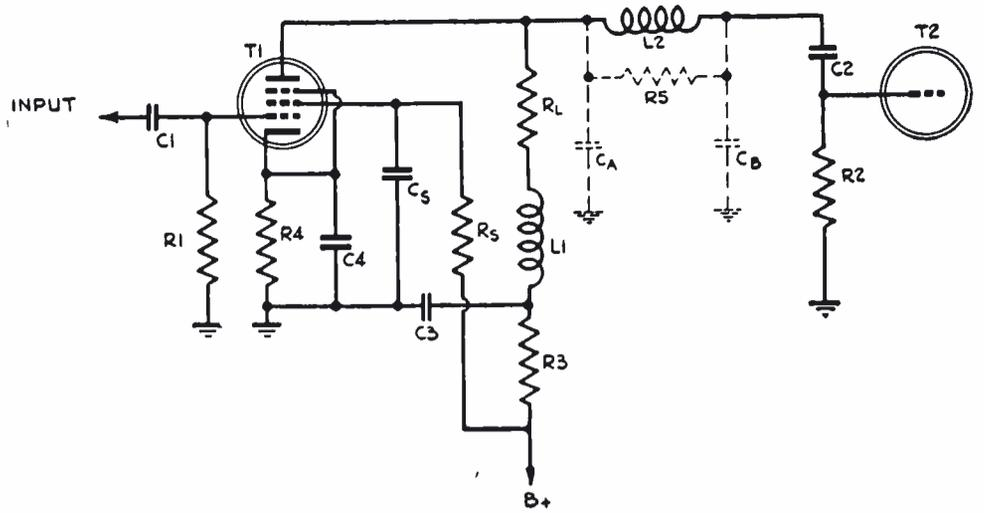
To compensate for  $R_1-C_1$  or  $R_2-C_2$
