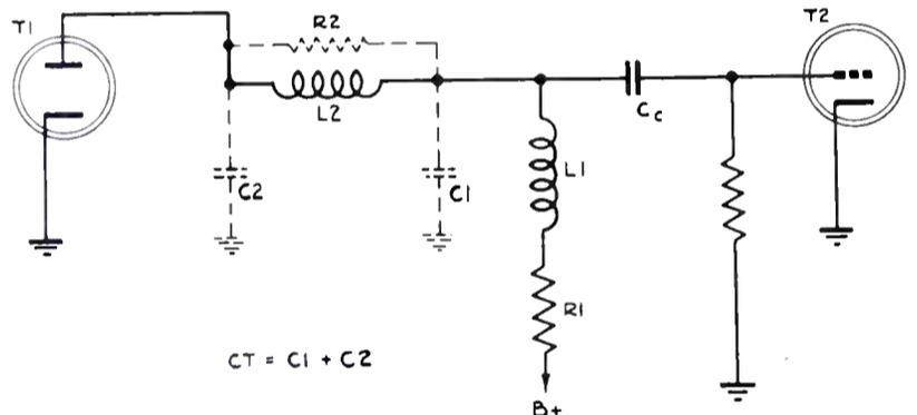
FIG. 11. Combination peaking stage.
