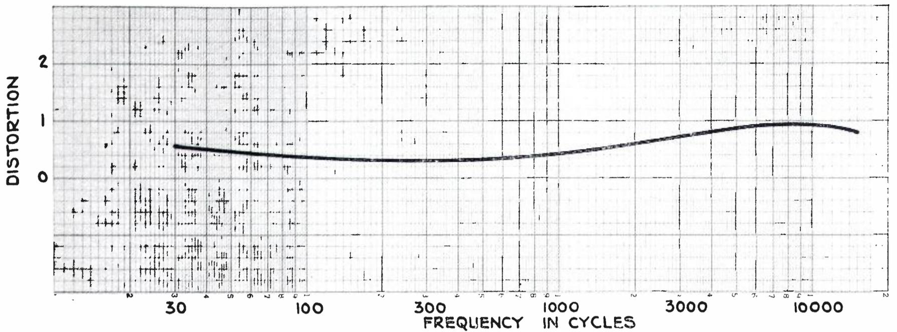
FIG. 5. Typical distortion versus frequency curve for an FM transmitting system. A curve of this type must be filed in answer to Par. 6(d) of Form No. 320.
