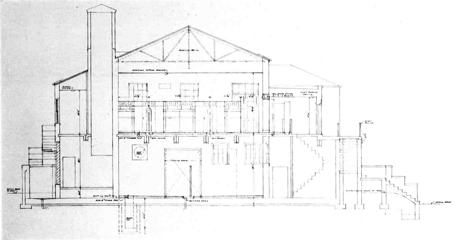
FIG. 1. Longitudinal section of transmitter building, located at Wayne, N. J., which houses OWI-CBS International shortwave stations WOOC and WOOW.
