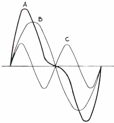
FIG. 13. Complex wave with components in phase.
