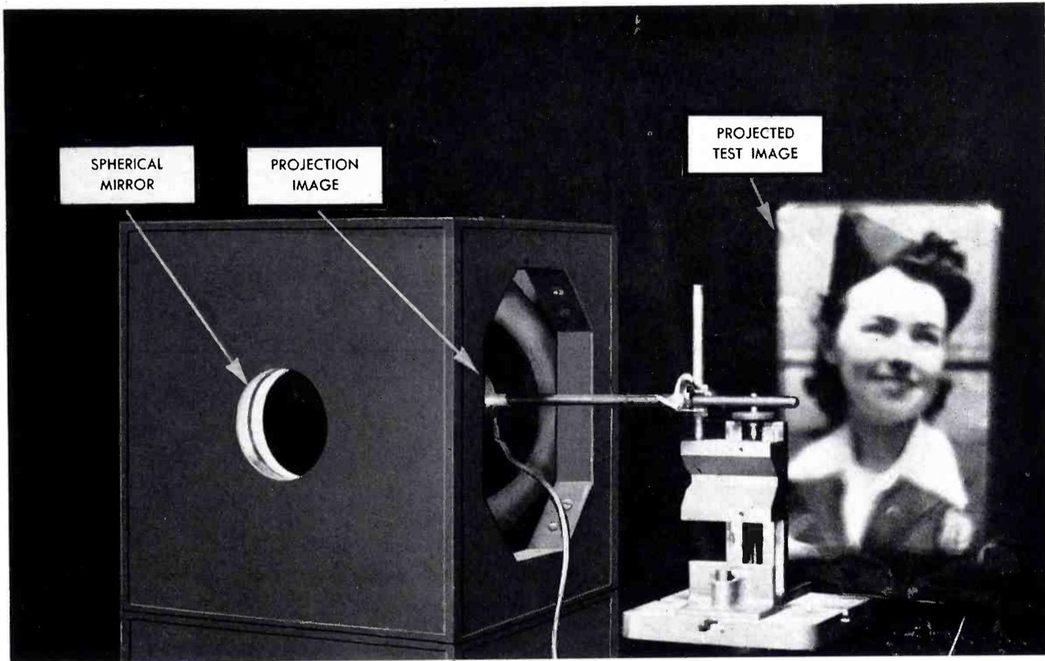
1. This is a temporary test setup used to check the molded correcting lenses before they are mounted in a receiver. The box in the foreground contains a standard spherical mirror mounted on the inner surface of the near side. At the proper focal point is an illuminated image simulating the face of the projection tube. In this view, no correcting lens is in place, hence the projected picture is very fuzzy.
