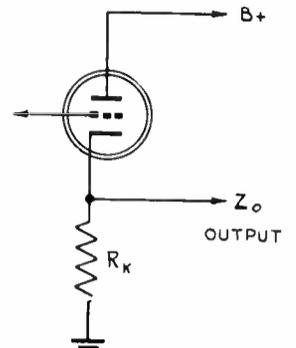
FIG. 15. Pentode cathode follower. FIG. 16. Triode cathode follower.
