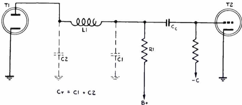
FIG. 9. Series peaking stage.
