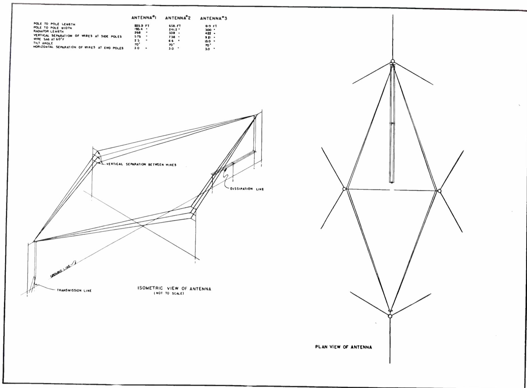
**FIG. 6.** Illustration of multiple-wire rhombic antennas employed at Wayne plant. Three different sizes are in use, their dimensions being determined by design frequencies of 9.6 Mc, 11.8 Mc and 15.3 Mc. These are connected as terminated rhombics and each can be operated over a relatively wide band of frequencies providing antenna facilities for the International frequency range of 6 to 21 megacycles.
