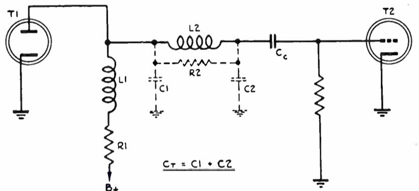
FIG. 10. Combination peaking stage.
