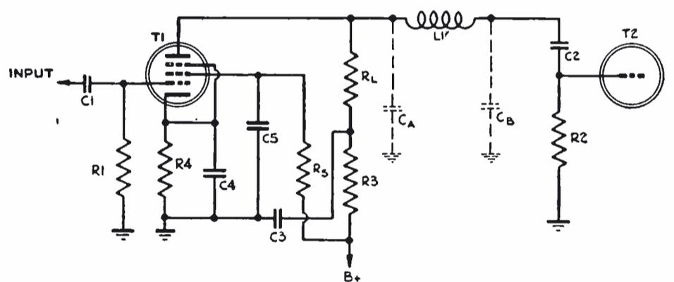
To compensate for  $R_1-C_1$  or  $R_2-C_2$
