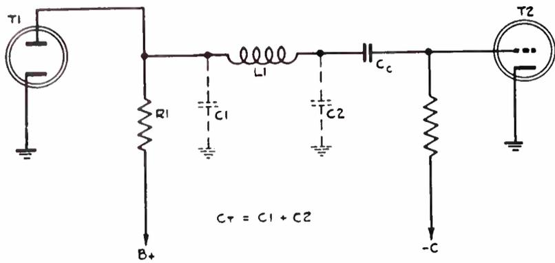
FIG. 8. Series peaking stage.
