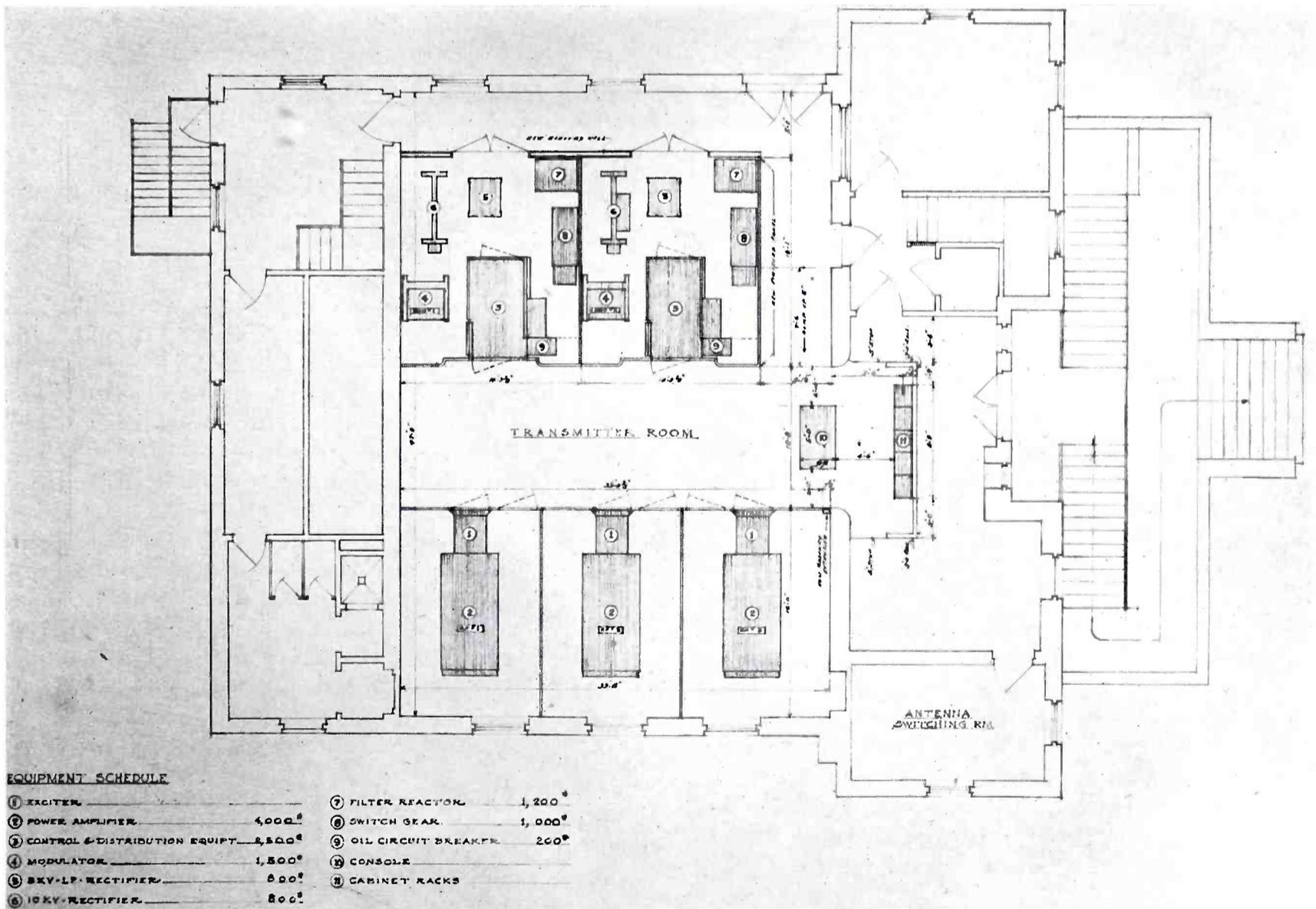
FIG. 2. Floor plan of OWI-CBS plant showing general placement of the two RCA 50 KW shortwave transmitters. Three complete r-f channels are mounted adjacent to one another on one side of the transmitter room and two complete modulator-power supply units are on the opposite side.
