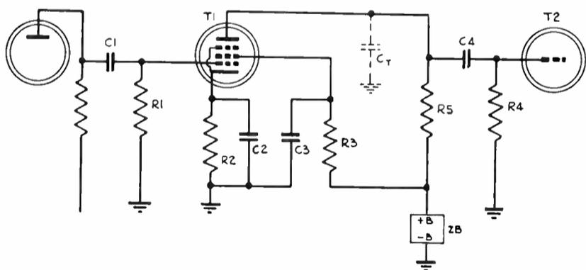
FIG. 1. Conventional R-C coupled amplifier stage.
