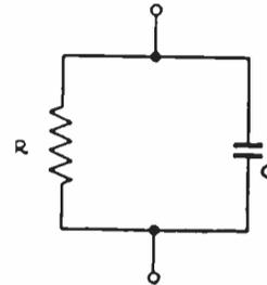
FIG. 4. Equivalent cathode or plate load network.
