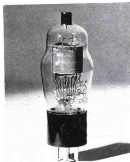
Figure 5. The shield grid tube.
