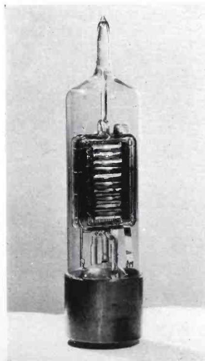
Figure 6. Tube used in first Trans-Atlantic broadcast—1915.
