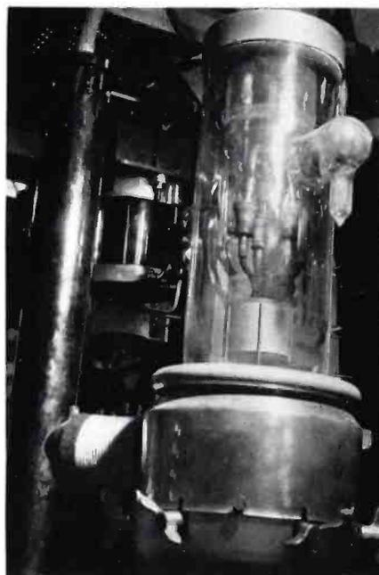
A closeup of a 100 KW tube used in the 50 KW transmitter.
