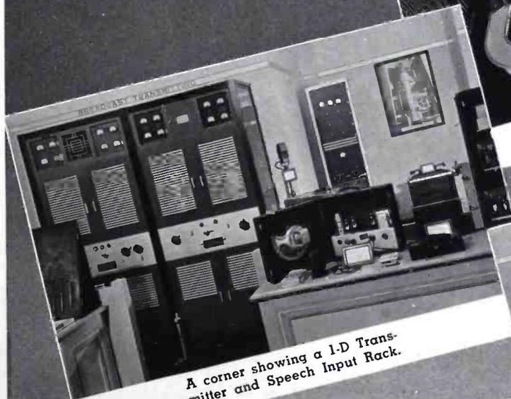
A corner showing a 1-D Transmitter and Speech Input Rack.
