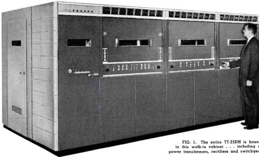
FIG. 1. The entire TT-25DH is housed in this walk-in cabinet . . . including all power transformers, rectifiers and switchgear.
