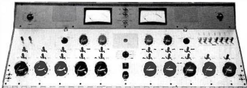
FIG. 3. Front view of consolette showing "human engineered" arrangement of controls.
