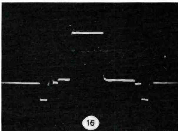
This slide (No. 16) shows the video round robin under average circumstances. The streaking as shown by the rounding of the corners can be more easily seen and photographed if the CRO is set on the 1RE roll-off position. Note that the top left corner of the window is almost square but that there is some rounding of the bottom right corner. This is considered to be the present state of the art.
