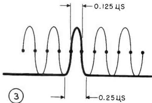
Although a sine-squared pulse could be produced this way, it is not practical from a design standpoint. Actually, it is produced by using a very narrow pulse which is widened and shaped by filters. Thus, one pulse and three sets of filters provide the  $\frac{1}{4}$ ,  $\frac{1}{8}$ ,  $\frac{1}{16}$  microsecond pulses.
