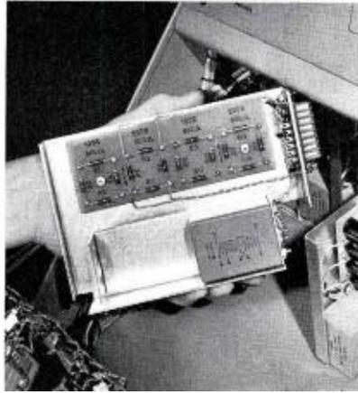
FIG. 20. High level isolation unit.
