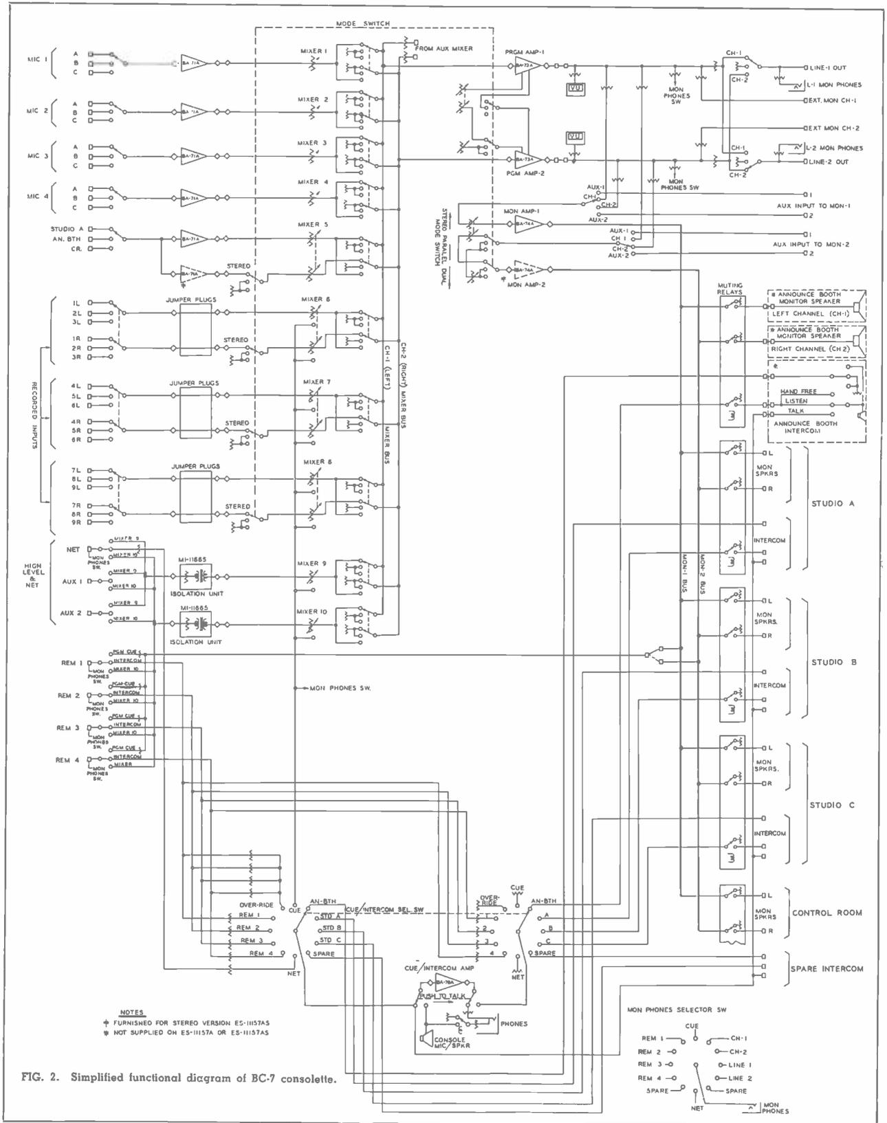
Two output program line keys are provided. Each program line input has a three position selector switch to provide selection of signal from either program amplifier. The center (or "OFF") position, terminates the line.
