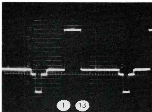
Thus, overshoots do not normally leave the control room. Since there is no energy in the edges of the window signal above 4.0 mc, any appreciable ringing occurring at the top left corner means there is in-band trouble and should be reported.
