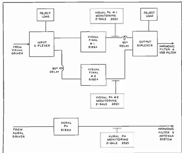
FIG. 12. Block diagram of the power-amplifier portion of the transmitter. Diplexed amplifiers increase transmitter reliability and better overall transmitter performance.
