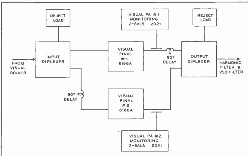
FIG. 7. Block diagram of the visual finals in the TT-25DH transmitter. Diplexing improves the reliability of the transmitter.
