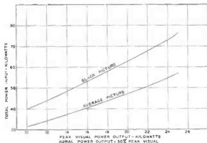
FIG. 3. Input-vs.-output power curve for the TT-25DH transmitter. Note that, at full power with an average-brightness picture, the TT-25DH draws only 60 kw of primary power.
