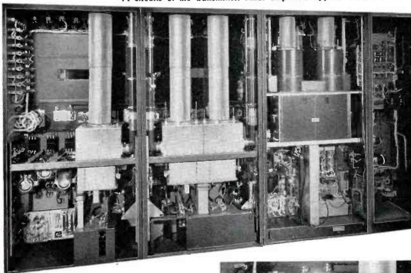
have to be replaced. This feature helps reduce operating costs and also reduces the possibility of lost air time. High-voltage transformer failures have resulted from mercury-vapor tube faults. This type of transformer failure is eliminated by the use of silicon diodes.
