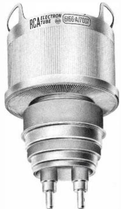
FIG. 8. The Type 6166A ceramic tetrode. The TT-25DH uses three (one aural; two visual) of this tube type as power amplifiers. The aural operates Class "C", the visual, Class "B".
