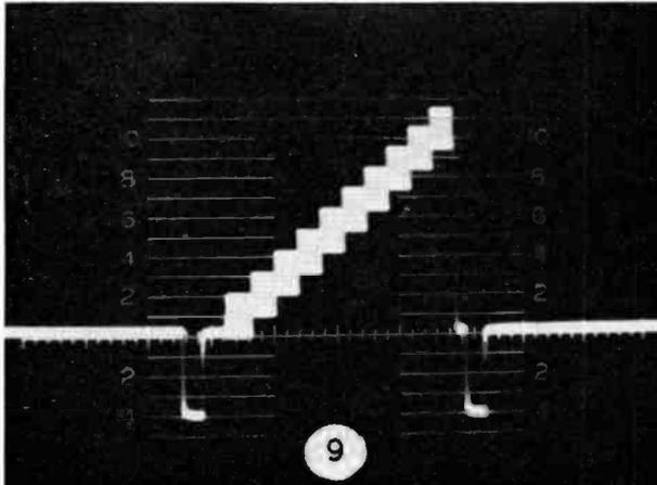
The actual stairs start late in this signal so the 3.5 mc sinewaves can start at the blanking level and still not interfere with the backporch burst during color shows (Slide No. 10).
