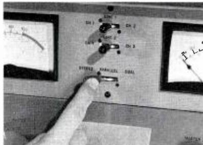
FIG. 11. Line-out and mode selector switches.
