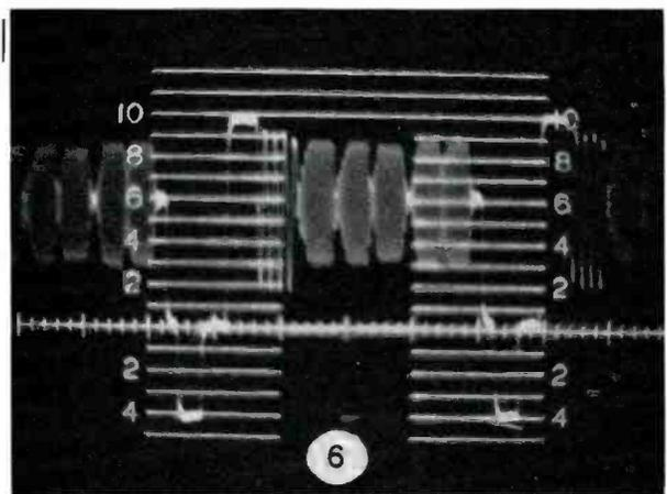
A condition which is not acceptable is shown by slide (No. 6). Although the high-frequency response as shown here is relatively flat, the level of the white bar indicates that there is a mismatch between the low frequencies and high frequencies. Another unacceptable condition is shown by this slide (No. 7) which illustrates an hour-glass response. There are two main objections to this type of response: (1) it accentuates ringing, and (2) it "softens" the monochrome rendition of color receivers.
