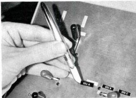
FIG. 5. Pressure sensitive metallic labels are supplied so that panel designations can be tailored to individual needs.
