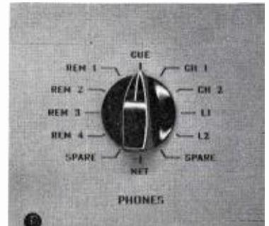
FIG. 12. Monitor phones selector switch.
