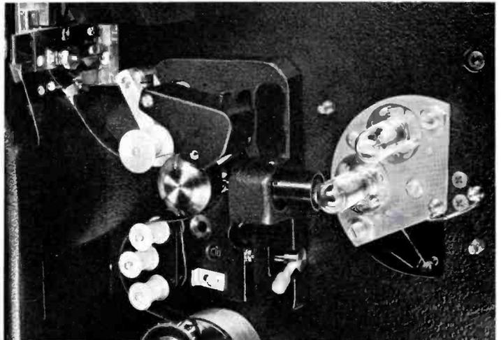
This is a solenoid operated device, which upon sensing that loop loss has occurred applies a force to the film that causes film slippage to occur at the gate between pull-downs. When sufficient film has been recovered from the top loop to establish optimum lower loop size, a second sensing switch de-energizes the solenoid, and the loop restorer arm is free to return to its normal position. Sufficient compliance has been provided to avoid any possible damage to the film during claw engagement.
