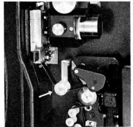
FIG. 7. Automatic exciter-lamp-changer, operating within one second, contributes to the high reliability of the TP-66 Projector.
