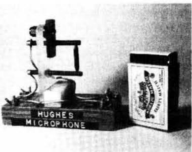
**Fig. 2.4: Replica of the original microphone invented by Professor Hughes (circa 1850)**
