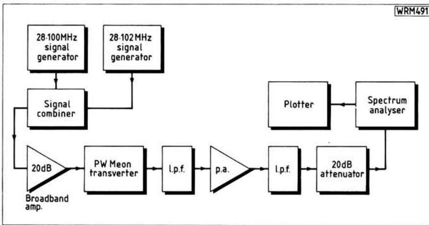
Fig. 7: Arrangement used for i.m.d. measurements
