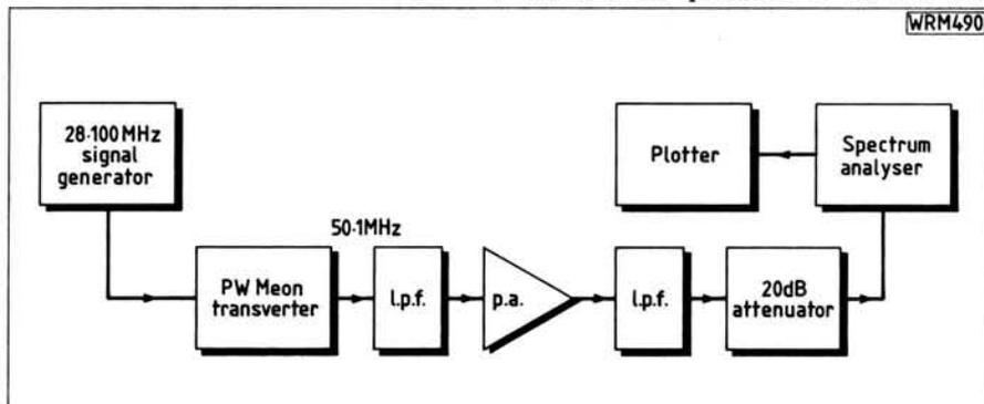
Fig. 5: Equipment set-up for spectral performance checks
