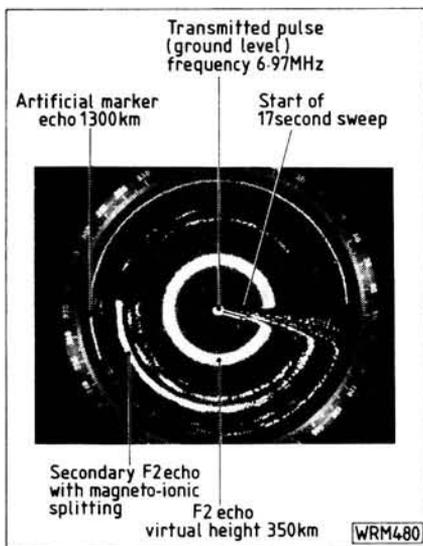
**Fig. 1.3: Strong F layer echo with secondary echoes and magneto-ionic splitting. Critical frequency 6.97MHz. The display shows an F2 complex with Fo and Fx secondary echoes. Recorded June 1983. Note the constant amplitude of the F2 primary echo**
