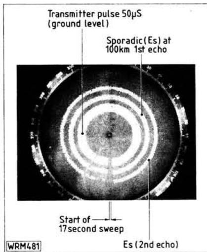
**Fig. 1.4: Sporadic-E (Es). A good example of Sporadic-E with primary and secondary echoes. Recorded June 1983. Note the constant amplitude of the primary Sporadic-E. Similar Es clouds were observed during the summer of 1984, up to the end of August of that year and frequently lasting for periods of up to one hour**
