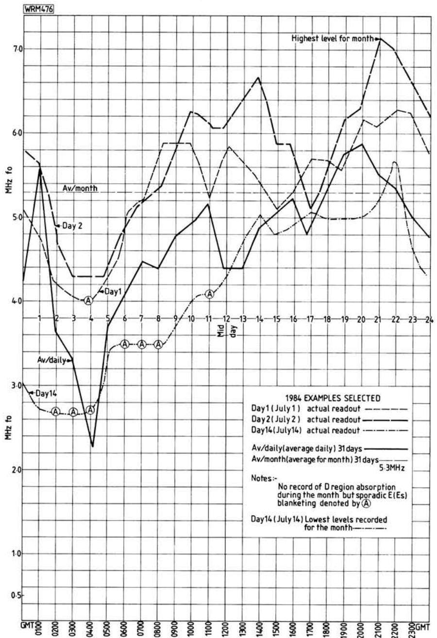
**Fig. 1.6: Plots of critical frequencies for 24 hours on selected days during July 1984. Annotations in panel on diagram and in text provide further information. Note: No "D" region absorption (due to s.i.d.) observed during the month. During the higher levels of sunspots, critical frequencies have regularly been above 7MHz**
