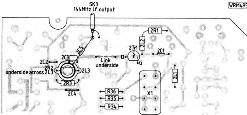
**Fig. 2: Revised component location. 2L3 is tapped at 2 turns from the top**
