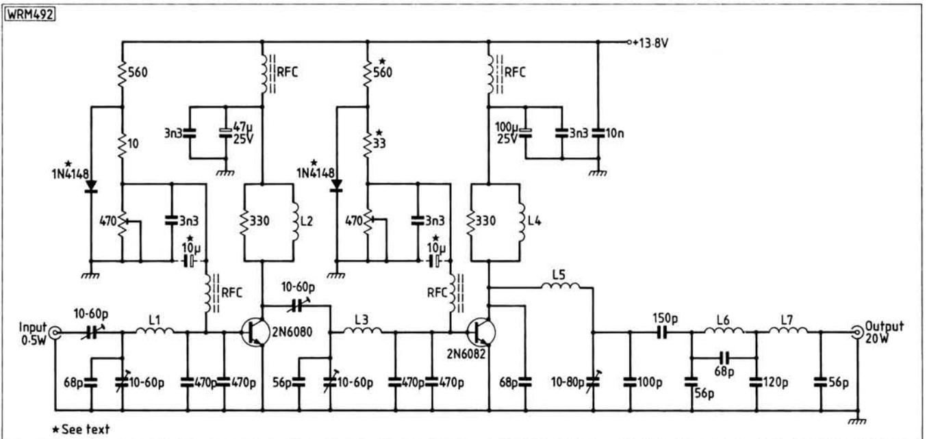
**Fig. 3: Circuit diagram of the Spectrum TA6U2 p.a.**
