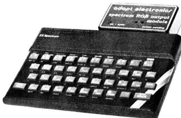
monitor socket so that leads are readily available to couple to any RGB monitor.
