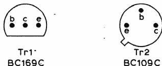
Fig. 5: Transistor base connections.
