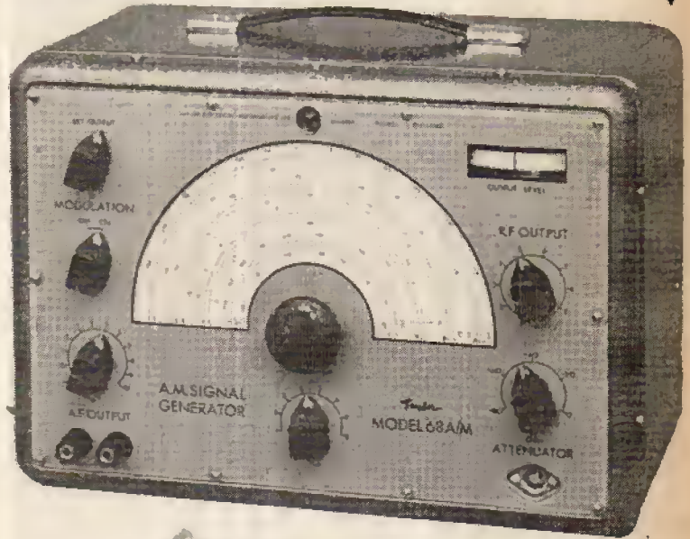
Fig. 16: The still popular Taylor Model 68A/M signal generator. Frequency range is from 100kHz to 240MHz (all on fundamentals) over 8 ranges. Although a.m. only, the instrument is suitable for the alignment of ratio detectors and f.m. r.f. and i.f. stages. A variable 400Hz audio output is available and an r.f. monitoring meter allows accurate setting of the signal applied to the attenuators.
