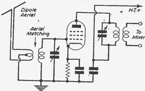
Fig. 12.—The functional circuit of a V.H.F. amplifier stage.
