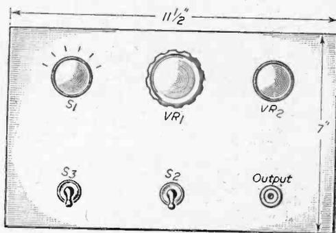
Fig. 3.—Layout of panel.
