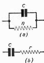
Fig. 13 (a) and (b).—These two circuits are actually identical.
