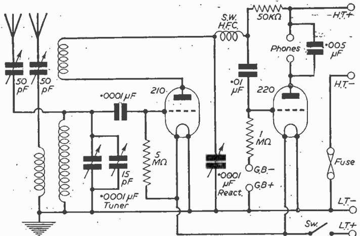
Fig. 1.—Theoretical circuit of a simple two-valve receiver.
