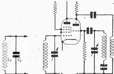
Fig. 2.—The test circuit and a typical frequency-changer stage.
