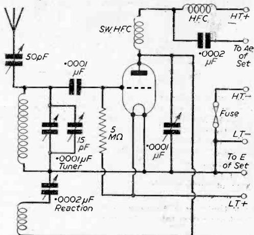
Fig. 2.—Simple one-valve converter.
