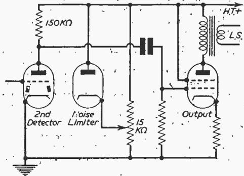
Fig. 2.—Simple clipper circuit.
