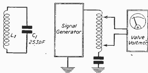
Figs. 3 and 4.—The test circuit and method of using a signal generator.
