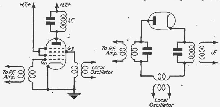
Fig. 13.—Two types of mixer circuits for obtaining the heterodyne beat between two frequencies.
