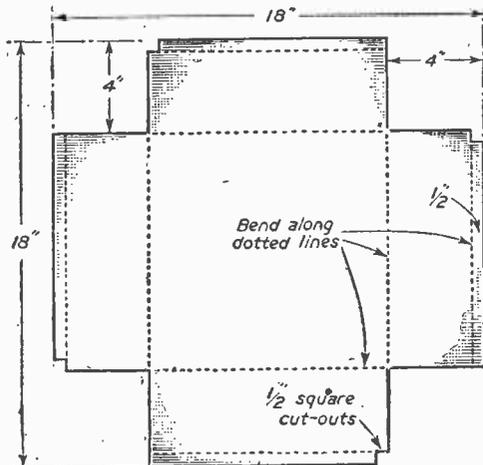
Fig. 2.—Details of the chassis.
