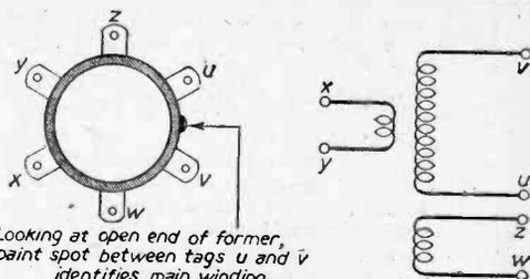
Looking at open end of former, paint spot between tags u and v identifies main winding. (w and z on 'Green' coils)
