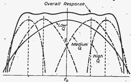
Fig. 15.—The combined effect of a number of stagger-tuned circuits.
