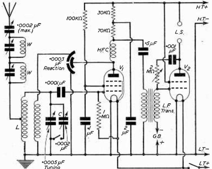
Fig. 1.—Theoretical Circuit. Note the wavetraps W, the coil L, and the condenser C which extends the waverange.
