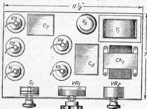
Fig. 2.—Layout of chassis.
