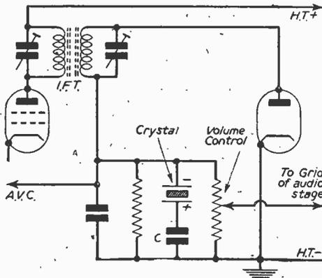
Fig. 3.—In this shunt circuit a crystal diode is used.
