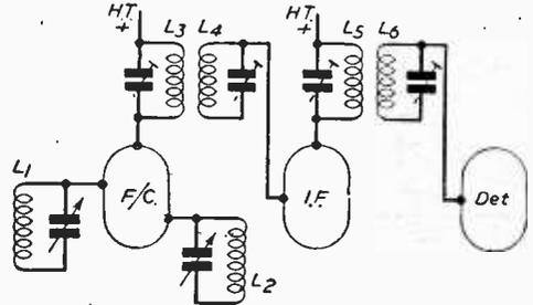
Fig. 3.—Simplified diagram of the tuning found in a circuit of the Fig. 2 type.
