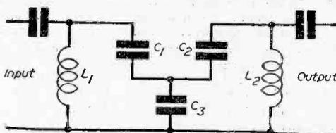
Fig. 16.—An I.F. transformer using mutual capacitance instead of mutual inductance coupling. The high frequency hump is tuned by means of C1 and C2 while the low frequency hump by means of C3.
