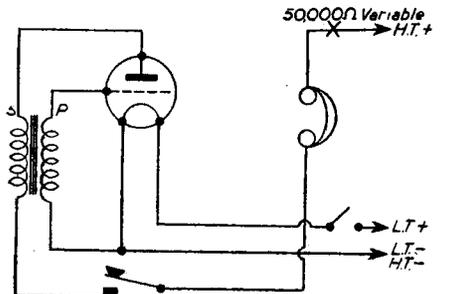
Fig. 2.—If preferred an audio-frequency oscillator, with the circuit shown here, may be used for practice purposes.
