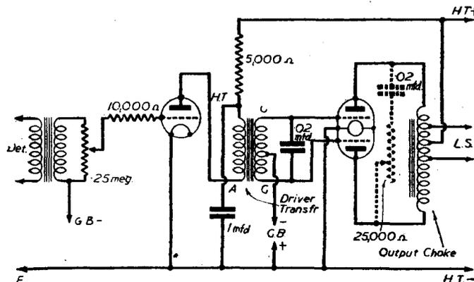
There is also an optional tone-correction circuit between the two anodes, as used in Q.P.P.
