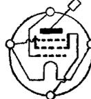
Fig. 3.—To improve matters, an additional grid was added to the tetrode, thus providing us with the pentode.
