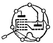
Fig. 5.—Another electrode assembly known as a triode hexode. This is superior to the heptode.
