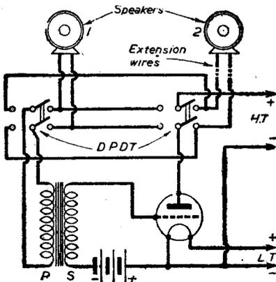
Circuit diagram for a novel house telephone system.
