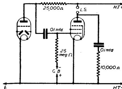
Fig. 3.—Skeleton circuit of an R.C.C. stage following a double-diode-triode. Fixed tone compensation is shown, and the connections given are for battery bias. Auto-bias may generally be used, as in Fig. 2.
