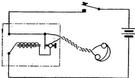
Fig. 1.—An excellent morse practice set using a good high-rate buzzer in conjunction with a morse key and a pair of 'phones.
