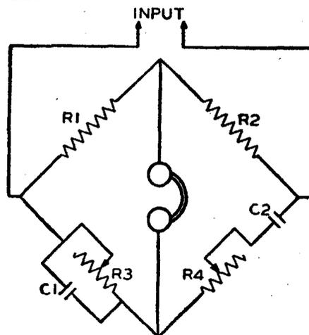
Fig. 3.—Wien's bridge circuit on which the instrument is based. C1, C2—.0133 mfd. mica (made from the following). .01 mfd., .003 mfd., .0003 mfd. All 2% tolerance. R1—2,000 ohms, 1 w. R2—1,000 ohms, linear taper. R3—1,000 ohms, 1 w. R4, R5—Dual 500,000 ohm pot.
