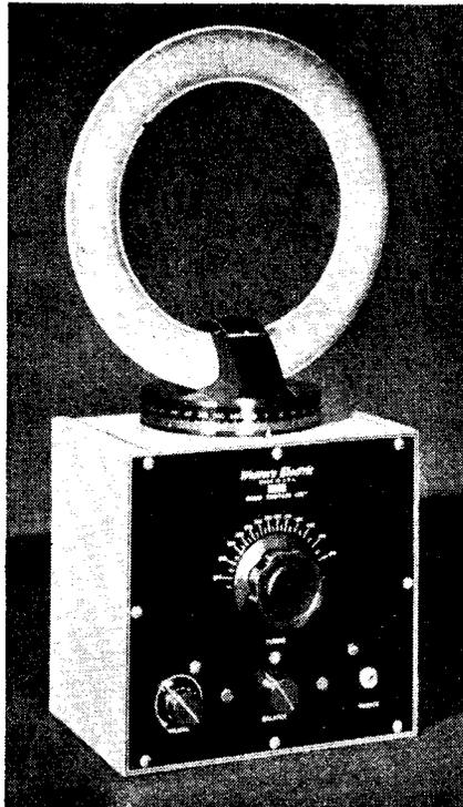
The radio compass unit made by Western Electric.
