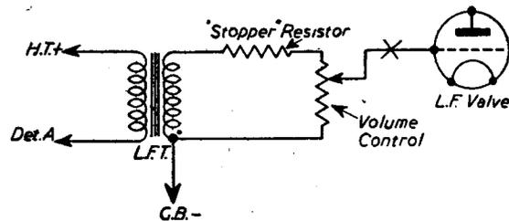
Fig. 1.—A high-resistance "stopper" resistor in the position shown will cut down the maximum volume to a marked degree, due to its being in series with the element of the volume-control potentiometer.
