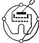
Fig. 2.—By adding another grid (screen) the tetrode or screen-grid valve is formed.
