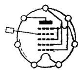
Fig. 4.—This shows how the pentagrid or heptode is formed. This type of valve is primarily intended for frequency-changing in a superhet.
