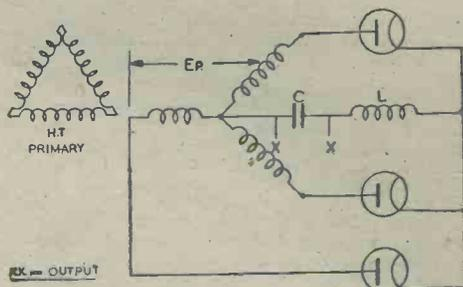
Fig. 5.—Three-phase half-wave rectification.
