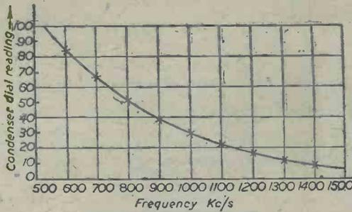
Fig. 6.—Condenser calibration.
