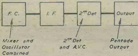
Fig. 1.—Unit sequence of commercial receiver.
