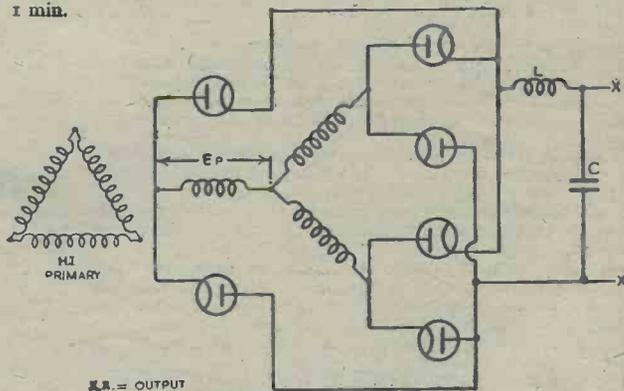
Fig. 6.—Three-phase full-wave rectification.
