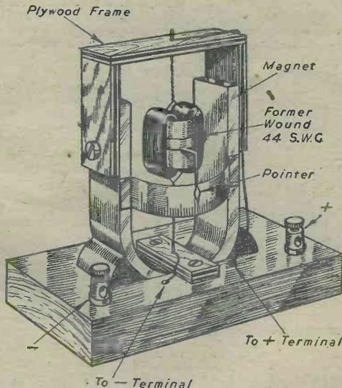
A simple moving-coil Galvanometer.
