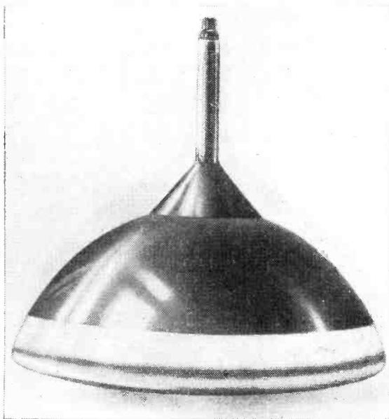
*The short-necked, large-faced flat tube which has been developed successfully abroad.*
