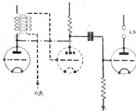
Fig. 2.—A transformer-coupled L.F. stage and arrangements for cutting it out.
