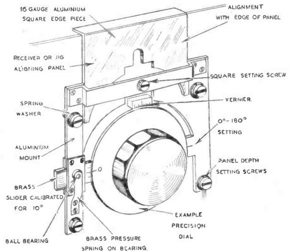
A novel jig for calibrating and checking dials.
