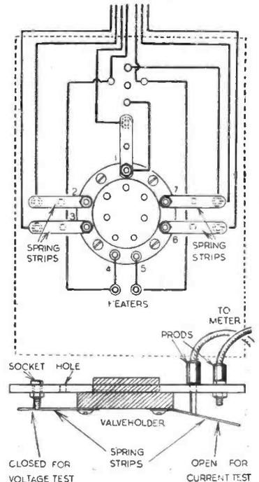
Rear view of the valve adapter showing wiring connections.
