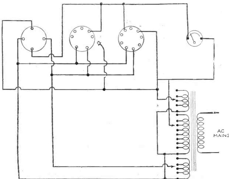
Fig. 2.—Basis of the modern commercial all-valve tester.
