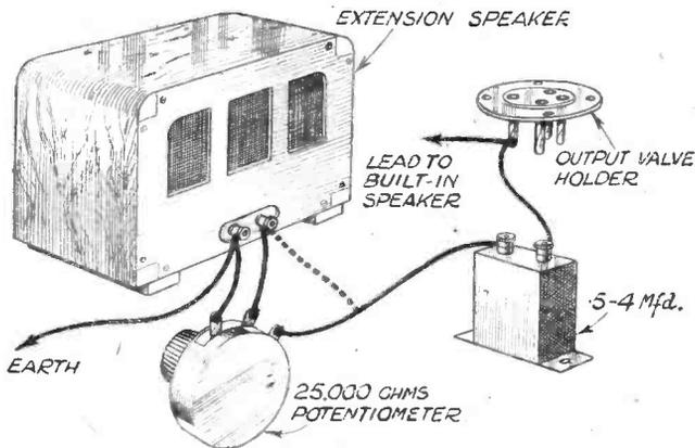
Fig. 1.—Simple connections for an extension speaker with remote volume control. This can be omitted by using the connection shown by a broken line.
