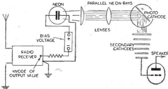
A pictorial illustration and theoretical circuit of a light-sensitive set-up which was exhibited on Stand No. 18, and which included the new electron multiplier described in these pages last week. The small diagram shows the general principles upon which the electron multiplier operates, and in the example a photo-electric cathode is indicated.
