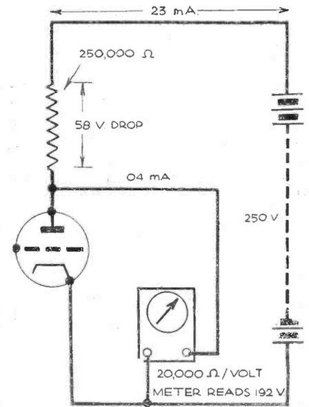
Fig. 5.—A very high-resistance voltmeter gives practically correct readings as shown here.
