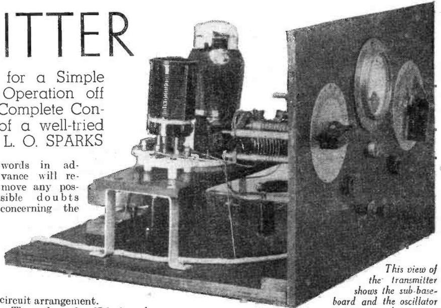
This view of the transmitter shows the sub-baseboard and the oscillator coil.
