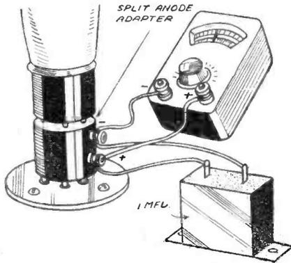
The simplest way of testing a valve by means of a "split leg" adapter.
