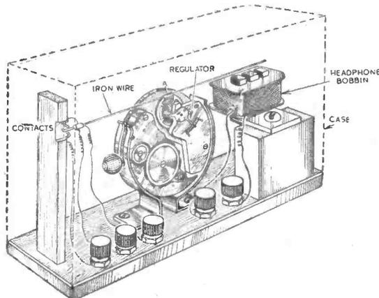
For constructing this sensitive relay the works of an old wrist-watch were utilised.
