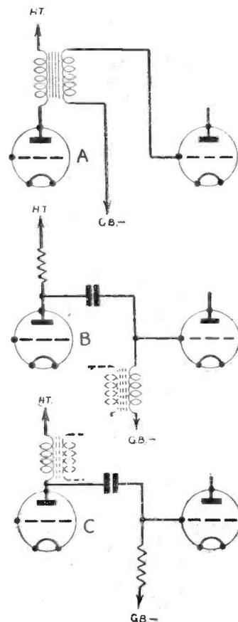
Fig. 3.—Using a faulty L.F. transformer, showing the two methods of connection at B and C.
