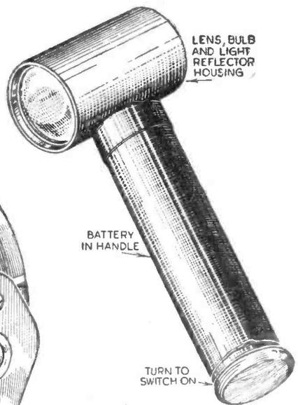
An ideal accessory for the serviceman, this magnifier incorporates a powerful light source. The magnification is approximately 20 diameters and the handle houses the battery. This is a Servisol product, and the length is 7 in. The handle is 1 1/2 in. diameter and the price is 15s. 6d.
