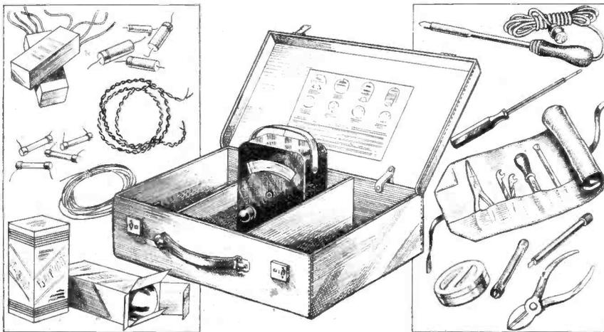
A suitably fitted-out attaché case, with good multi-range meter, small tools and a few spares, is essential to the successful service man.
