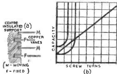
An air-dielectric trimmer of novel design produced by T.C.C. By means of an ingenious threaded device the action of rotating the screw results in successive interleaving of the vanes somewhat in concertina fashion. The graph shows the capacity variation plotted against screw turns. High smoothing properties, with compact size, are the main features of this neat electrolytic condenser. These Midgets are produced by T.C.C.
