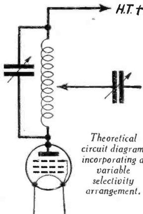
selective. After some experiments I replaced the fixed coupling condenser by a small semi-variable baseboard mounting component with a maximum capacity of 56 mmfd. I then made the anode coil of bare wire on a grooved former, and by adjusting the tapping point on the coil I found that I could vary the degree of selectivity, although, of course, signal strength was also affected. The accompanying theoretical diagram shows the final arrangement.—W. LANE (N.W.5)
