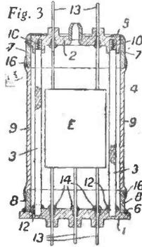
recesses in the other disc 2 with the interposition of springs 10.
