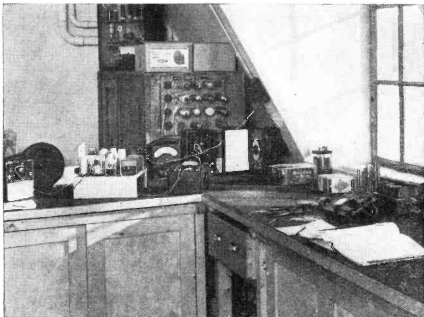
A corner of the PRACTICAL WIRELESS laboratory. Benches are well lighted, a rack is fitted for all types of valves and the meters are carefully stored in cupboards. The large speaker baffle, test amplifiers and power units are not shown in this picture.
