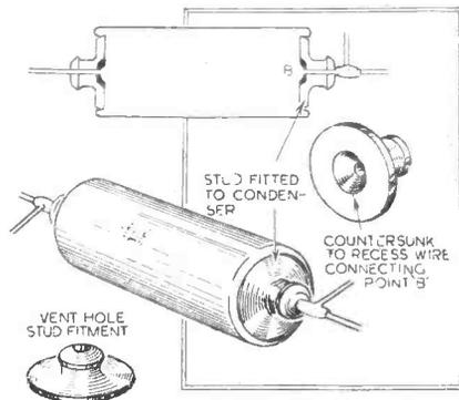
A simple method of protecting tubular condensers.
