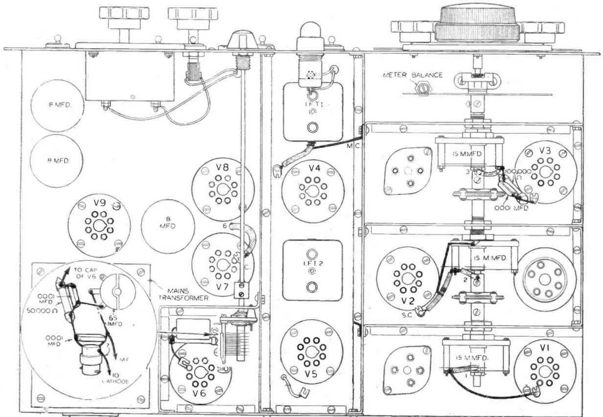
*Above chassis view of the "Air-Hawk" 9. The B.F.O. unit wiring is shown separately, on the mains transformer, for clarity.*
