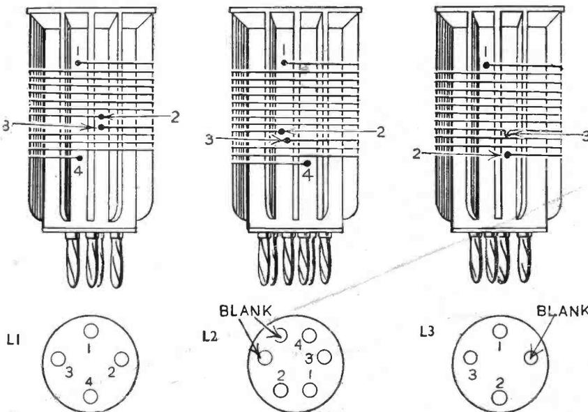
The above illustrations show the three coils needed for each waveband, with the connections to the pins. The lower illustrations show the pins, viewed from below the coils—that is, the under-chassis view of the coilholders. For the three smallest coils threaded formers should be used, and for the remainder plain formers are required. Note that all windings are in the same direction.
