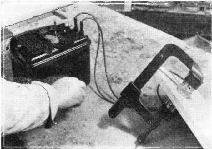
Fig. 5.—Every G.E.C. component that is mechanically operated undergoes a stringent test in which it is manipulated several thousand times.
