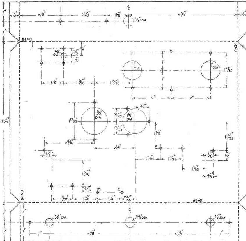
Drilling diagram for the chassis
