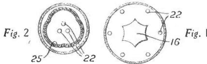
may be interposed between the cathode and anodes; the latter may be independently connected to circuit elements or connected together. The anodes 22, Fig. 2, may be arranged inside the cathode, which as shown has three curved emitting surfaces 25.
