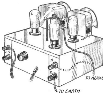
Fig. 7.—The H.F. stage may be cut out by transferring the aerial lead as shown here.
