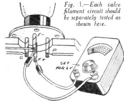
Fig. 1.—Each valve filament circuit should be separately tested as shown here.
