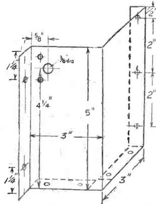
Fig. 7.—This is part of the B.F.O. screen. It is attached to the right-hand screen in Fig. 4, and at the rear to Fig. 8.
