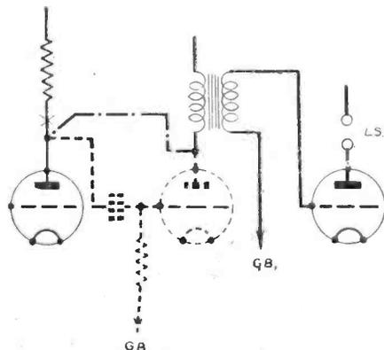
Fig. 1.—Cutting out an L.F. stage which is R.-C. coupled. The H.T. feed should be disconnected at the point marked "X."
