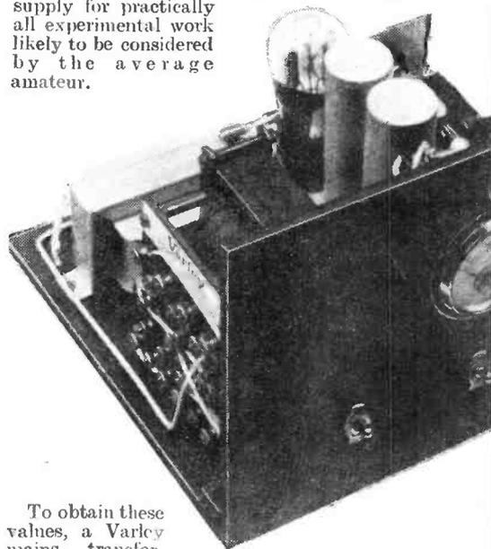
To obtain these values, a Varley mains transformer, Type E.P. 40, is used in conjunction with a Cossor rectifying valve of the indirectly-heated class, namely, their 431 U.
