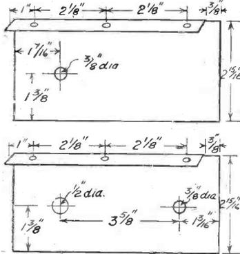
Fig. 3.—The above are two of the underside partitions separating the band-setters. The third partition is shown in Fig. 10. The upper unit is placed nearest the rear of chassis.
