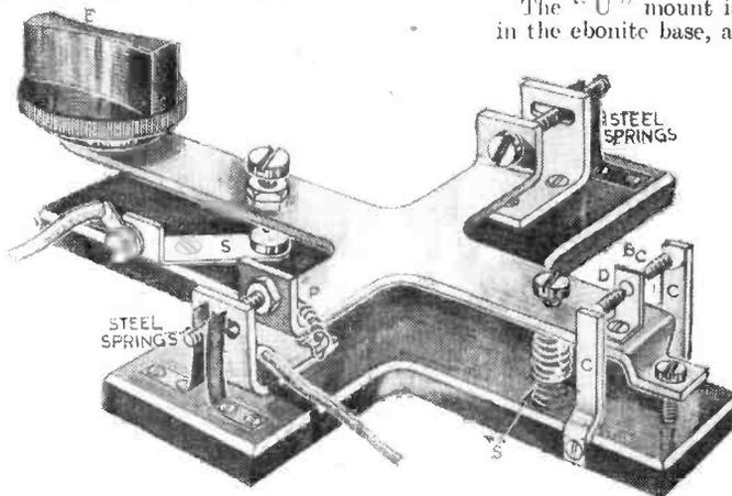
A pictorial sketch of the dual-action morse key, showing the details of construction.
