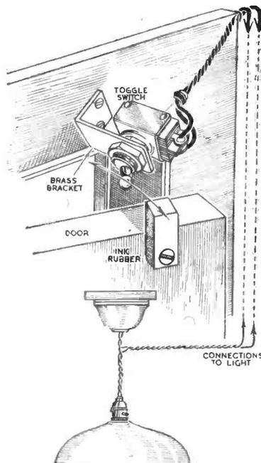
A handy dodge for operating a light switch by the the opening and closing of a door.
