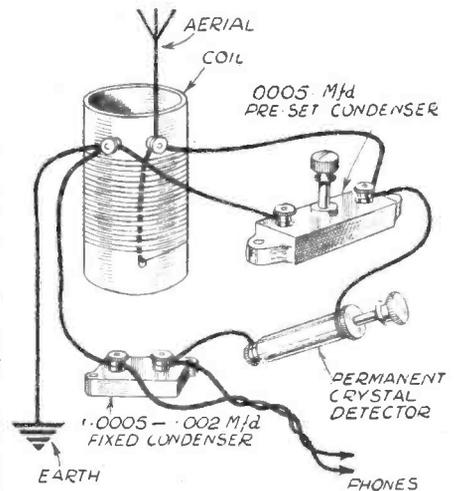
Fig. 2.—How a crystal receiver can easily be made. The coil can be of any type and only the medium-wave winding is used. If home made, use a 2-in. diameter former and wind on 50 turns of 24-gauge enamelled wire.
