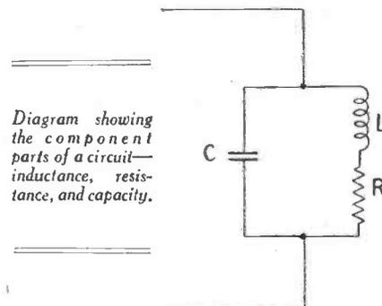
Diagram showing the component parts of a circuit—inductance, resistance, and capacity.
