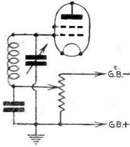
Fig. 1.—Controlling gain in a battery receiver may be accomplished by either of the methods above.
