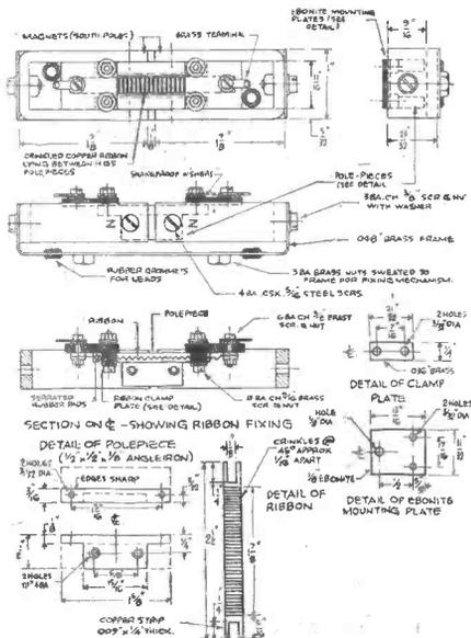
Constructional details of the mechanism for a ribbon microphone.
