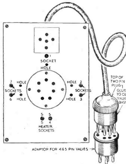
A simple valve adapter for voltage testing purposes.
