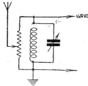
Fig. 3.—Controlling input by a resistance across the aerial circuit.
