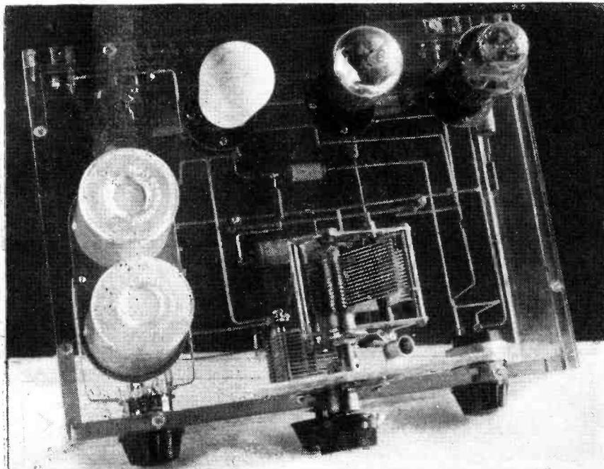
This view of the receiver shows clearly the layout of components on the transparent chassis.
