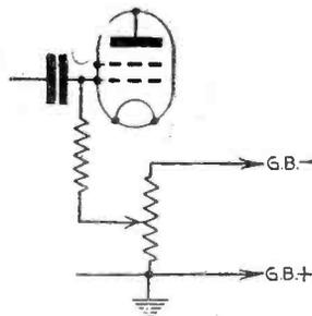
Fig. 2 (left)—Controlling a valve of the indirectly-heated type.
