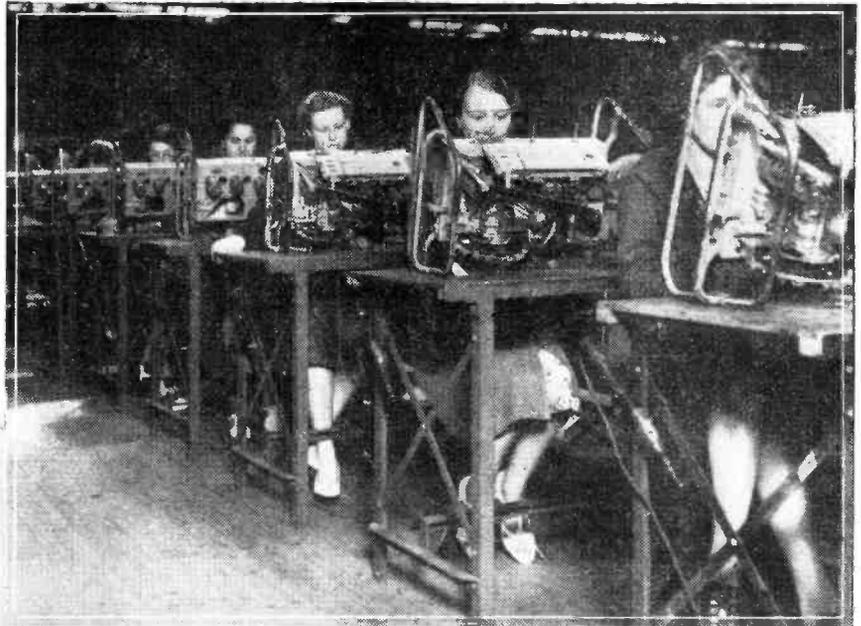
This novel view of production desks at Ekco Works shows new motor-controlled models nearly ready to leave their "cradles" for their cabinets. The cradles are clamped to the chassis at the start of the assembly process and remain until the end. Note the temporary pillars on the chassis, protecting the press-button units from damage before they are actually mounted in the cabinet.
