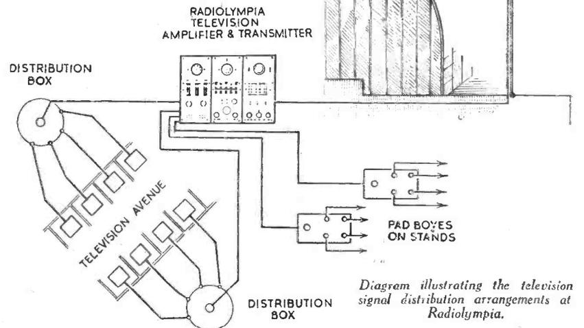
Diagram illustrating the television signal distribution arrangements at Radiolympia.
