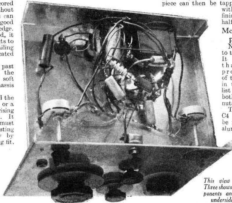
This view of the Trio-Pen Three shows the layout of components and wiring on the underside of the chassis.
