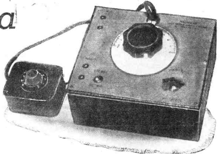
A Radiolab all-wave oscillator which can be used for testing down to 10 metres. The batteries are contained in the small case.
