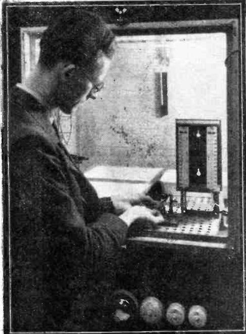
Fig. 1.—An insulation material testing cabinet installed by the G.E.C. for making sure that their sets function properly in foreign climes.
