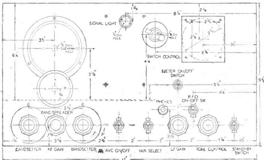
Fig. 2.—Panel layout and drilling dimensions.
