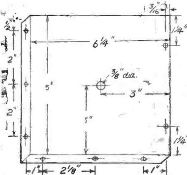
Fig. 6.—These are the supports for the band-spread condensers. Three of these have to be made, and all are identical. The central hole must be exact to enable the condensers to be mounted in line.
