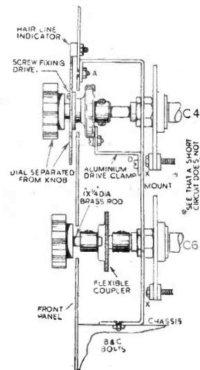
Fig. 4.—Side view of the aluminium brackets on which are mounted the condensers C4 and C6 and flexible coupling.
