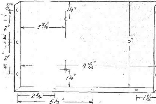
Fig. 4.—These are the two long partitions enclosing the I.F. and second detector stages. The unit on the right is bolted to the partitions separating the bandsread condensers. Note carefully the direction of the turned-up edges. The two-hole turn is attached subsequently to the panel.
