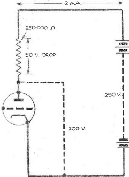
Fig. 3.—Circuit data of an R.C. stage, showing actual voltage and current readings.
