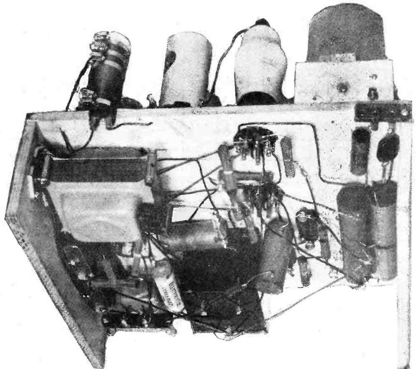
*Chassis construction simplifies wiring and enables a compact receiver to be made up, bulky components being accommodated beneath the chassis.*
