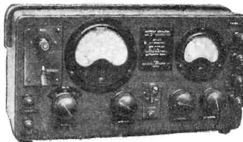
A G.E.C. valve-voltmeter for battery operation.
