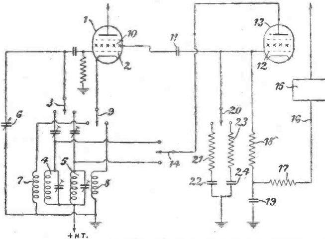
Fig. 1.—The modified circuit to which this article refers, the first valve being the local oscillator.
