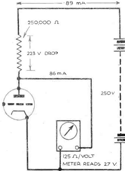
Fig. 4.—How a low-resistance voltmeter will give false readings from the circuit shown in Fig. 3.
