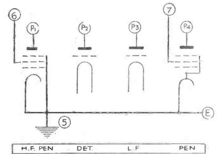
Fig. 2.—Circuit junctions for individual voltage measurements.
