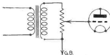
Fig. 6 (above)—A transformer is controlled as shown here, whilst on the right (Fig. 7) is a simple means of controlling speaker volume.
