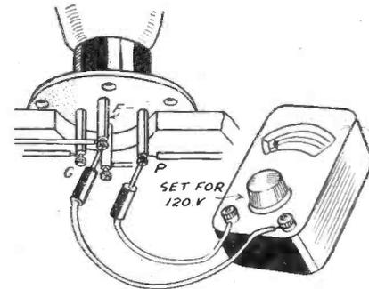
Fig. 6.—Test for H.T. at each anode with a high-resistance voltmeter.
