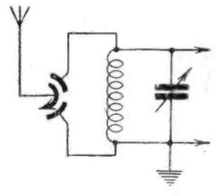
Fig. 4—Here the input is controlled by a differential condenser.
