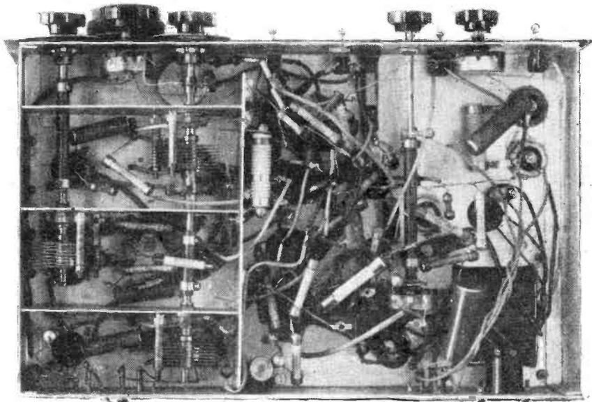
Fig. 1.—This view of the underside of the chassis shows the network of wiring and the screened tuning sections.
