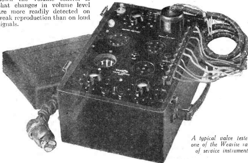
A typical valve tester—one of the Wearite range of service instruments.
