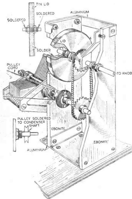
A part sectional view of a simple flywheel tuning movement.
