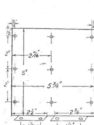
Fig. 8.—This section encloses the rear of the I.F. screens (Fig. 4) and is also attached to Fig. 7.
