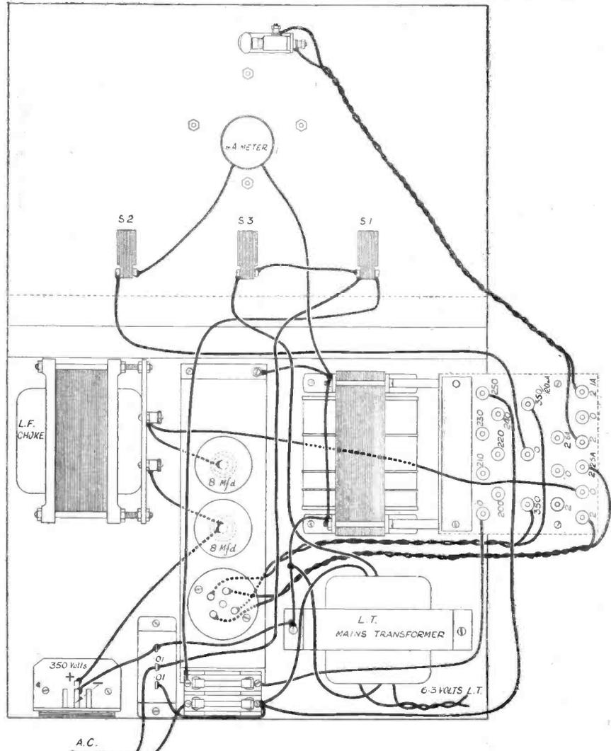
Fig. 4.—The fixed condenser .01—.01 mfd. across the mains is optional. If any hum is present, then it should be employed. The Varley E.P.40 has a different terminal panel than that shown.
