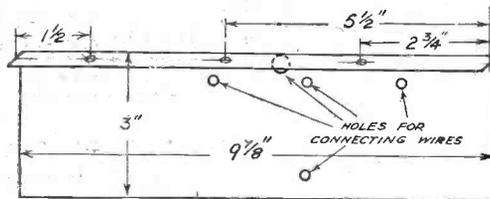
Fig. 5.—This partition is for the underside of the chassis and separates the band-setting condenser.
