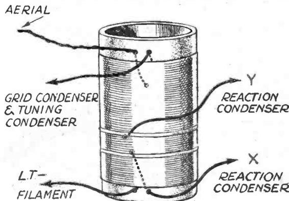
Fig. 3.—Coil connection details for the A.R.P. receiver.
