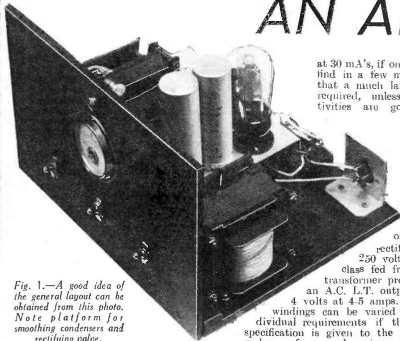
Fig. 1.—A good idea of the general layout can be obtained from this photo. Note platform for smoothing condensers and rectifying valve.
