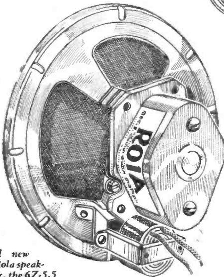
A new Rola speaker, the 6Z-5.5 P.M. This has a 4 1/2 in. cone and weighs 1 1/2 lb. It is an excellent model for portable or similar receivers where the space available is limited, the overall diameter being 6 1/2 in. and the overall depth 2 1/2 in. The speech coil has an impedance of 3 ohms and the price of the speaker is 16s.
