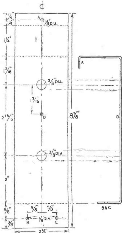
Fig. 5.—Drilling diagram and details of the aluminium bracket.
