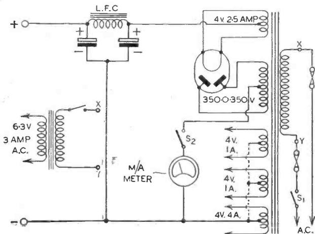
Fig. 2.—Theoretical circuit diagram of the All-Purpose A.C. Power Pack.
