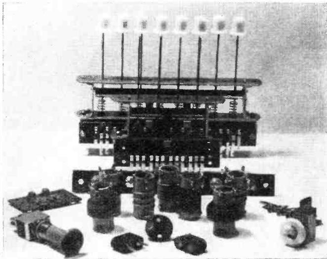
Above is one of the push-button tuning switch units including a new 4-way type. In the foreground are the new Unit coils which are available for straight or superhet receivers for tuning from 6 to 2,600 metres. Midget plugs and sockets and strip connectors may also be seen.
