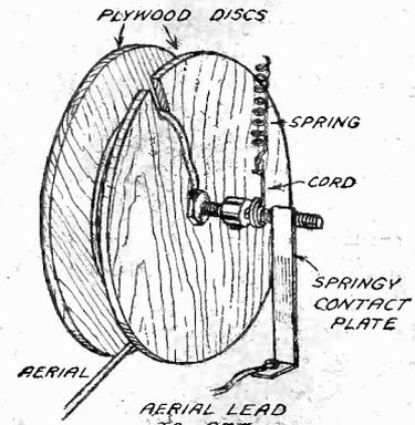
Fig. 5.—How a self-winding throw-out aerial can be made when the space permits. The "wheel" should be as large as permitted by the design of the set.
