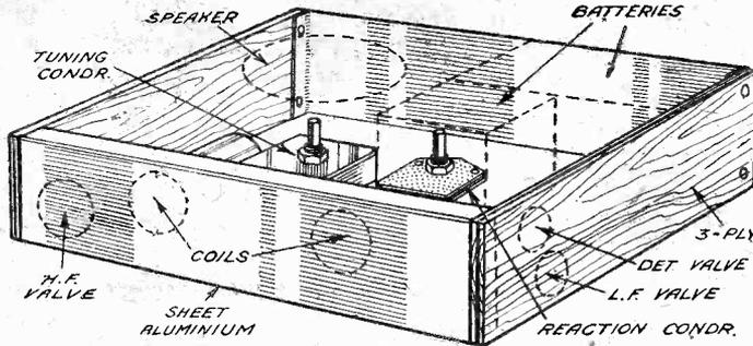
Fig. 4.—The illustration on the left gives an idea for the layout of a small portable to be carried in an attaché case of standard proportions.
