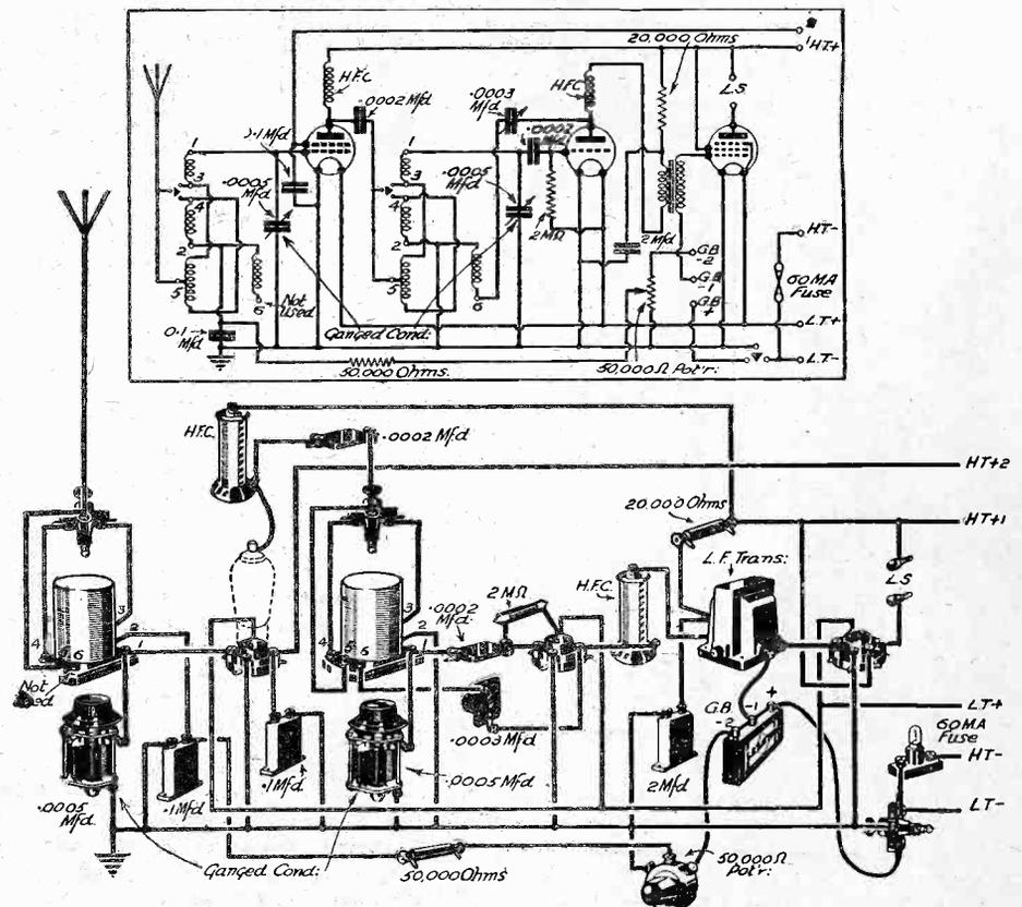
Fig. 1.—Above is a good circuit for a three-valve receiver having a V.M. value and using a pair of the tuners described in the accompanying text.
