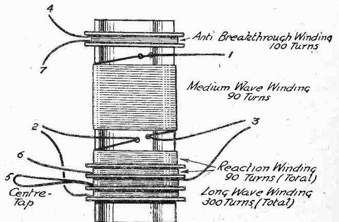
Fig. 7.—This sketch gives the necessary constructional details of a coil provided with an anti-break-through winding.
