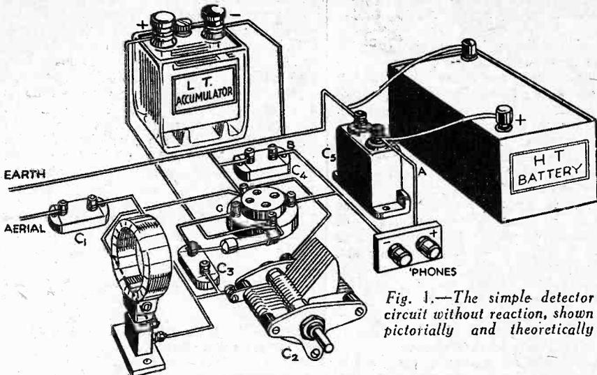
Fig. 1.—The simple detector circuit without reaction, shown pictorially and theoretically
