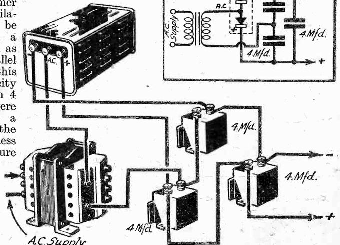
Fig. 9.—The above sketch shows the connections to a full-wave metal rectifier wired on the "voltage-doubler" principle.
