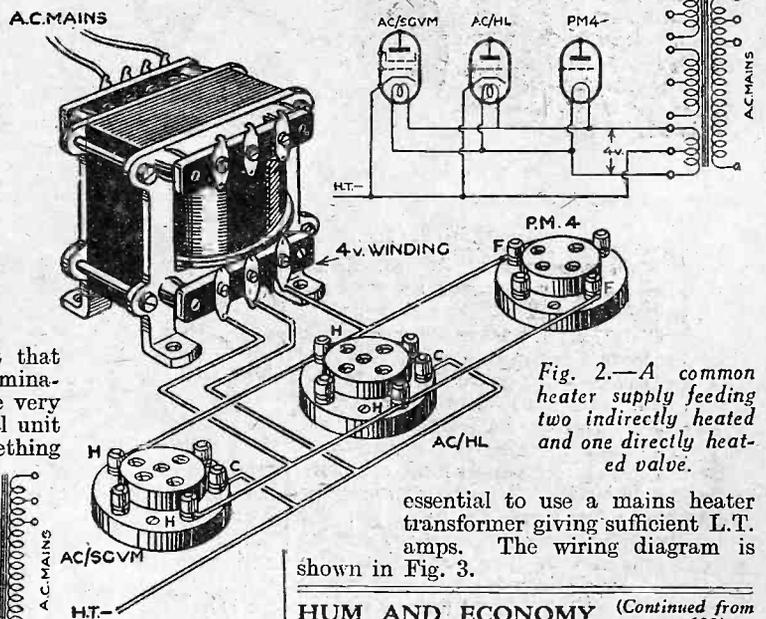
Fig. 2.—A common heater supply feeding two indirectly heated and one directly heated valve.
