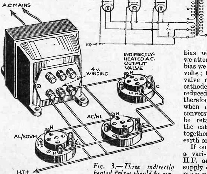
Fig. 3.—Three indirectly heated valves should be connected as shown in this illustration.
