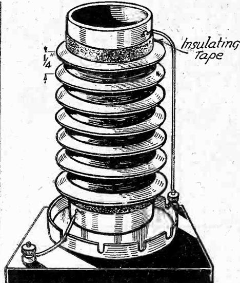
Fig. 2.—Constructional details of a very efficient H.F. choke made from the same materials as those employed for the coils.
