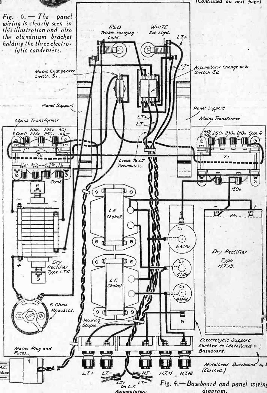
Fig. 4.— Baseboard and panel wiring diagram.
