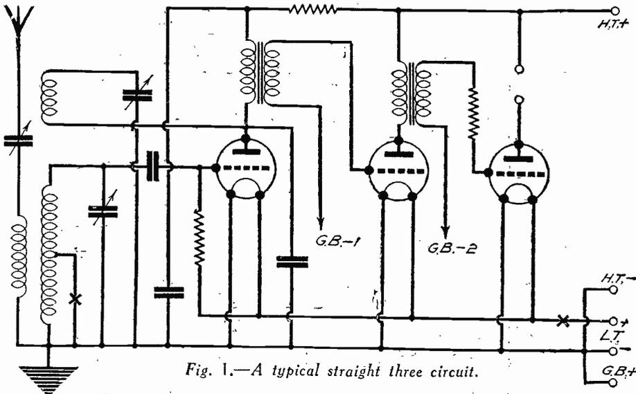
Fig. 1.—A typical straight three circuit.
