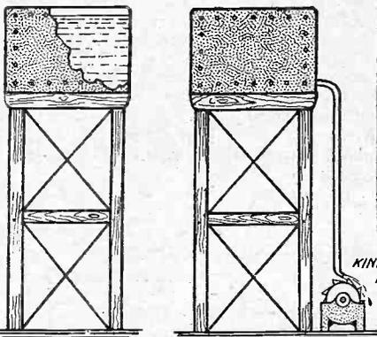
Fig. 1.—Difference of potential illustrated by the height of a tank of water.
