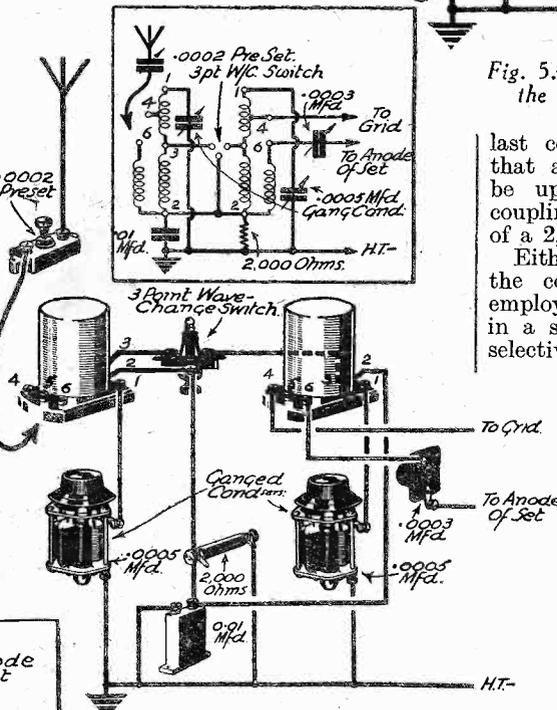
Fig. 4.—Pictorial and theoretical diagrams showing how a pair of home-made screened coils can be employed in an efficient band-pass filter circuit.
