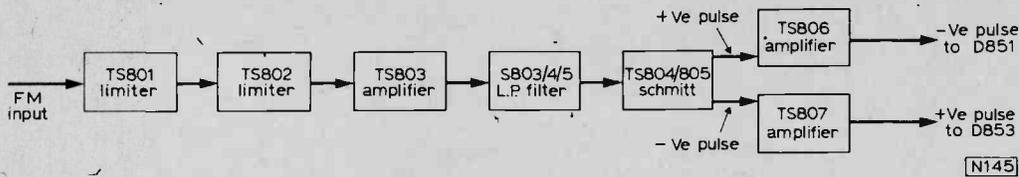
Fig. 11: Block diagram of the dropout detector circuit.
