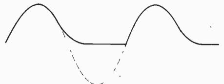
With a small resistance as load, the capacitor cannot store enough charge to keep current flowing, and the waveshape is almost as for a half-wave unsmoothed circuit
