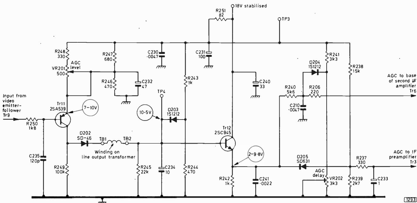
Fig. 3: A.G.C. circuit used in the Bush Model TV300. The i.f. strip comprises a preamplifier (TR3) which is mounted on a subpanel close to the u.h.f. tuner, followed by three stages (TR5, TR6 and TR8) on the main panel. TR8 is in the large centre rear screening can along with the video emitter-follower (TR9). A.G.C. is applied to the base of TR5 from the emitter of TR6 which thus acts as an a.g.c. amplifier as well as an i.f. amplifier.
