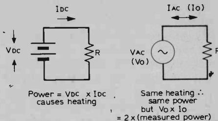
Fig. 11: Comparing power dissipated due to d.c. and a.c. supply sources.
