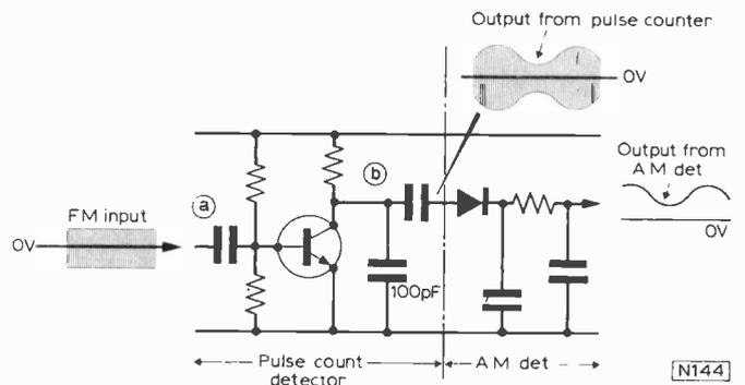
Fig. 10: A simple pulse-counting detector circuit.
