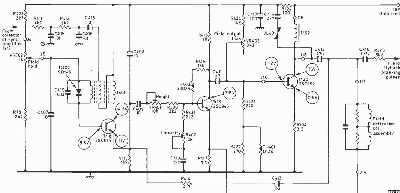
Fig. 2: Bush Model TV300 field timebase circuit. Field and line flyback blanking are carried out in the emitter circuit of the 2SC1103 video output transistor (TR10).
