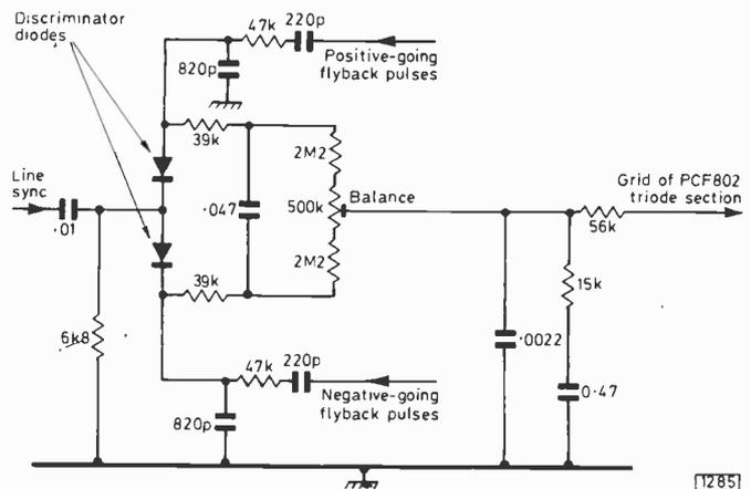
Fig. 1: Flywheel sync circuit used in the Grundig Models R500E/GB, T2002E/GB and P2002E/GB.
