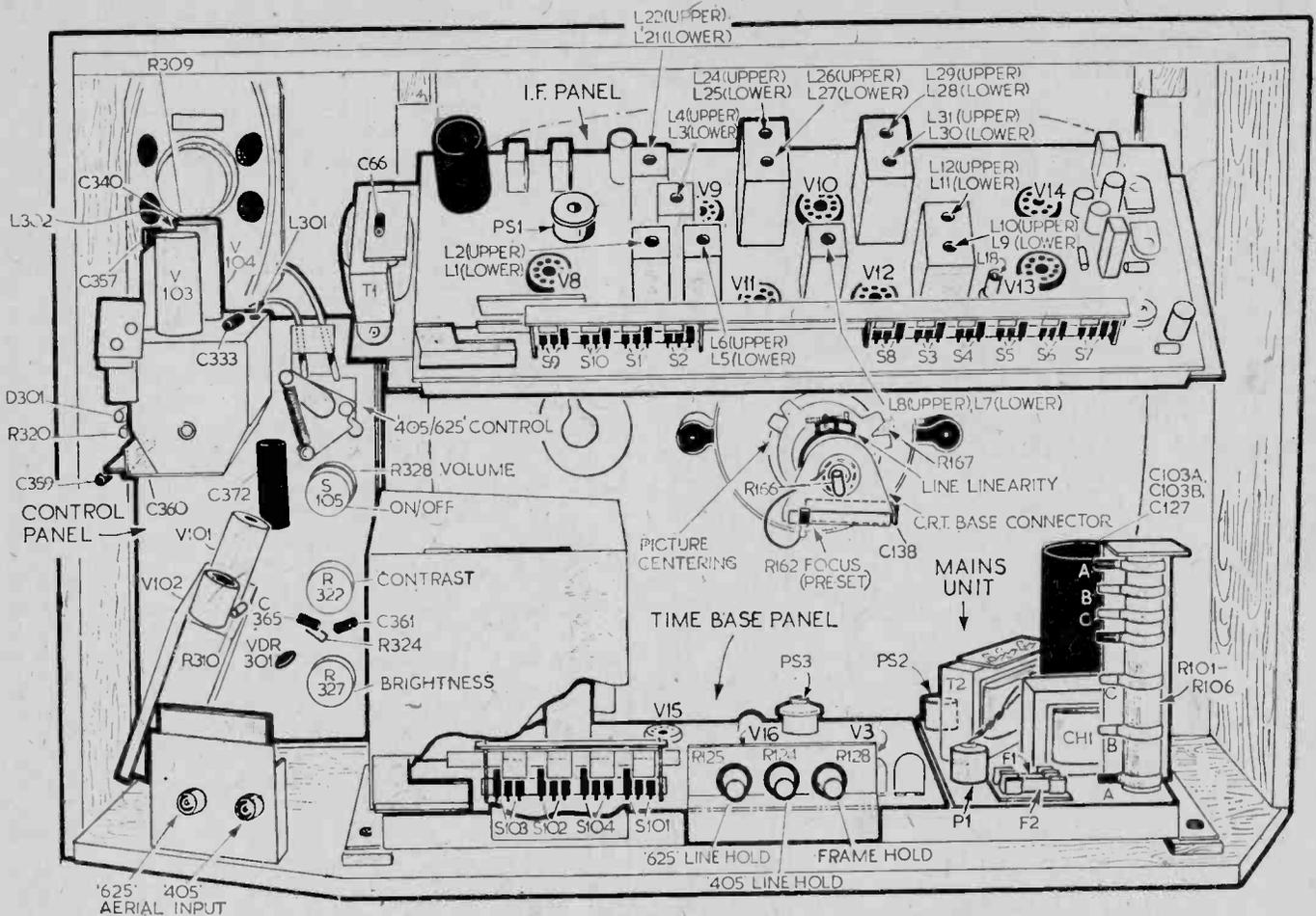
Fig. 3: Rear chassis view, DR1 series receivers. In the DR20 series, V10 and V14 are omitted and a transistor u.h.f. tuner is used. Diagram reproduced from "Electrical and Electronic Trader" Service Sheet 1729/T291 by kind permission of the Editor.
