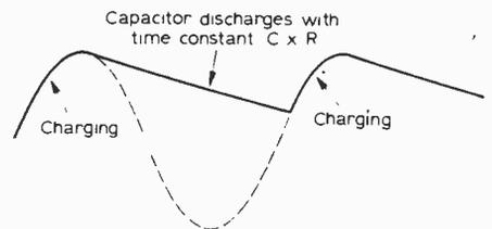
With a load, the capacitor starts discharging whenever the voltage of the rectifier input falls below  $V_0$ . When the rectifier conducts again, the capacitor charges again.
