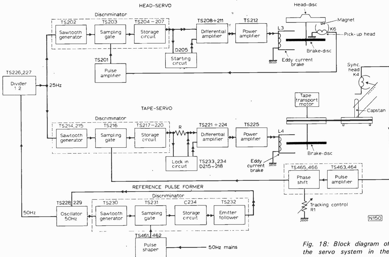
Fig. 18: Block diagram of the servo system in the Playback mode.
