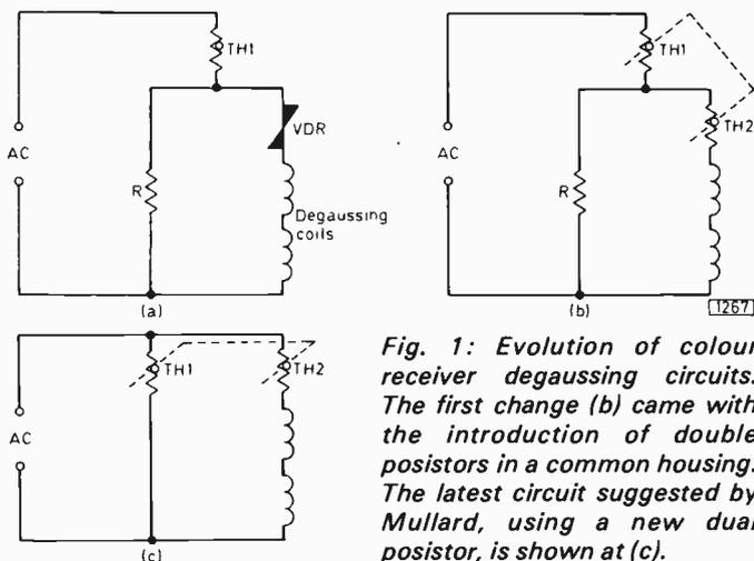
Fig. 1: Evolution of colour receiver degaussing circuits. The first change (b) came with the introduction of double posistors in a common housing. The latest circuit suggested by Mullard, using a new dual posistor, is shown at (c).
