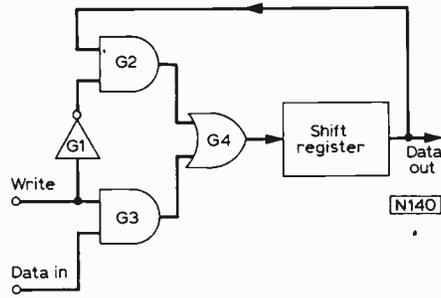
Fig. 30: Logic arrangement to allow recirculation of data.
