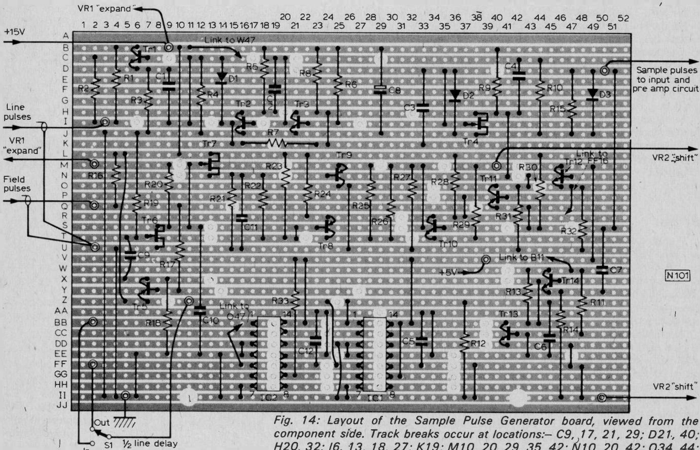
Fig. 14: Layout of the Sample Pulse Generator board, viewed from the component side. Track breaks occur at locations:- C9, 17, 21, 29; D21, 40; H20, 32; I6, 13, 18, 27; K19; M10, 20, 29, 35, 42; N10, 20, 42; O34, 44; P34; Q15, 38; R31; S13, 31, 41, 47; T13, 22, 32; W41; X13, 41; Y14, 27; Z9, 25; AA29; BB19, 24, 29, 39; CC19, 24, 29, 39; DD19, 24, 29, 39; EE19, 25, 29, 36, 47; FF19, 24, 29, 36; GG19, 24, 29, 36; HH19, 24, 29, 36.
