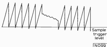
Fig. 12: Mixed ramp waveform with reduced field ramp to produce expanded display, i.e. only part of the line period is sampled.
