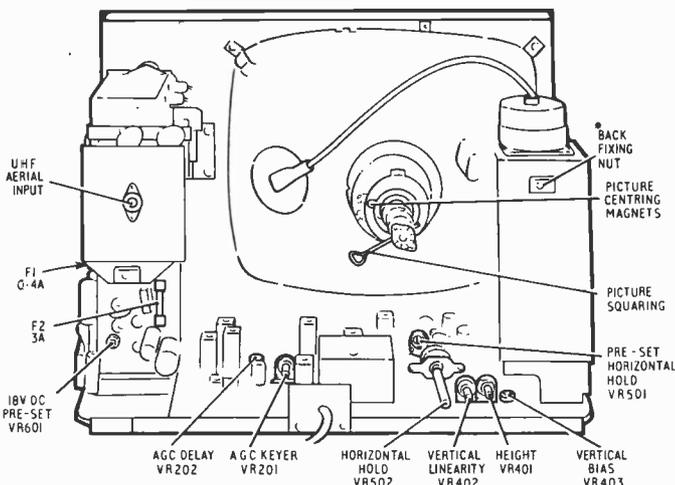
Fig. 1: Rear chassis view of the Bush Model TV300. The length of the top right back fixing screw must not exceed 14mm.
