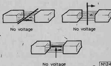
Fig. 4: A moving conductor must cut the lines of force to induce a voltage.
