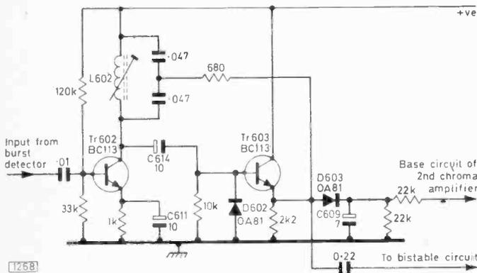
in question however the turn-on potential was barely 7V: ident coil adjustment increased this marginally, but there was obviously a defect somewhere in this part of the circuit.
