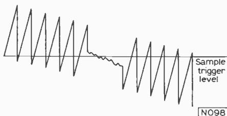
Fig. 11: Mixed line and field ramps for progressive triggering of line sample pulses.
