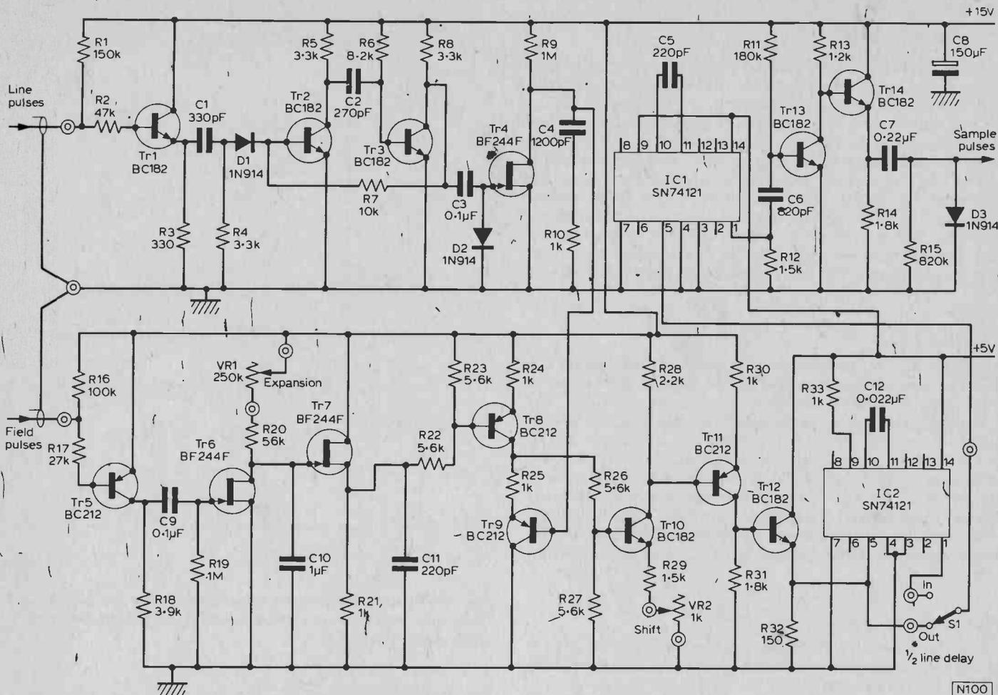
Fig. 13: Circuit diagram of the Sample Pulse Generator. The sampling pulses go directly to the gate of Tr6 on the Preamplifier (Fig. 9 last month).
