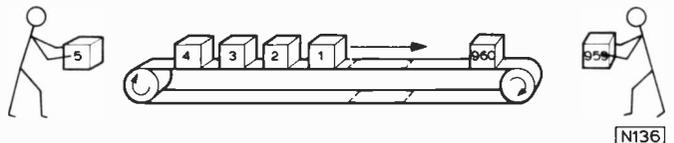
Fig. 26: The conveyor belt analogue of a sequential access memory. Each package represents one character.
