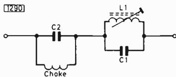
Fig. 2: Series/parallel filter used to obtain the local carrier required for synchronous video detection.
