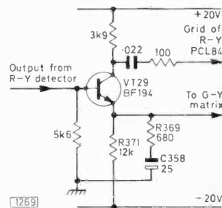
Fig. 2 (right): R - Y preamplifier stage, Pye 691 chassis.
