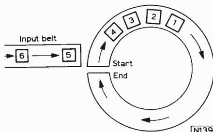
Fig. 29: The luggage carousel analogue of the recirculating shift register.
