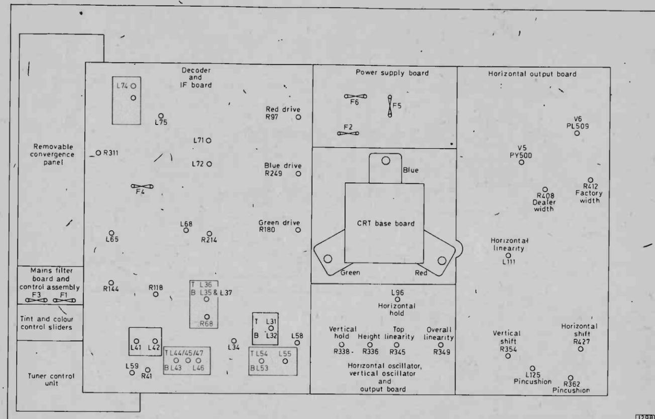
Fig. 1: Rear view of the CVC5 chassis.
