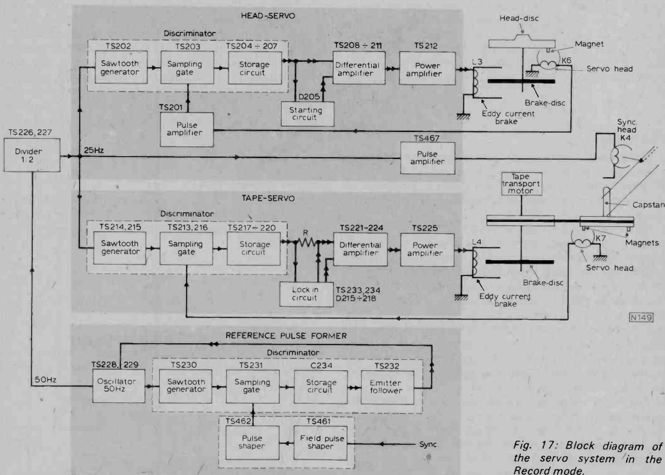
Fig. 17: Block diagram of the servo system in the Record mode.
