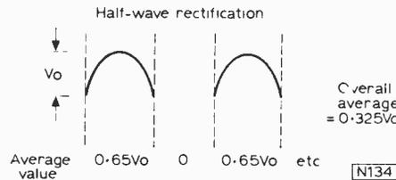
Fig 14: Average value of a half-wave rectified sine wave.
