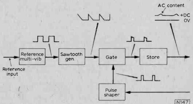
Fig. 15: Block diagram of the error-voltage generator.
