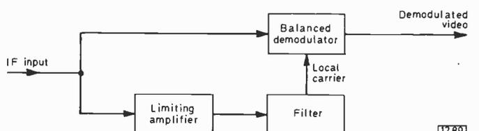
Fig. 1: Synchronous detection of the video signal, using a local carrier obtained from the transmitted carrier by limiting and filtering.
