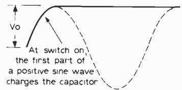
With no load, the capacitor charges up through the rectifier to the peak voltage  $V_0$
