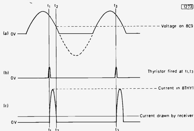
Fig. 2: (a) Duty cycle, or conduction angle, of thyristor 8THY1. (b) Trigger pulses from the diac fire the thyristor at times  $t_1$ ,  $t_3$  etc. (c) During the time  $t_1$  to  $t_2$  the reservoir capacitor 8C9 has to be charged sufficiently to be able to supply energy to the receiver until time  $t_3$ .
