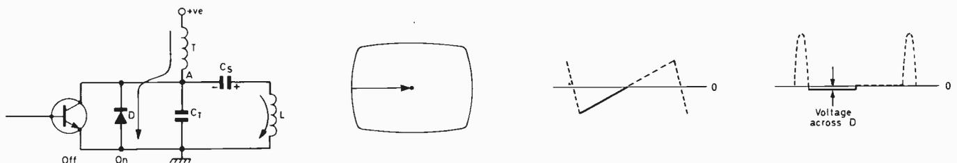
Fig. 4: Conditions during the first part of the forward scan – beam moving from the left-hand side towards the centre of the screen.
