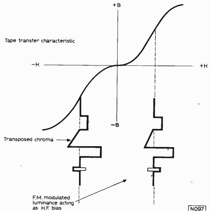
Fig. 8: The f.m. luminance signal acts as h.f. bias for the lower frequency chrominance signal on recording.
