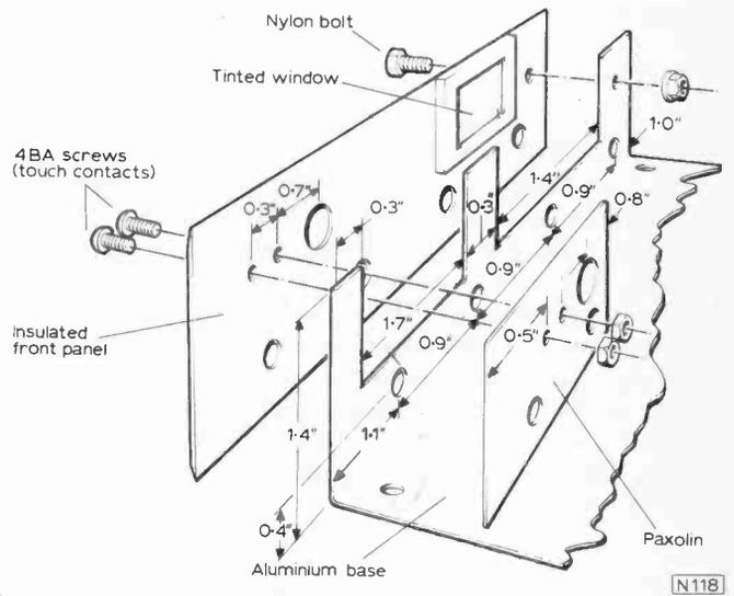
Fig. 7: Arrangement of front panel on the prototype Receiver/Control unit. The panel itself was made from material 3mm ( $\frac{1}{8}$ in) thick.
