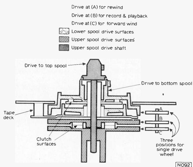
Fig. 2: Principle of the tape spool drive mechanism.
