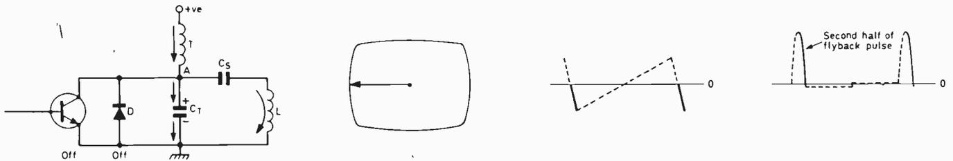
Fig. 3: Conditions during the second half of the flyback – beam moving from the centre towards the left-hand side of the screen.
