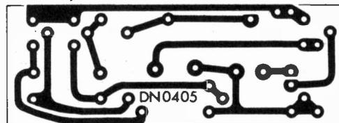
Fig. 5: P.C.B. design and component layout for the ultrasonic transmitter unit, both shown full size.
