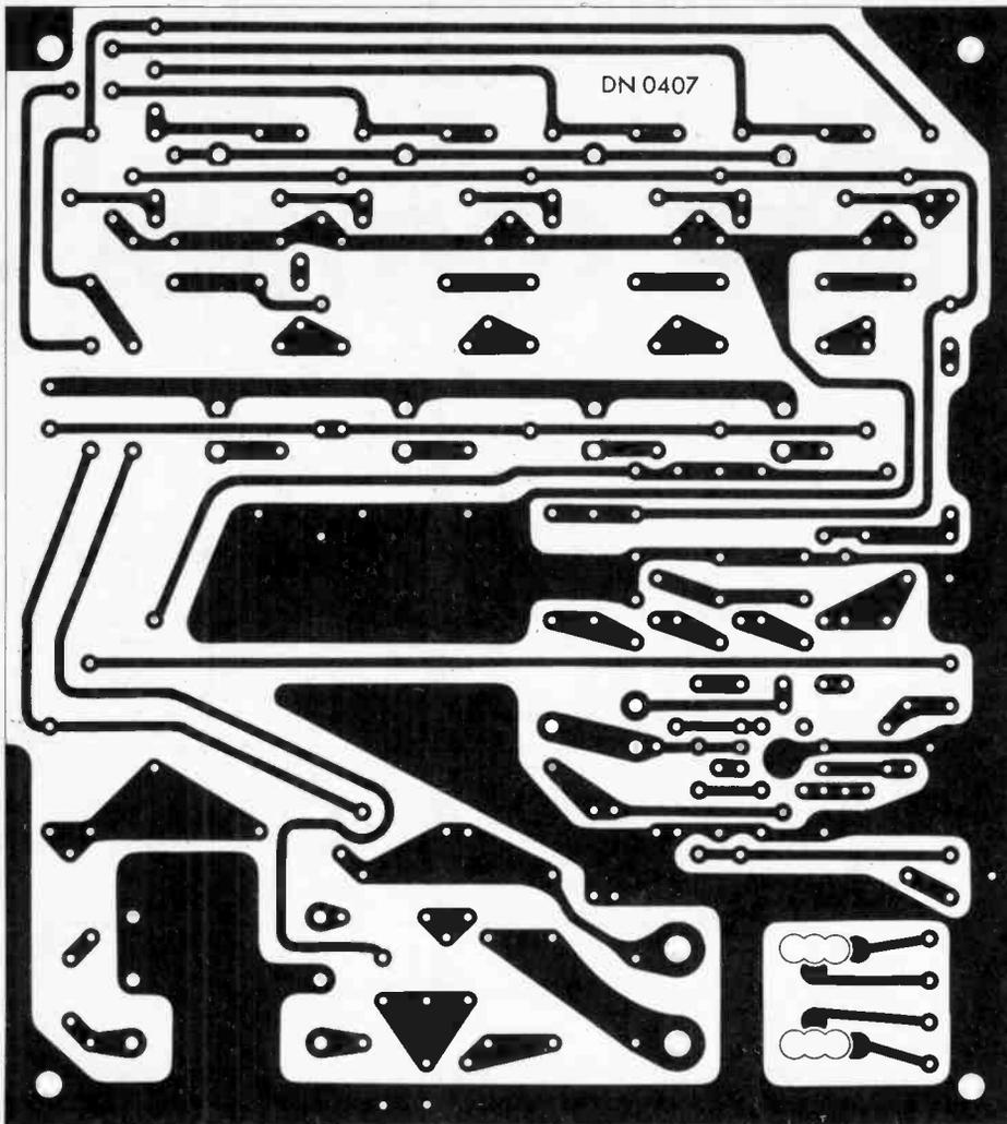
Fig. 6: The p.c.b. design (left) and component layout (right) for the Receiver/Control unit, both shown full size. For details of connections to the relay contacts, see text.
