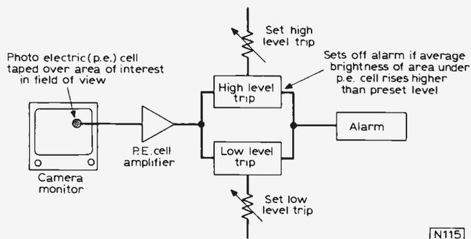
Fig. 3: A simple "add-on" movement detector, which requires no electrical connection to the television system.
