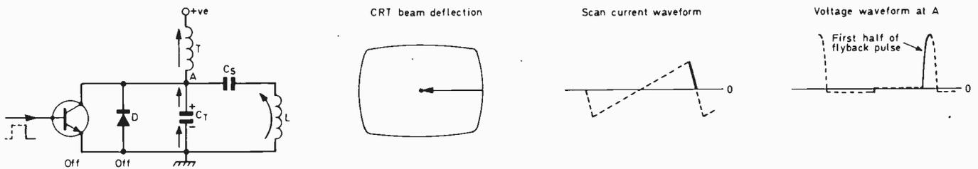
Fig. 2: Conditions during the first half of the flyback – beam moving from the right-hand side towards the centre of the screen.
