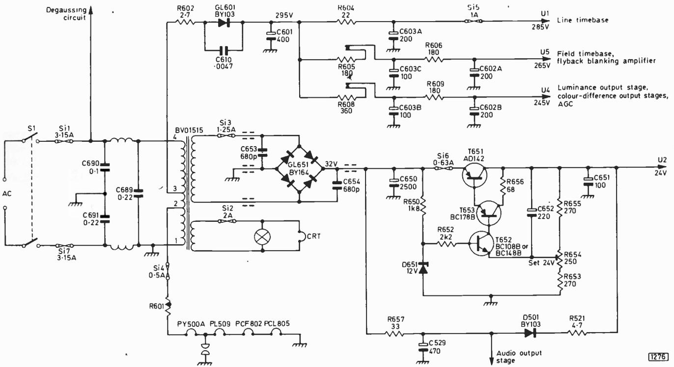
Fig. 1: Power supply circuits. D501 and R521 protect the audio output transistors.
