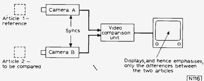
Fig. 4: Basic arrangement of an image comparator.
