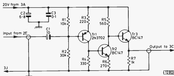
Fig. 1: Fast video amplifier circuit. Use a 6.8µF solid tantalum capacitor (C2) on the board as well as adding one on the RGB board – see text.
