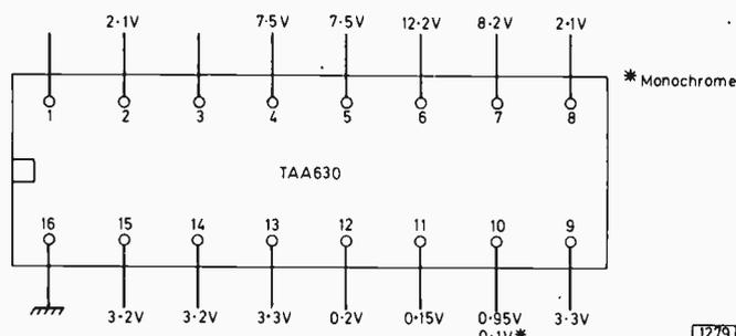
Fig. 4: D.C. voltages at the pins of the TAA630 i.c. in the decoder. Measured with a valve voltmeter and signal present.
