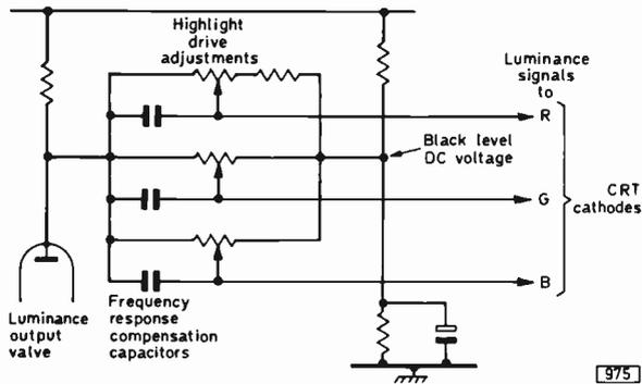
Fig. 2: Using this simple circuit, correct grey-scale tracking is maintained despite changes of h.t. voltage.
