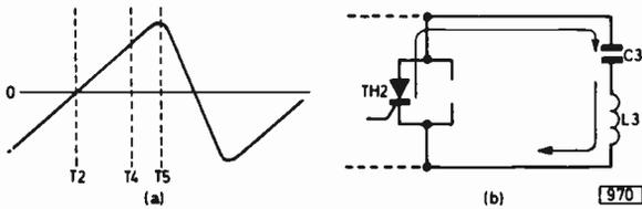
Fig. 3: Condition of the circuit between times  $T_2$  and  $T_4$ , with  $TH_2$  conducting.
