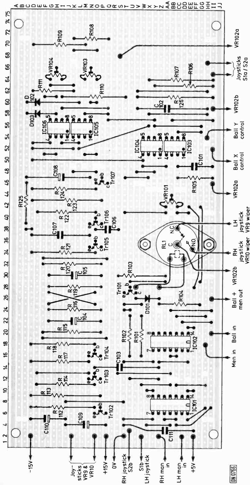
Fig. 15: Layout of the simple game board, viewed from the copper side.
