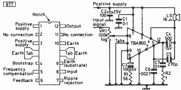
Fig. 1 (left): Pin connections to the TBA800. The TBA810S and TBA810AS are the same except that there is no connection to pin 3.
