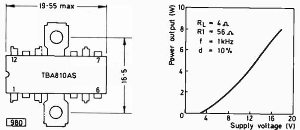
Fig. 7 (left): Outline drawing of the TBA810AS.
