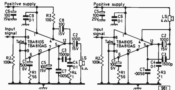
Figs. 9 and 10: Alternative audio circuits using the TBA810S or TBA810AS.
