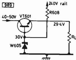
Fig. 1 (left): Operation of the series emitter-follower (VT601) which stabilises the 30V rail.
