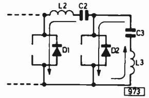
as the current in the coils builds up and at time  $T_0$  the voltage is insufficient to drive current through  $L_2$ ,  $C_2$  and the coils. The current then finds an easier path (see Fig. 7) through scan diode  $D_2$  and we are back at the start of the next forward scan period.
