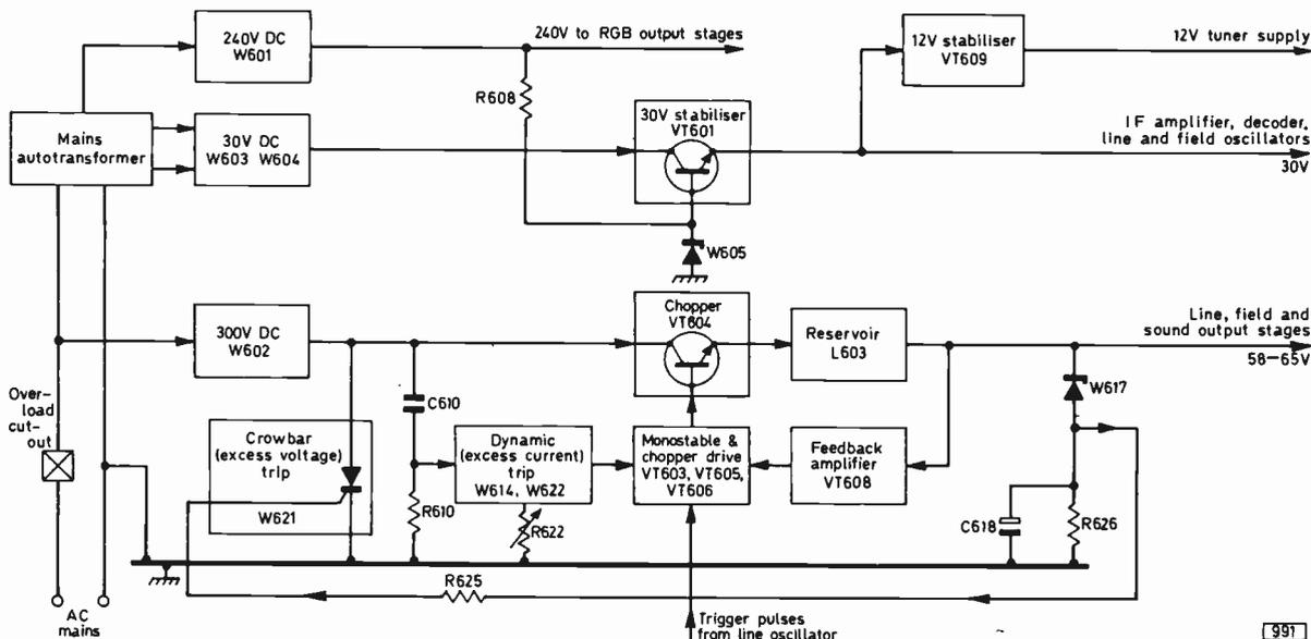
Fig. 3: Block diagram of the power supply arrangements used in the BRC/TCE 3000/3500 colour chassis.
