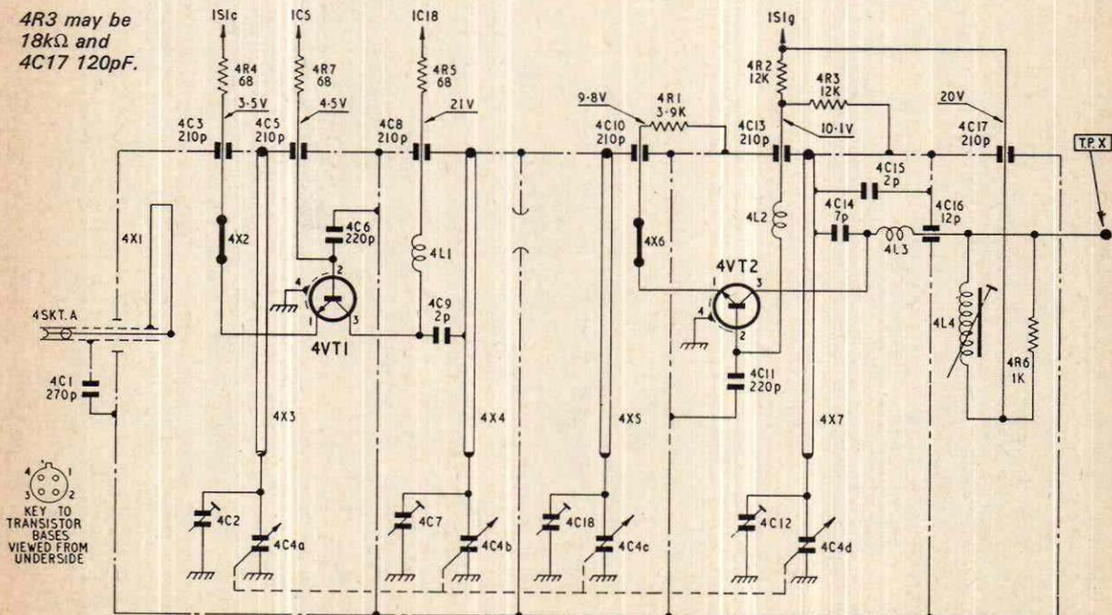
Fig. 5: U.H.F. section of tuner unit type A633. 4VT1 BF180, 4VT2 BF181.
