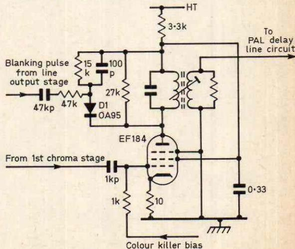
Fig. 1: Second chroma stage in the Philips G6 colour chassis, showing the burst-blanking system.
