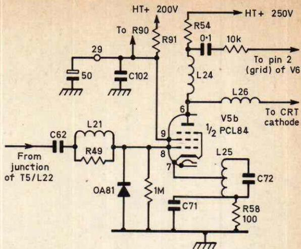
Fig. 5: Modified video amplifier circuit.
