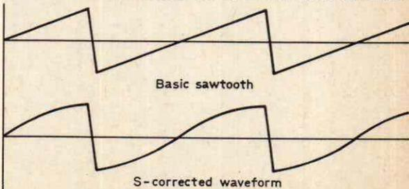
Fig. 7: Illustrating S-correction of line scanning.
