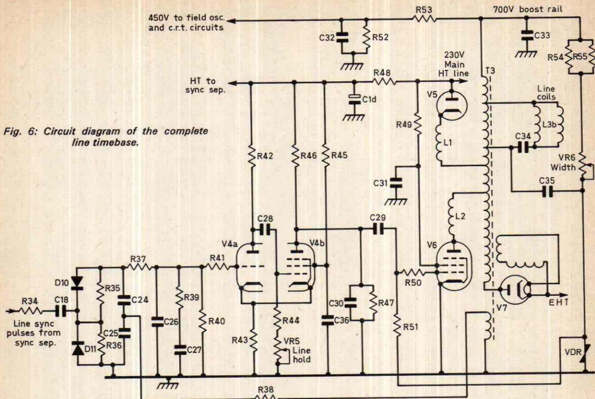
Fig. 6: Circuit diagram of the complete line timebase.
