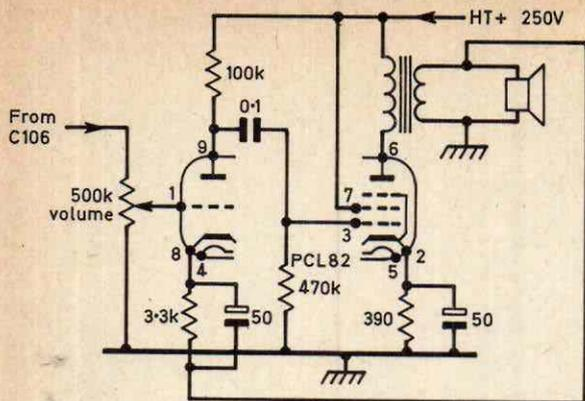
Fig. 3: Suggested audio amplifier circuit.
