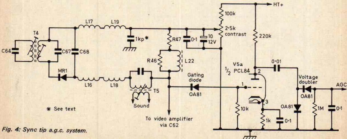
Fig. 4: Sync tip a.g.c. system.
