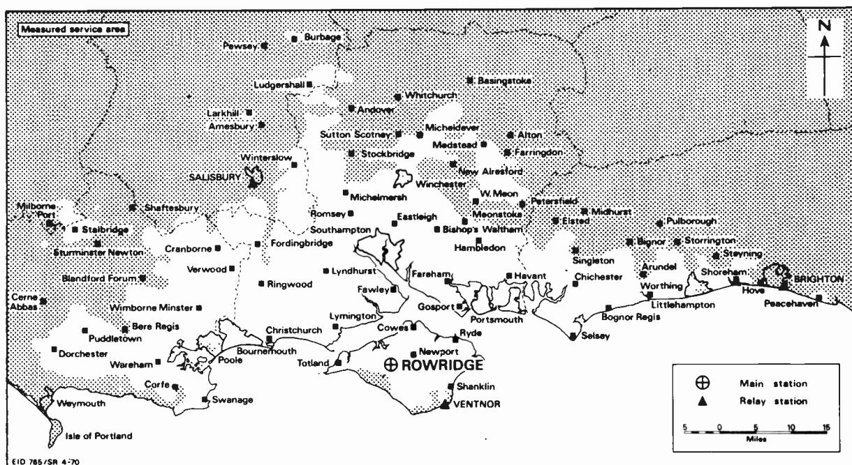
The above BBC map shows the approximate service area of the Rowridge u.h.f. transmitter (maximum vision e.r.p. 500kW, directional aerial). Small pockets of poor reception too small to be shown in this map may be experienced. Channels: BBC-2 24; ITA 27; BBC-1 31. Horizontal polarisation, receiving aerial group A.
