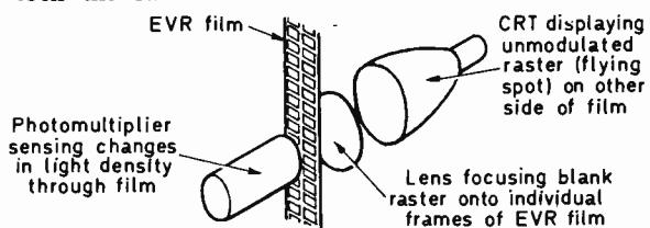
Fig. 4: Principle of flying-spot scanning.
