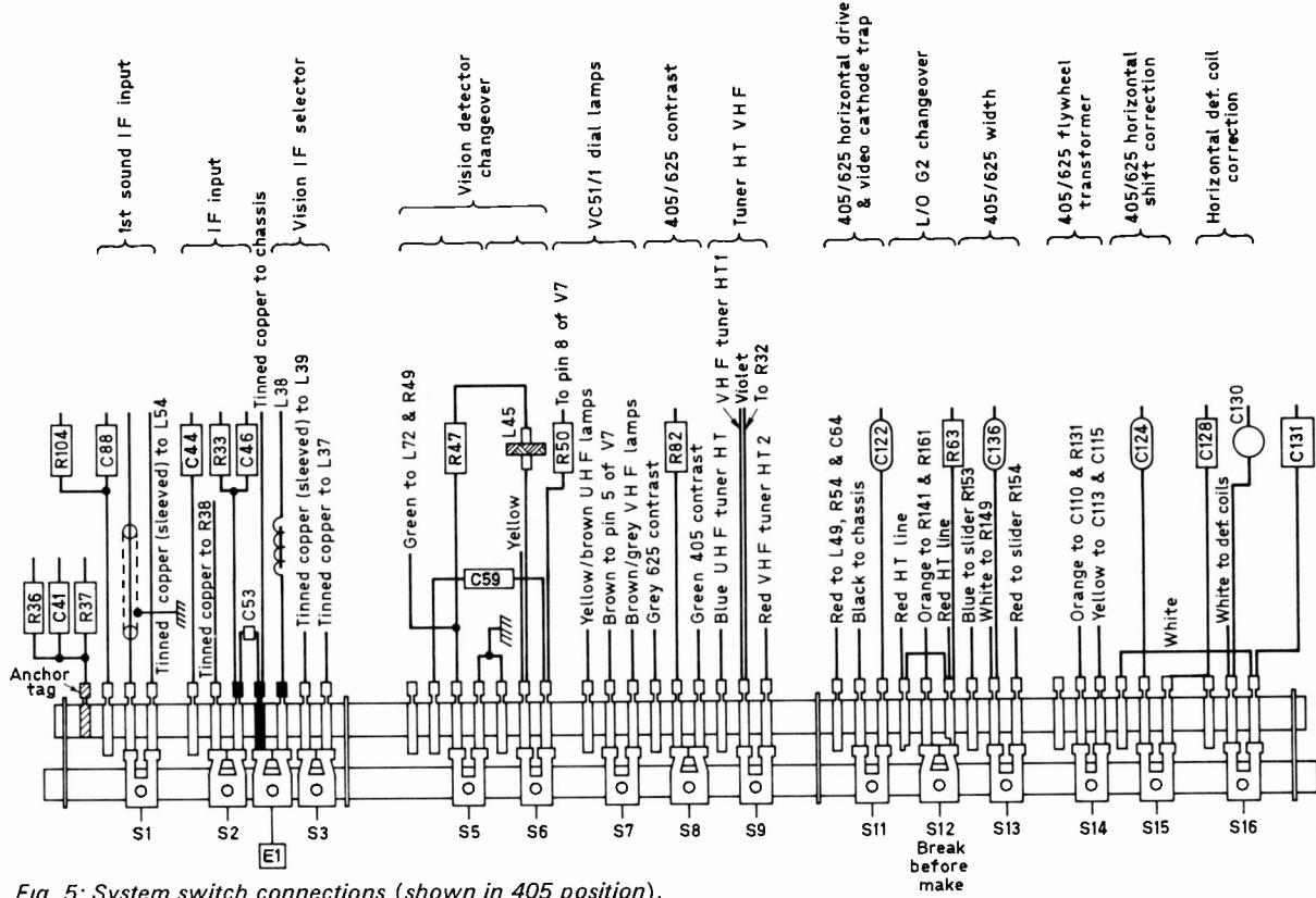
*Fig. 5: System switch connections (shown in 405 position).*
