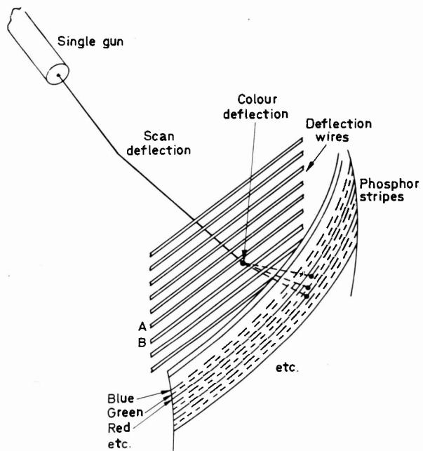
Fig. 3: Principle of the beam deflection type of tube. The chromatron is an example of this type of tube. The electron beam from a single gun lands on a green stripe if undeflected; if wire A is positive and wire B negative it lands on a blue stripe; if wire A is negative and B positive it lands on a red stripe.
