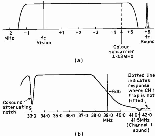
Fig. 1: (a) Transmission spectrum of a 625-line transmitter. (b) Response curve of an i.f. strip, using intercarrier sound, to handle the above transmitter spectrum. Note that the sense of the vision and sound signal is reversed at i.f. as the tuner's local oscillator operates above the channel frequency.
