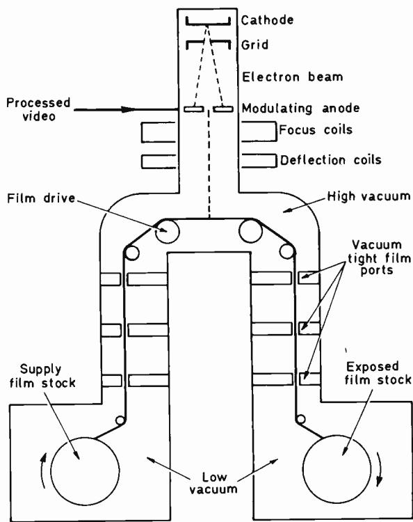
Fig. 2: Electron-beam recorder.
