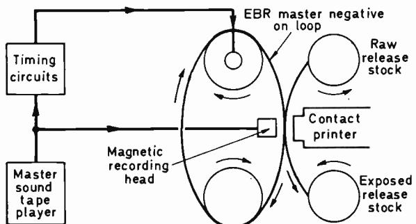
Fig. 3: High-speed EVR printer arrangement.
