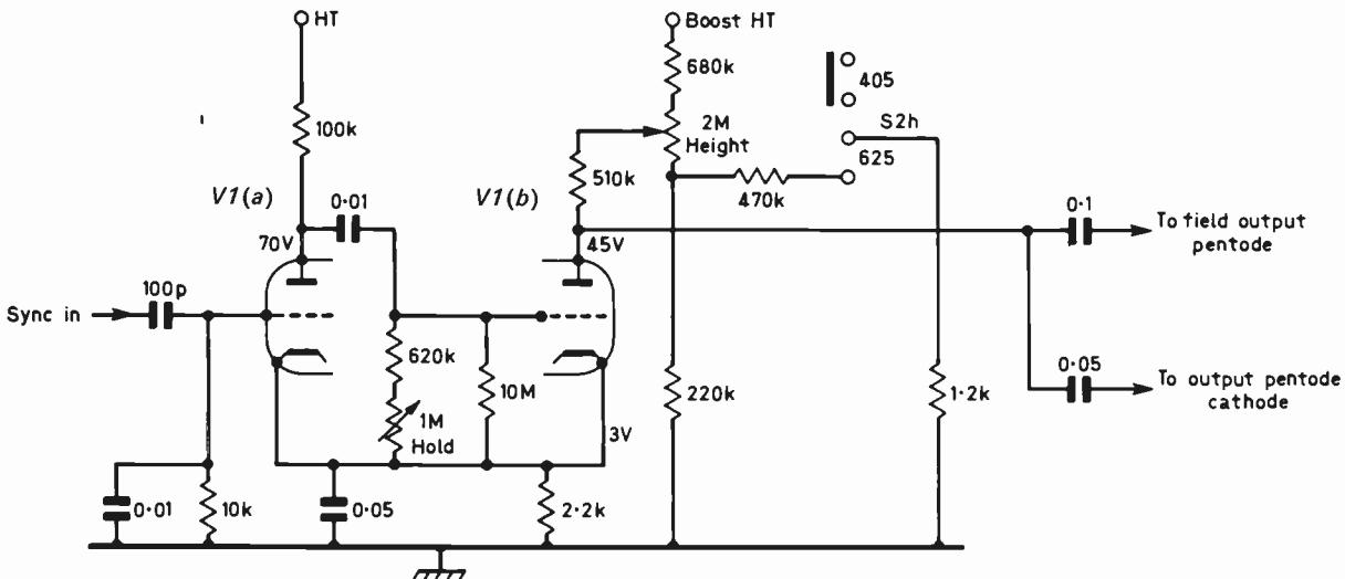
Fig. 1: Field generator circuit of the Bush Model TV115L. System switch S2h slightly reduces the right-hand triode anode voltage on 625 lines to equalise height. Fault symptoms were greatly reduced height and completely folded-over picture.
