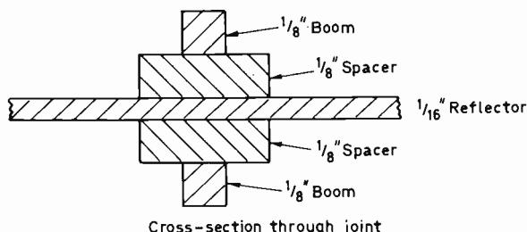
Fig. 2: Reflector assembly.
