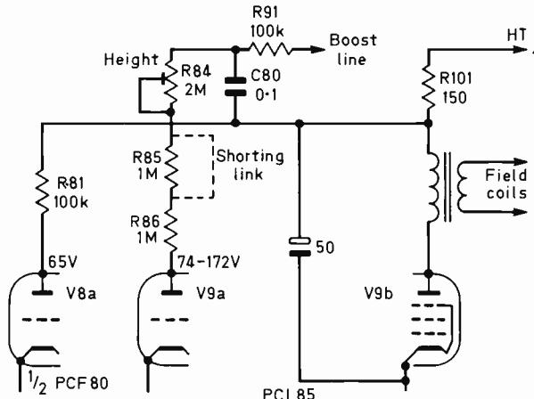
Fig. 2: Anode h.t. supplies in the RGD Model 628 field circuit. Height on this receiver had suddenly reduced to about half due to severe reduction of V9a anode voltage.
