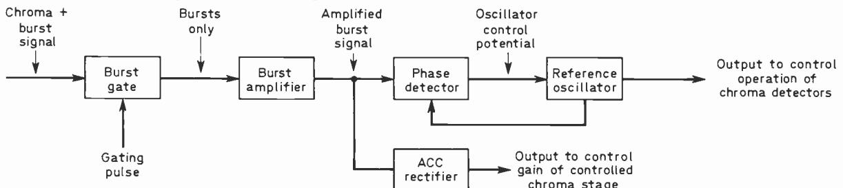
Fig. 1: Block diagram of the burst, a.c.c. and reference oscillator sections of a colour receiver decoder.
