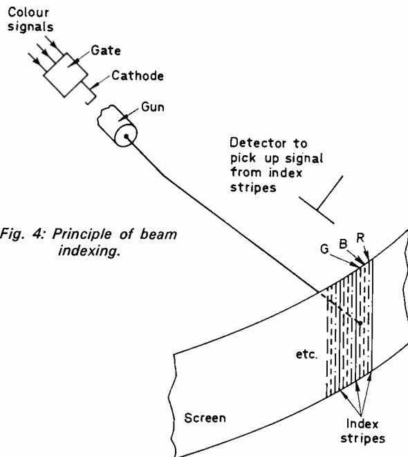
Fig. 4: Principle of beam indexing.
