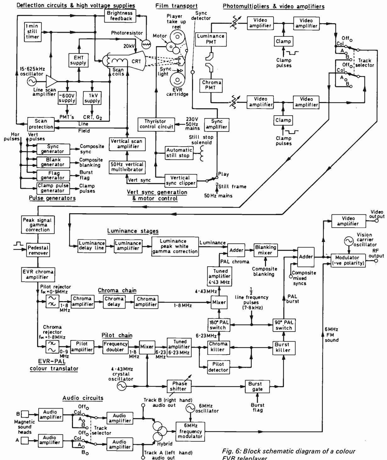
Fig. 6: Block schematic diagram of a colour EVR teleplayer.
