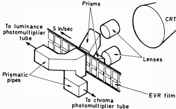
Fig. 5: Optical system in an EVR teleplayer.
