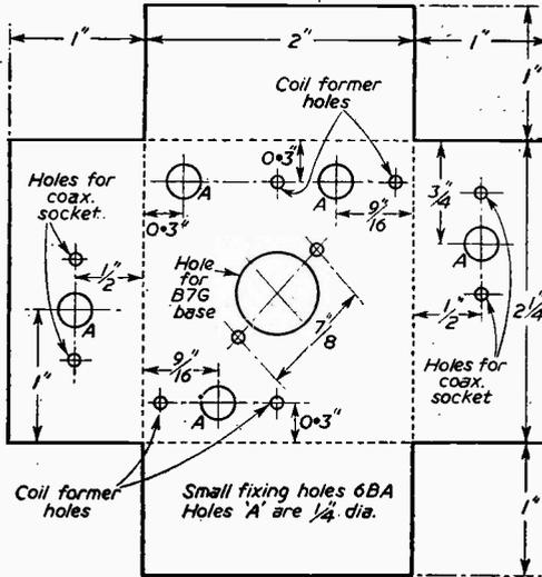
Fig. 2.—Showing drilling and fixing hole details.
