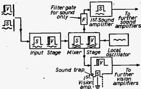
Fig. 20.—A block diagram similar to Fig. 19, but relating to a superhet receiver. See also Fig. 21.
