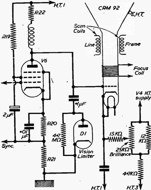
Fig. 2.—Video amplifier output, C.R.T. and brilliance circuit.
