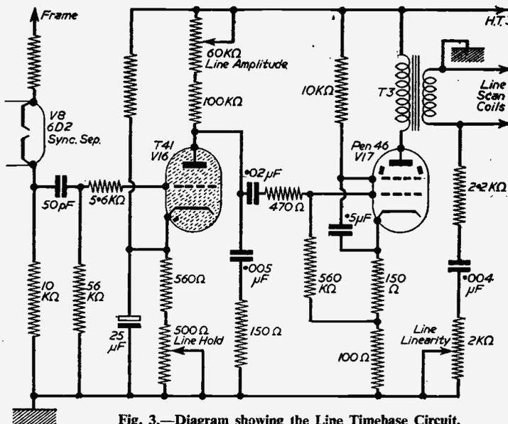
Fig. 3.—Diagram showing the Line Timebase Circuit.
