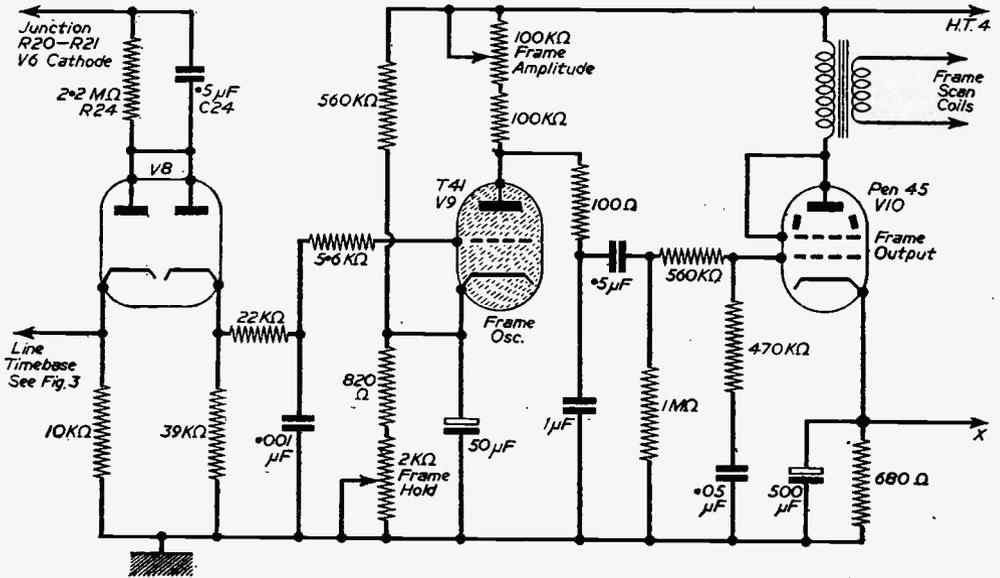
Fig. 4.—Frame Timebase and Sync Separator circuit.
