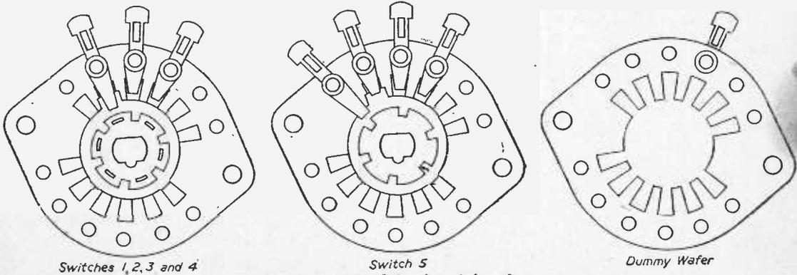
Fig. 3.—Details of the six switch wafers.
