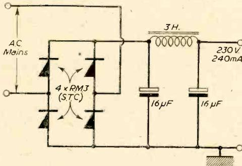
Fig. 8.—Bridge rectifier capable of working from the mains. Neither side of mains directly connected to chassis.
