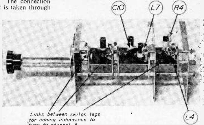
View of the switch unit with some components identified.
