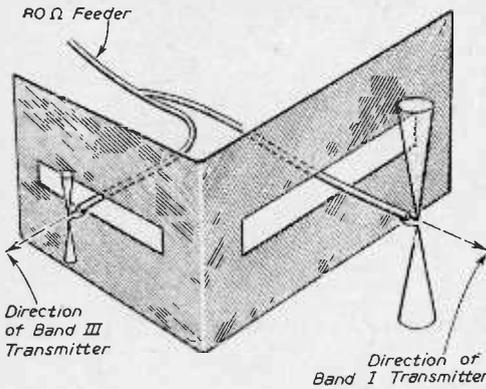
Fig. 3.— Slot length = R. Slot width =  $\frac{R}{12}$
