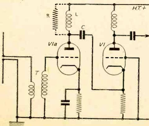
Fig. 4. — The basic cascode circuit.
