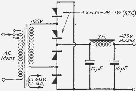
Fig. 3.—Bridge rectifier developed from the push-pull version of Fig. 2.
