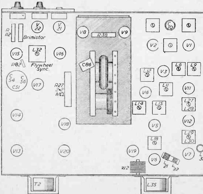
Fig. 3.—Simplified under-chassis view. Note W2 V6 bias metal rectifier, core of L32 and R82. The PL81 grid-leak is R27 2.2 M $\Omega$ . R116 may not be fitted.
