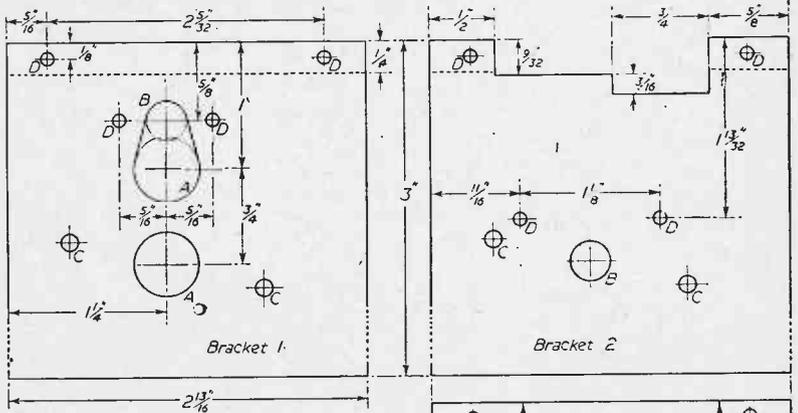
A Holes — 1/2" Dia. B Holes — 5/16" Dia.
