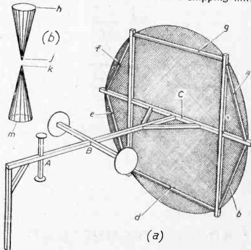
Fig. 2.—For horizontal polarisation dipole may require additional support. (a) All woodwork 1 in. square excepting a, b, d, e, f and g, these being 1 in. x  $\frac{1}{2}$  in. All joints half-lapped and screwed excepting at A and B where  $\frac{1}{2}$  in. holes are drilled and  $\frac{1}{2}$  in. dowel rod fitted. Bases of cones are plywood discs. (b) Copper strip or bonding wire around h, j, k and m to support wires. Connect coaxial cable to i and k.
