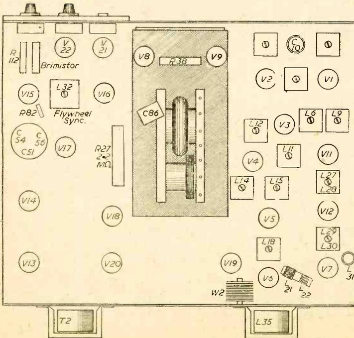
Fig. 3.—Simplified under-chassis view. Note W2 V6 bias metal rectifier, core of L32 and R82. The PL81 grid-leak is R27 2.2 M $\Omega$ . R112 may not be fitted.
