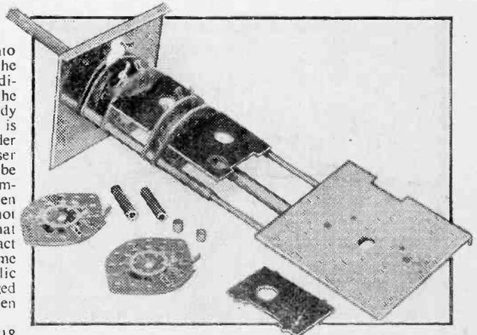
Component parts of the switch assembly.
