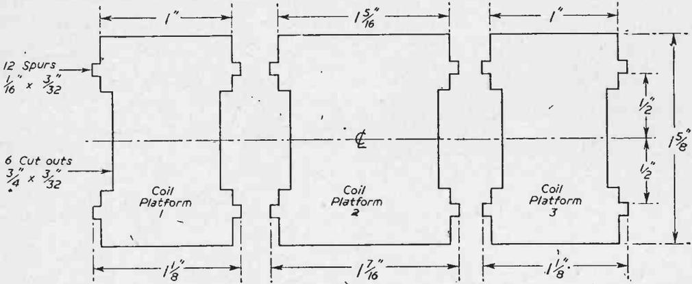
Fig. 5.—Details of the coil platforms—made from paxolin.
