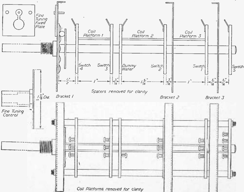
Fig. 4.—Details of assembly of the switch unit.
