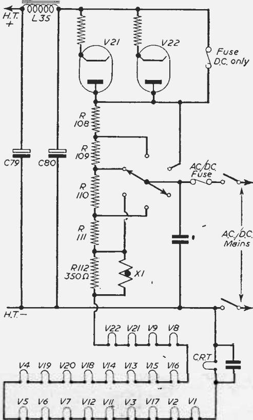
Fig. 4.—Showing power supplies and heater chain. R112 only fitted with Brimistor (X1) or Varite.
