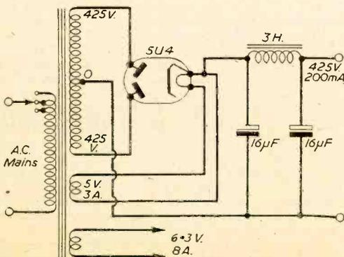
Fig. 1.—Full-wave supply system as used for a VCR97 Receiver. Additional smoothing is not shown.
