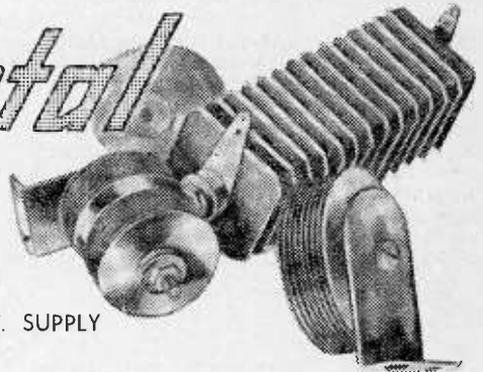
THE H.T. requirements of a television set are often met by using metal rectifiers. Valve rectifiers, because of their heavy emission, fail more often than other valves, while metal rectifiers, if not overloaded, last almost indefinitely.
