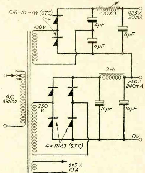
Fig. 4.—A more economical supply for a VCR97 Receiver, which can later be used for a magnetic picture tube if required.
