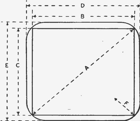
Fig. 5.—Showing how the diagonal measurement could mislead.
