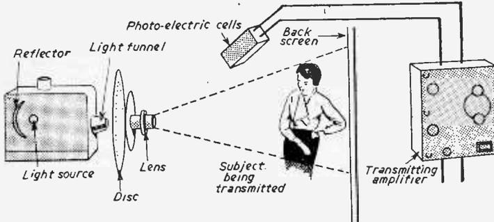
Fig. 3.—Diagram illustrating the manner in which the early television system worked.
