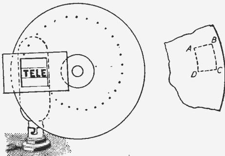
Fig. 4.—Another illustration of the method of building up an image by a mechanical disc.
