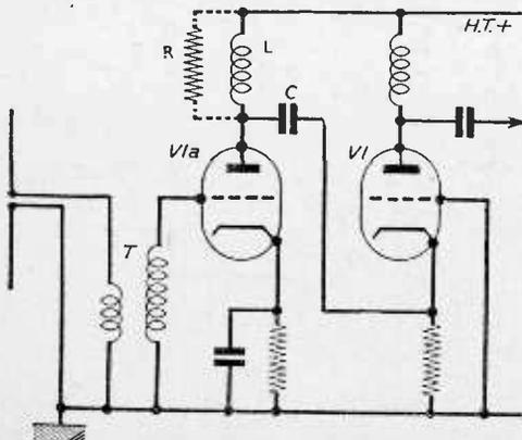
Fig. 4. — The basic cascode circuit.
