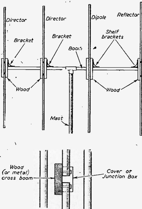
Fig. 10.—"Yagi" array and details of gap in dipole.
