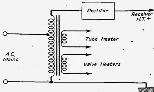
Fig. 1.—The familiar auto-transformer system of H.T. and heater supplies used on modern A.C. receivers.
