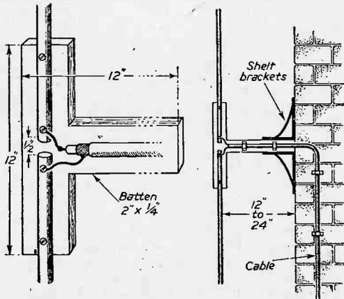
Fig. 1 (left).—Suggested mounting for the dipole. Fig. 2 (right).—A method of wall-fixing.
