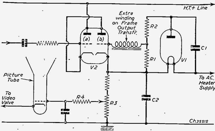
Fig. 57.—Protection circuit used in Philips' projection receiver, Model 799A.
