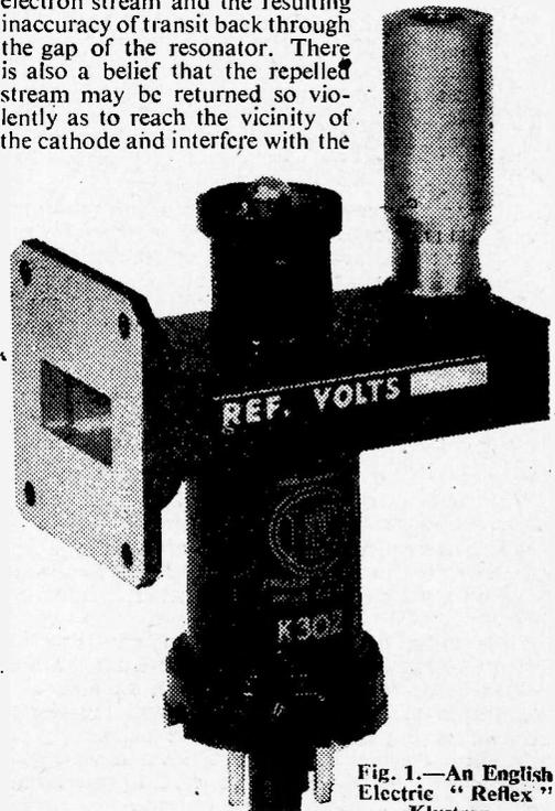
Fig. 1.—An English Electric "Reflex" Klystron.
