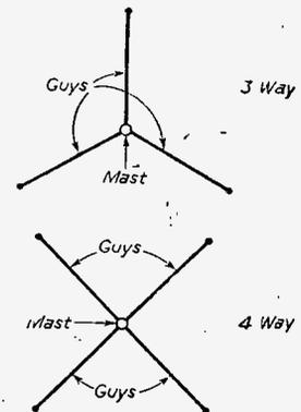
Fig. 11.—Method of guy in a heavy mast type aerial.
