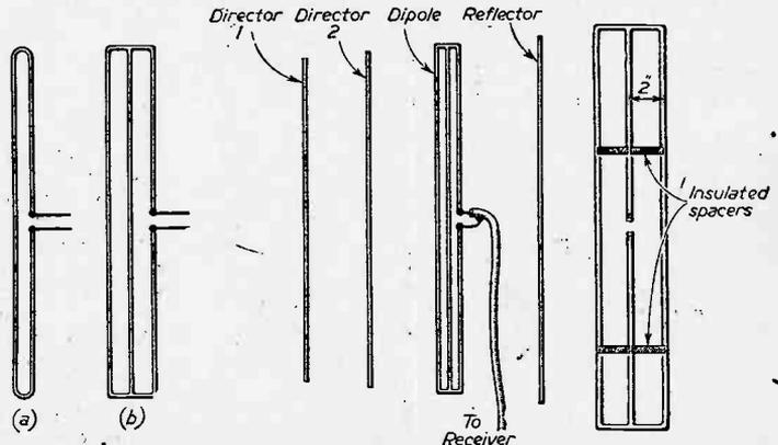
Fig. 7 (left).—Folded dipole aeriels. Fig. 8 (centre).—Folded dipole with directors. Fig. 9 (right).—A triple-folded dipole.
