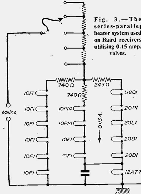
Fig. 3.—The series-parallel heater system used on Baird receivers utilising 0.15 amp. valves.
