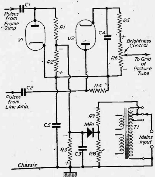
Fig. 56.—Picture-tube protection circuit used in the directly-viewed Ekco Model TC165.
