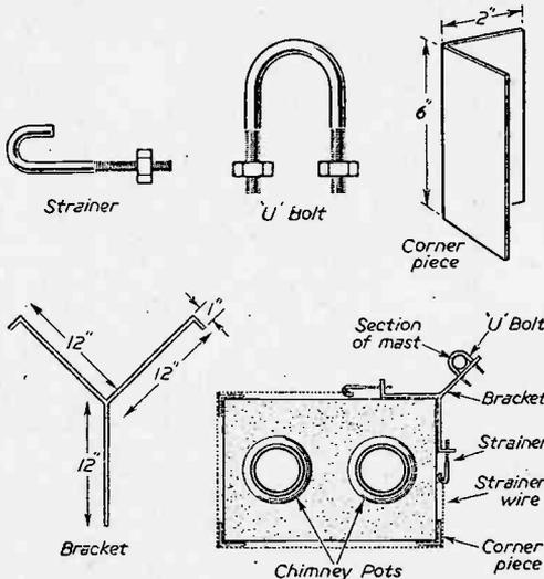
Fig. 6.—Details of chimney-lashing.
