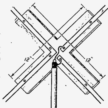
Fig. 5.—Mounting of the double-vee aerial shown in Fig. 3.
