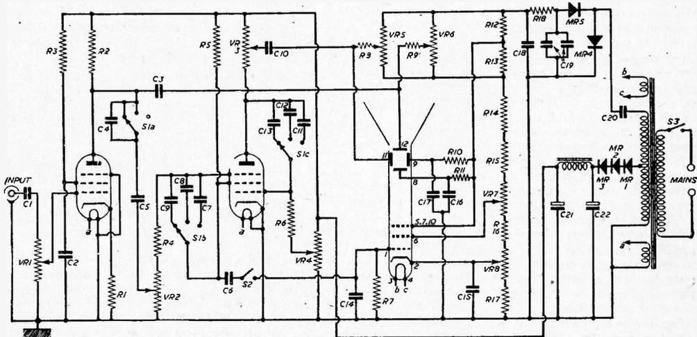
Fig. 1.—Complete theoretical circuit of the TV 'scope.
