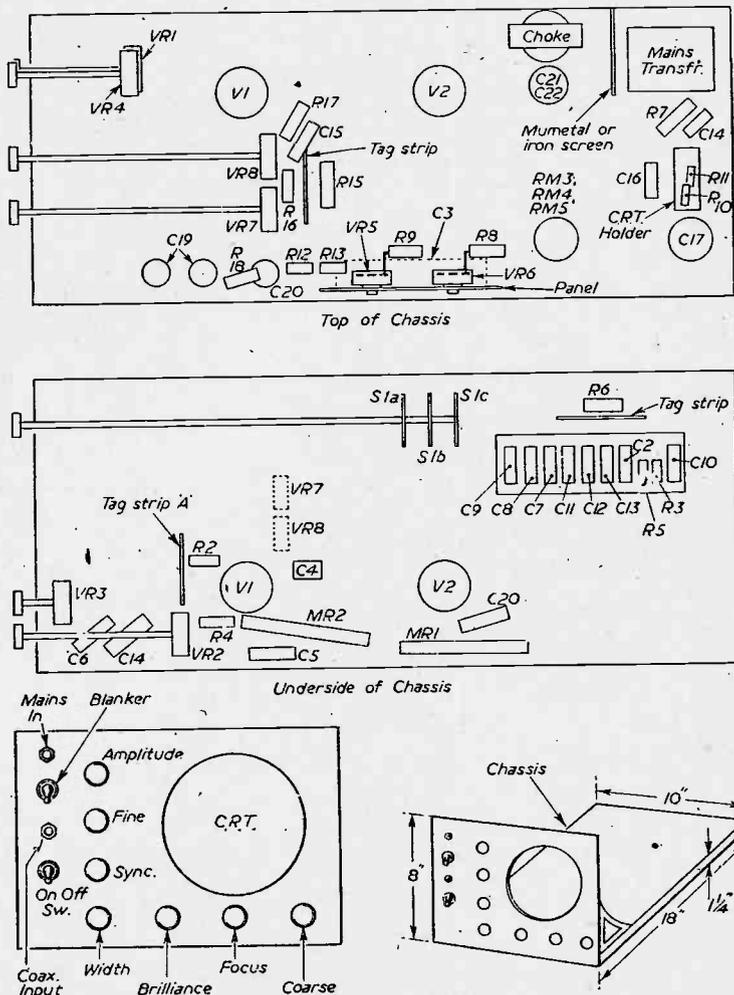
Fig. 2.—Details of the layout and positions of the main components.
