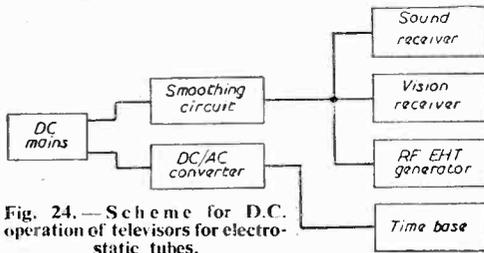
Fig. 24.—Scheme for D.C. operation of televisions for electrostatic tubes.
