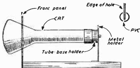
Fig. 2.—Method of mounting the tube as described last month.
