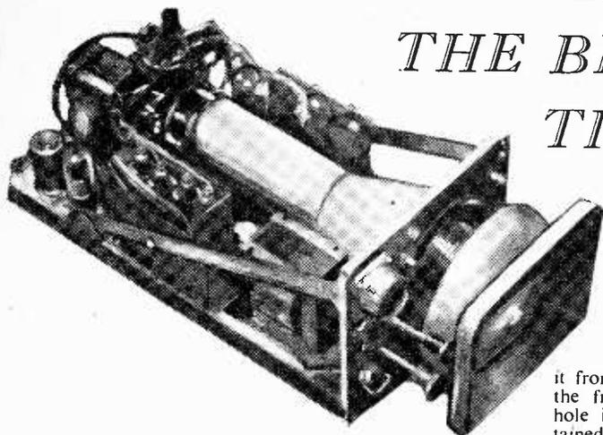
**T**WO cords are used one above and one under the tube, the ends being fixed in the bolts which held the original tube mask. Fishing line of the strong variety is a very suitable material to use.
