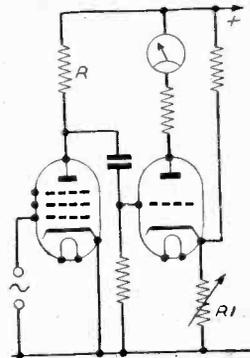
Fig. 3—A circuit arrangement for checking the load capacity.
