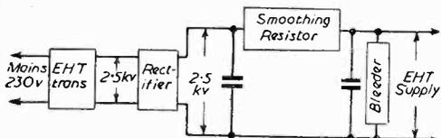
Fig. 28.—A mains type E.H.T. supply.
