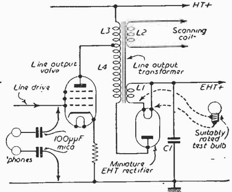
Fig. 12.—A typical line flyback E.H.T. circuit.
