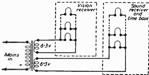
Fig. 22.—A parallel heater wiring arrangement.
