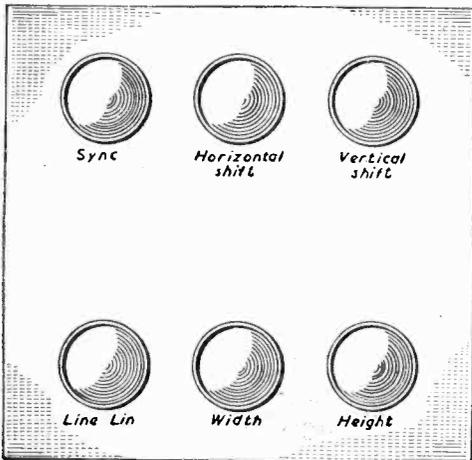
Fig. 5.—Main control panel layout.
