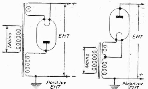
Fig. 29.—Showing the differences between a positive (left) and negative (right) E.H.T. supply.
