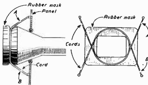
Fig. 3.—Method of mounting the mask.
