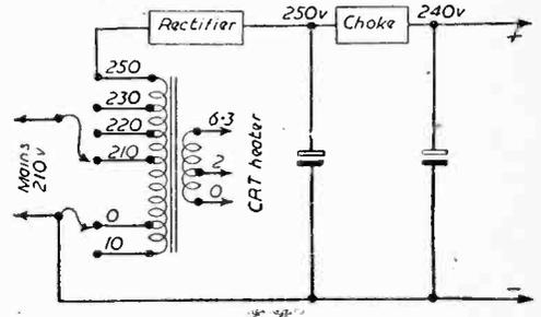
Fig. 27.—The auto-wound transformer arrangement.
