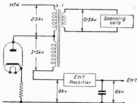
Fig. 30.—This is the flyback E.H.T. arrangement.
