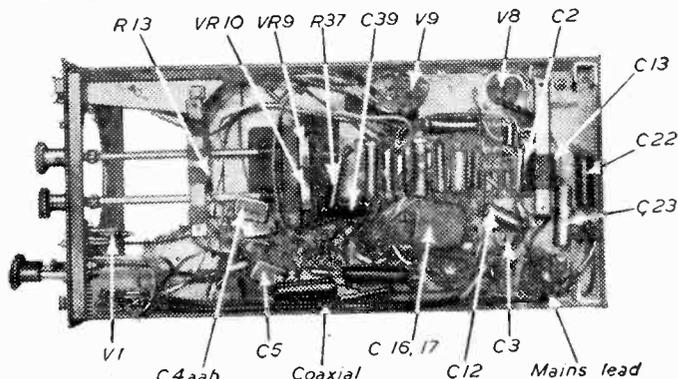
View of the completed unit. Positions of main components.
