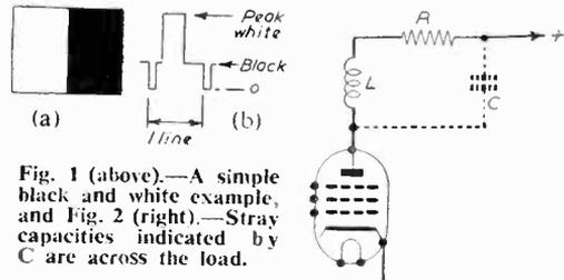
Fig. 1 (above).—A simple black and white example, and Fig. 2 (right).—Stray capacities indicated by C are across the load.
