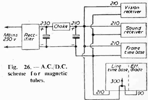
Fig. 26.—A.C./D.C. scheme for magnetic tubes.
