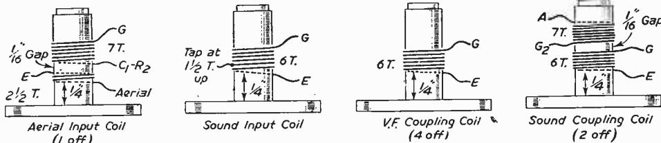
Fig. 7.—Details of the coils and the video corrector choke. The wire used for the coils is No. 28 D.C.C.
