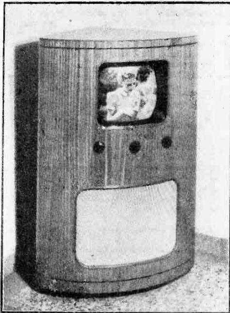
The Ambassador TV2 corner console model. It has a 12in. tube. (R. N. Fitton, Ltd.)
