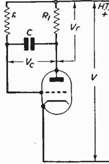
Fig. 10.—Miller integrator section of the time-base circuit.
