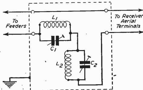
Fig. 1.—Circuit of the Wavetraps.
