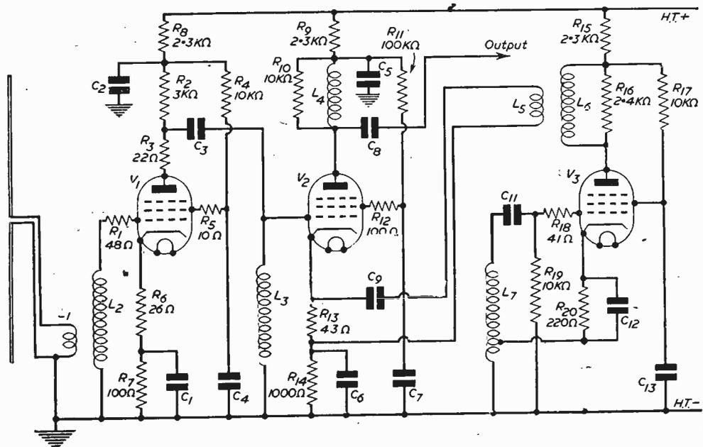
Fig. 1.—Original circuit of the RF24 Unit.
