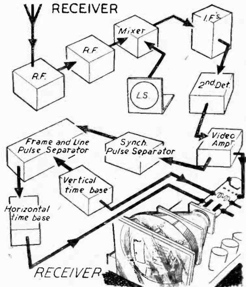
Figs. 24 and 25.—(Left) Block diagram of transmitting system showing chain of events from scanning to transmission. (Right) Block diagram showing chain of events from reception of sound and video signals by the receiver aerial, through the receiver to the tube.
