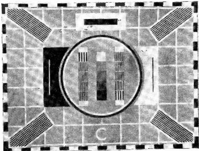
Test Card C, which will reveal practically any defect in a television receiver. The finest of the ruled squares will only be resolved when the acceptance of the receiver covers a bandwidth of 3 mc/s.
