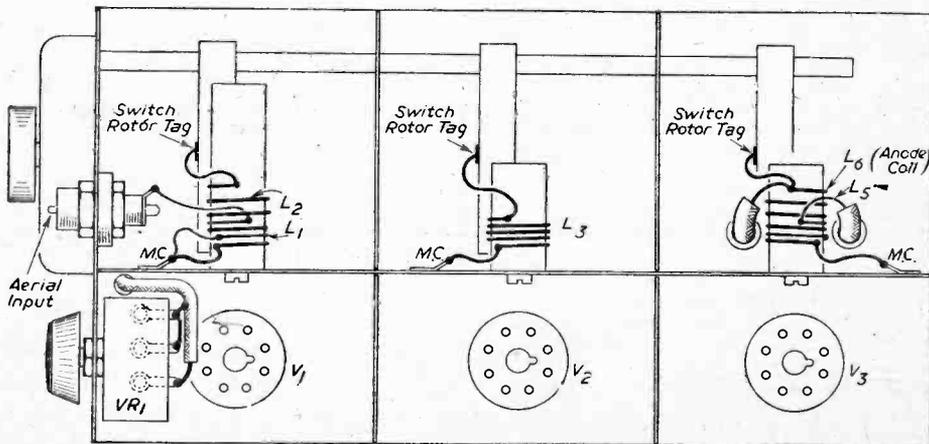
Fig. 4.—Top view, showing coil connections. The trimmers and fixed condenser have been omitted for clarity.
